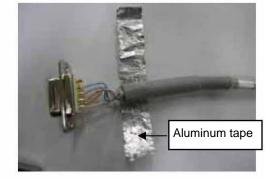
[3] Wrap an insulation table around the cable and then affix the cable with the cable holder. At this time, make sure the shielded wire does not project from the cable holder. (Cut the shielded wire, if necessary.)
