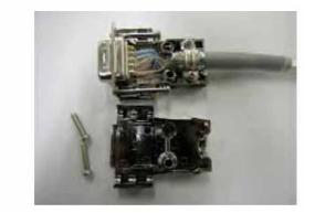
[2] Take out the cable holder and then remove the aluminum foil tape.
