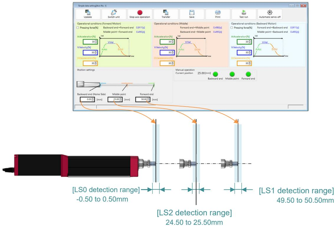
To adjust the LS signal detection range, open the "Parameters window".
