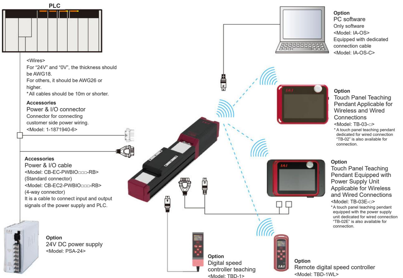
Supply 24V DC to the ELECYLINDER and input a signal from a master device to the ELECYLINDER.
