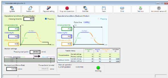
Simple data setting window in 3-Point Positioning Setting
