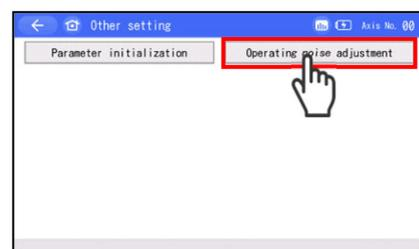
4. Touch  and  on the right and left of the levels (from 0 to 14) to adjust the level one by one to perform tuning. Once the tuning is finished, touch .
