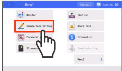
If the operating mode is not Monitor mode, the Message screen will be displayed. Switch to Monitor mode by following the displayed instructions.
