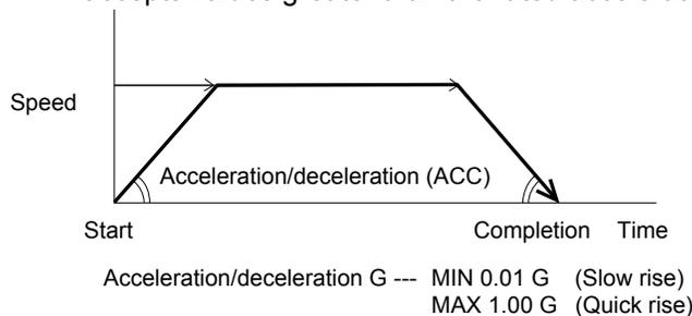
**Note:** Enter appropriate values for speed and acceleration/deceleration by referring to 1.3, “Specifications” and considering the installation conditions and shape of the load, to make sure the actuator will not receive excessive impact or vibration.
