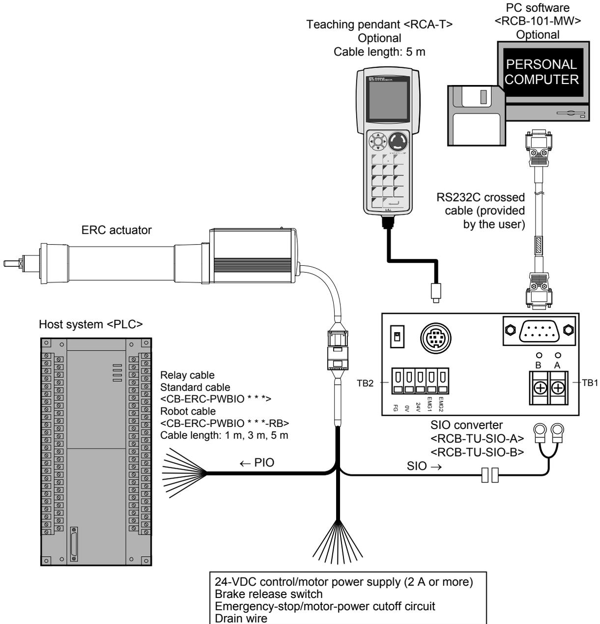
**Note:** Do not connect a teaching pendant and a PC at the same time. If both are connected at the same time, a communication error (message level) will occur.
