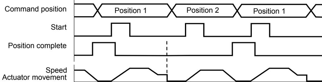
If the actuator has missed the load, the position complete output will not turn ON.
