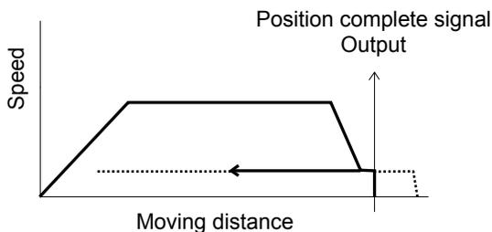
If the actuator is pushed back after the position complete output has turned ON because the actuator thrust is smaller than the reactive force of the load, the actuator will be pushed back all the way until its thrust balances out with the reactive force of the load. The position complete output will remain ON.
