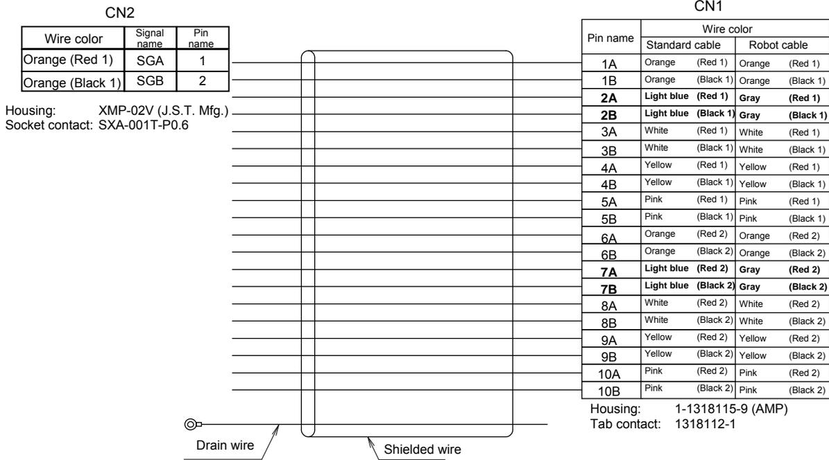
(Supplied cables to be connected to CN2)
