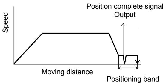
If the load moves in the pushed direction after the position complete output has turned ON, the actuator will push the load within the positioning band. If the current drops below the limiting value, the position complete signal will turn OFF. The signal will turn ON when the current rises to or above the limiting value.
