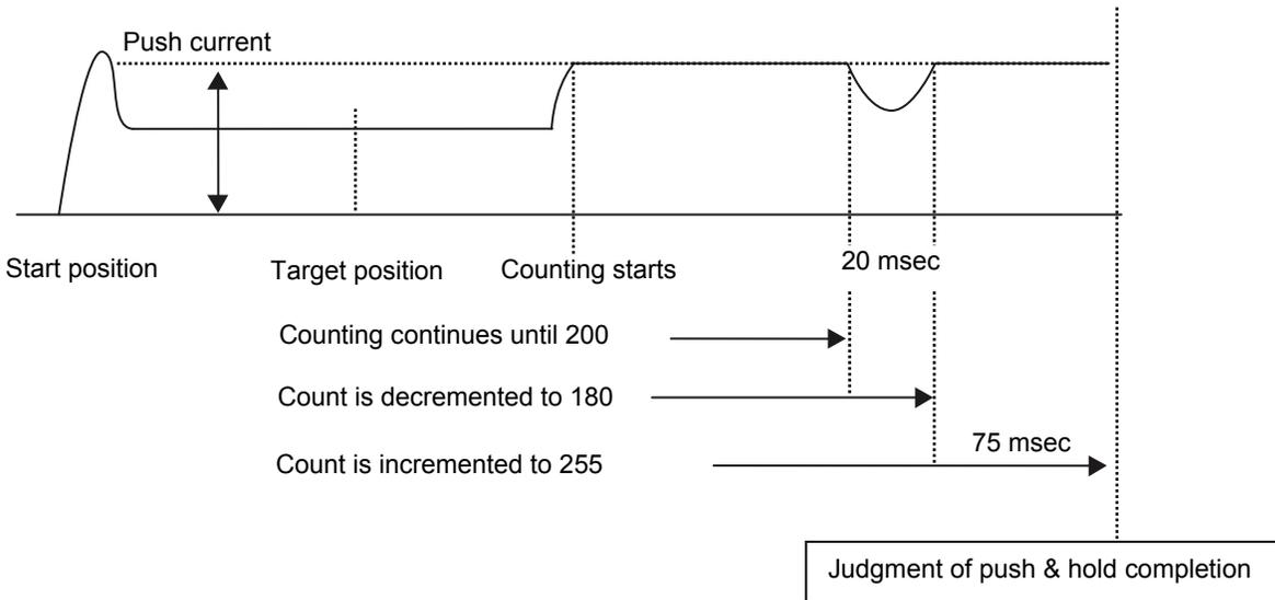
After reaching the push current, it is maintained for 200 msec. The current drops during the subsequent 20-msec period, and accordingly the count is decremented by 20. Therefore, when the operation is resumed the count will start from 180. Since the count will reach 255 after 75 msec at the push current, the controller will determine that the push & hold operation has completed.
