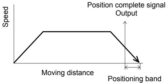
(1) The position complete output will turn ON at a position preceding the target position by the positioning band.
