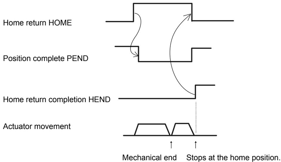
Note: When the home return signal turns ON, the position complete output will turn OFF.
