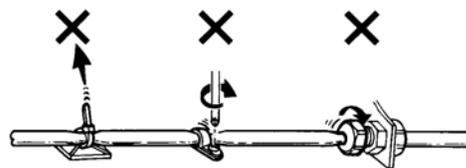
6. Do not pinch, drop a heavy object onto or cut the cable.
