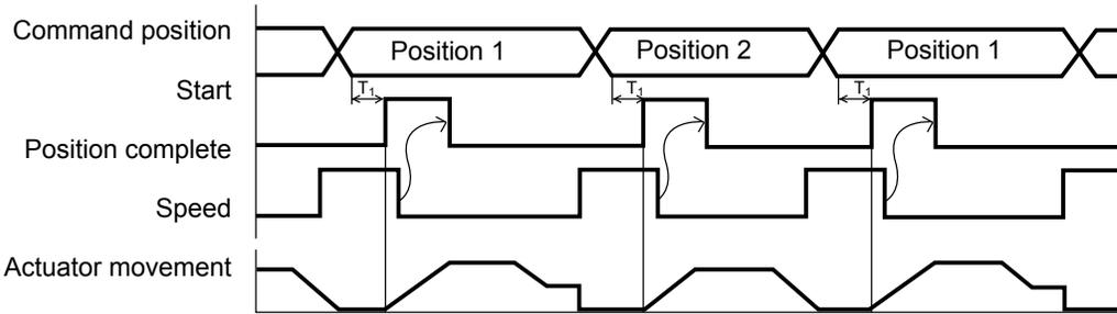
T1: 6 msec or more; time after selecting/entering a command position until the start input turns ON (The scan time of the host controller must be considered.)
