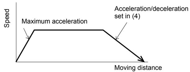
Note: A rough guide for enabling the acceleration only MAX function is when the actual payload capacity is one-third the load rating or less.
