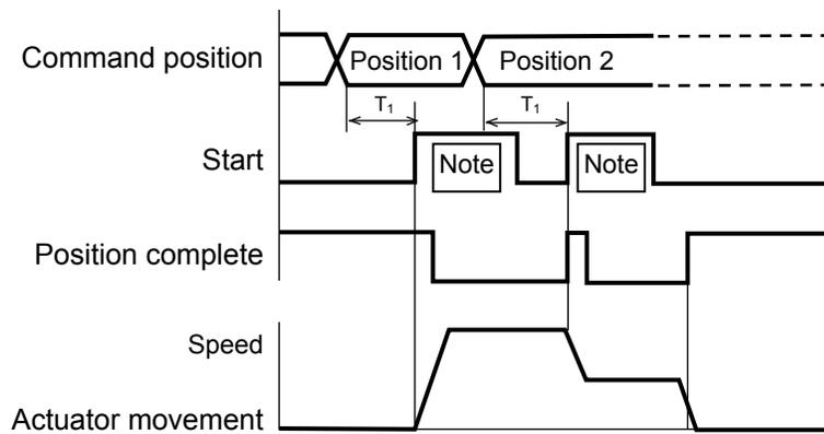
T1: 6 msec or more; time after selecting/entering a command position until the start input turns ON
