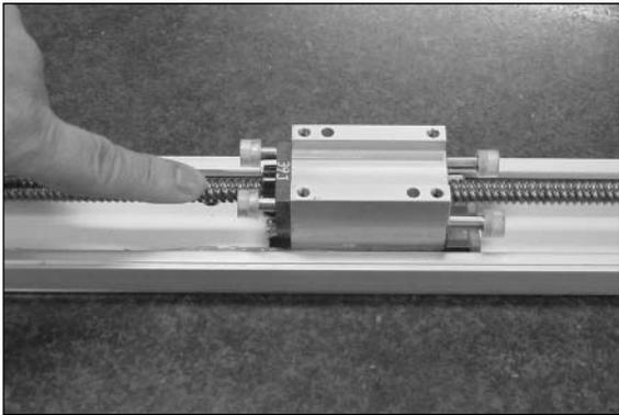
After cleaning the ball screw, apply grease and stroke the slider to let the grease spread evenly. As the final step, wipe off excess grease from the ball screw. This is because excessive grease will cause the agitation resistance to increase and allow the ball screw to generate heat easily. Wiping off excess grease will also prevent extra grease on the ball screw from flying off and staining the surrounding area as the screw turns.
