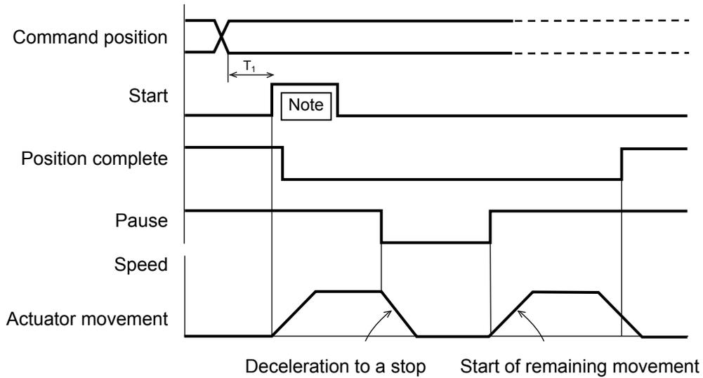
T1: 6 msec or more; time after selecting/entering a command position until the start input turns ON (The scan time of the host controller must be considered.)
