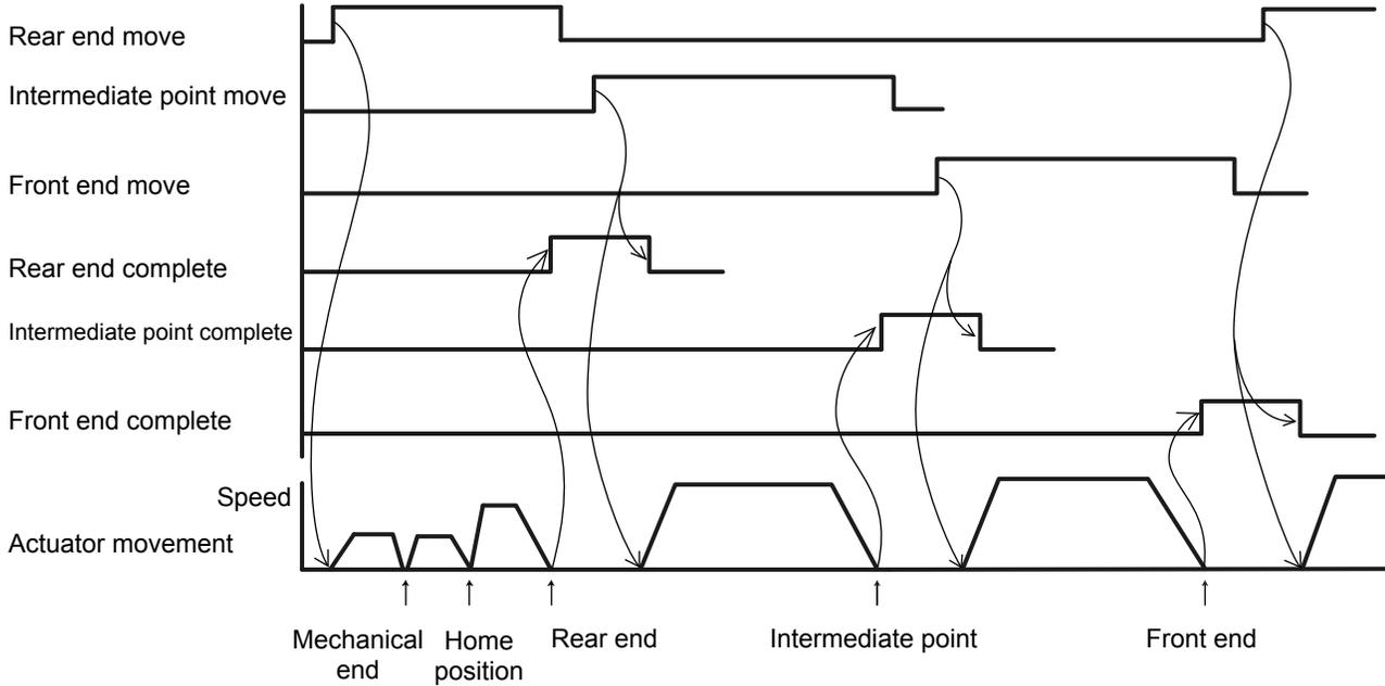
Note: Movement commands are executed based on the rise edge, so input each signal continuously for 6 msec or more.
