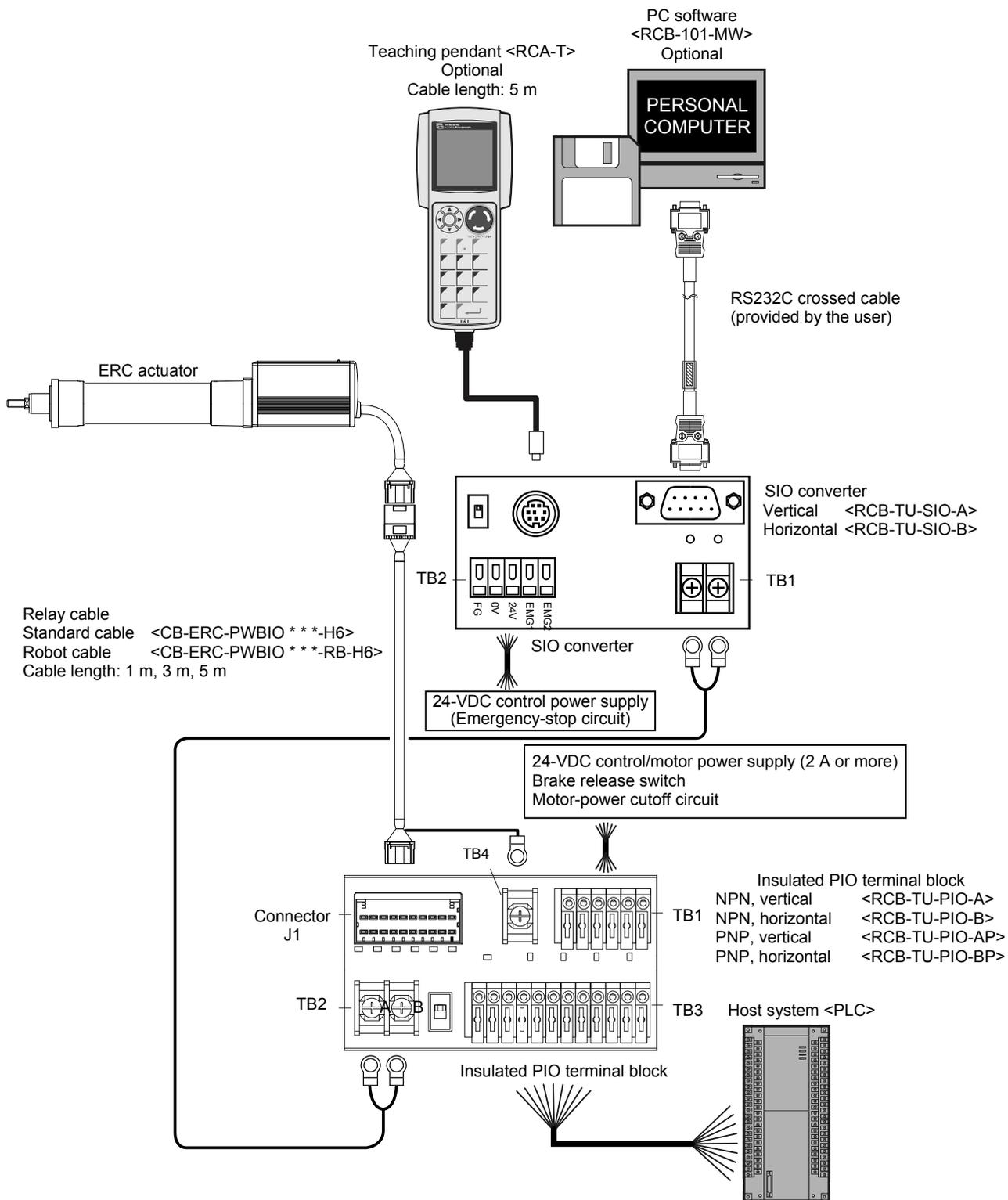
**Note:** Do not connect a teaching pendant and a PC at the same time. If both are connected at the same time, a communication error (message level) will occur.
