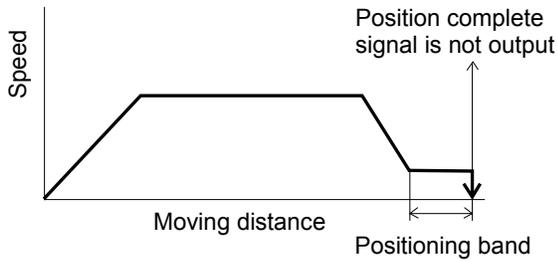
(1) After reaching the target position, the actuator will move at low speed. Even after contacting the load, the actuator will move to the end of the positioning band if the stepper motor current is yet to reach the current-limiting value. The position complete output will not turn ON even when the end of the positioning band is reached. (Provide a timeout check process after a sufficient period with a PLC.)
