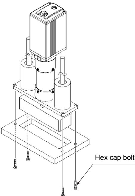
**⚠ Caution:** If the actuator is installed horizontally, exercise caution not to let the actuator receive excessive forces.
