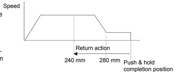
Note: When the start signal turns ON, the position complete output will turn OFF. The start signal must be turned OFF with the confirmation that the position complete output has turned OFF while the start signal remains ON. If the actuator has missed the load, the position complete output will not turn ON as shown below.
