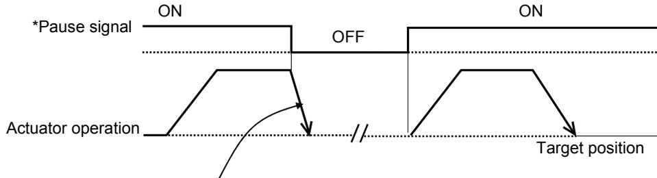
(Note) During deceleration, the acceleration/deceleration set in the position table under the currently executed position number is used.
