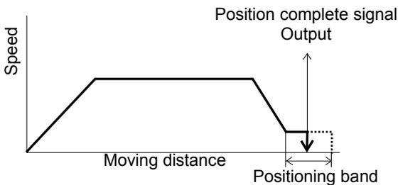
(1) After reaching the target position, the actuator will move at low speed (75 rpms). When the Pos. band set in the data table (see Note) is reached after the actuator contacts the load and the stepper motor current has reached the current-limiting value, the position complete output will turn ON.
