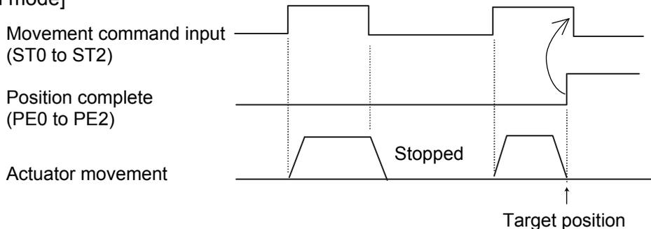
(Note) Turn OFF the movement command input after confirming that the target position has been reached.
