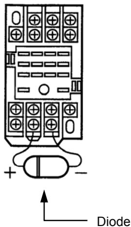
In a DC circuit, connecting a diode in reverse polarity will damage the diode, internal parts of the controller and/or DC power supply, so exercise due caution.
