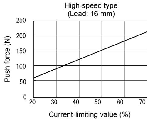
Note: The accuracy of push force at standstill is not guaranteed. The above graphs are provided for reference purposes only. If the push force is too small, malfunction may occur during push & hold operation due to slide resistance, etc., so exercise caution.
