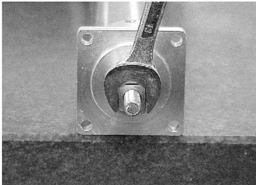
Note) Apply a spanner at the rod end bracket to prevent the rod from receiving any rotating moment when the load is installed.
