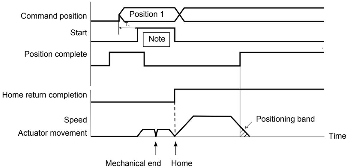
The position complete output will turn ON when the controller becomes ready following the power ON. To check if the controller is ready, always check if the position complete output is ON. The actuator will not operate unless the pause input is turned ON.
