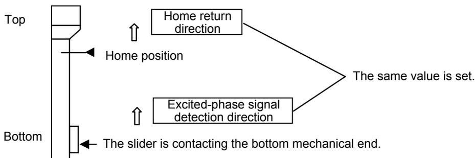
(Example 2) The power is turned on when the slider, installed vertically with the motor at the bottom, is contacting the bottom mechanical end.
