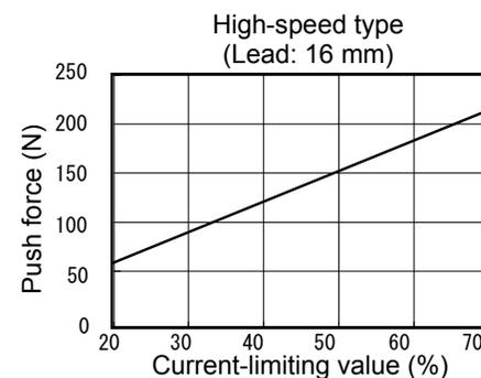
Note: The accuracy of push force at standstill is not guaranteed. The above graphs are provided for reference purposes only. If the push force is too small, malfunction may occur during push & hold operation due to slide resistance, etc., so exercise caution. The maximum current-limiting value is shown in the above graphs. The minimum value is 20%.
