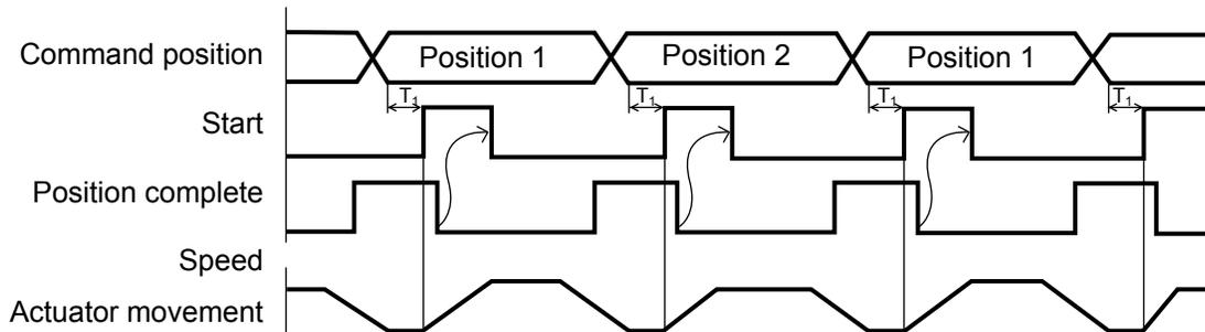
T1: 6 msec or more; time after selecting/entering a command position until the start input turns ON
