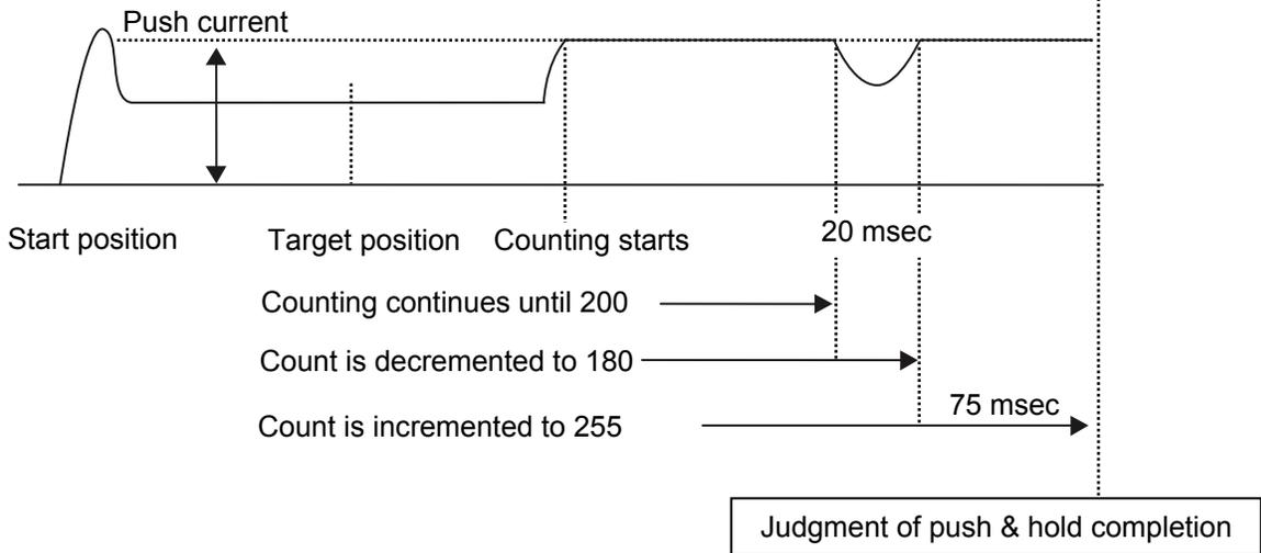
After reaching the push current, it is maintained for 200 msec. The current drops during the subsequent 20-msec period, and accordingly the count is decremented by 20. Therefore, when the operation is resumed the count will start from 180. Since the count will reach 255 after 75 msec at the push current, the controller will determine that the push & hold operation has completed.
