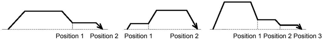
The speed change operation explained above is useful when, among others, the load is made of soft material or is a bottle or other shape that easily topples and you don't want to give vibration or shock to the work part when the actuator stops.
