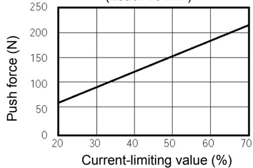
⚠ Caution: The precision of push force at standstill is not guaranteed. The above graphs are provided for reference purposes only. If the push force is too small, malfunction may occur during push & hold operation due to slide resistance, etc., so exercise caution. The maximum current-limiting value is shown in the above graphs. The minimum value is 20%.
