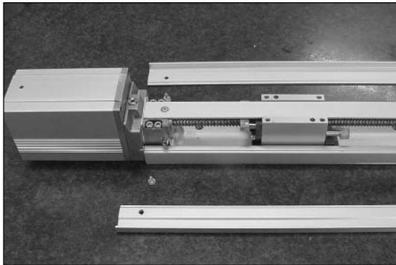
[1] With the SA6 and SA7, the screw cover and side covers can be removed using a hex wrench with 1.5 mm width across flats.
