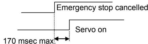
**⚠ Warning:** Since a pulse motor is used as the driving motor, the excited phase will be detected when the servo is turned on for the first time after the power on.
