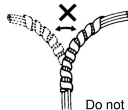
Do not use a spiral tube where the cable flexes frequently.
