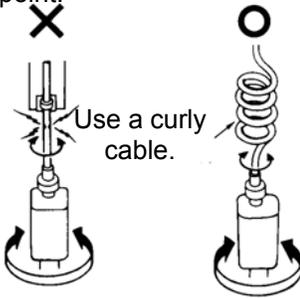
5. When fixing the cable, provide a moderate slack and do not tension it too tight.
