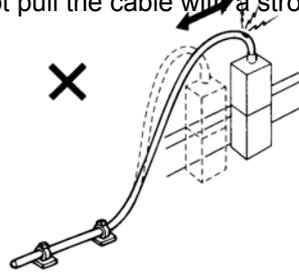
4. Do not let the cable receive a turning force at a single point.
