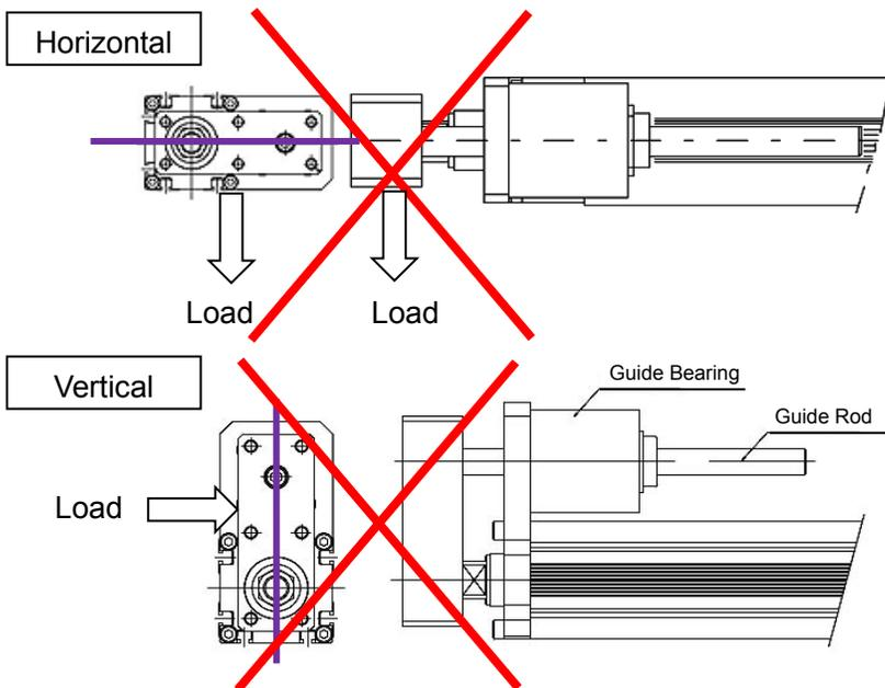
Do not attempt to use the unit in an environment that load torque or load moment can be applied as shown in the figures below.
