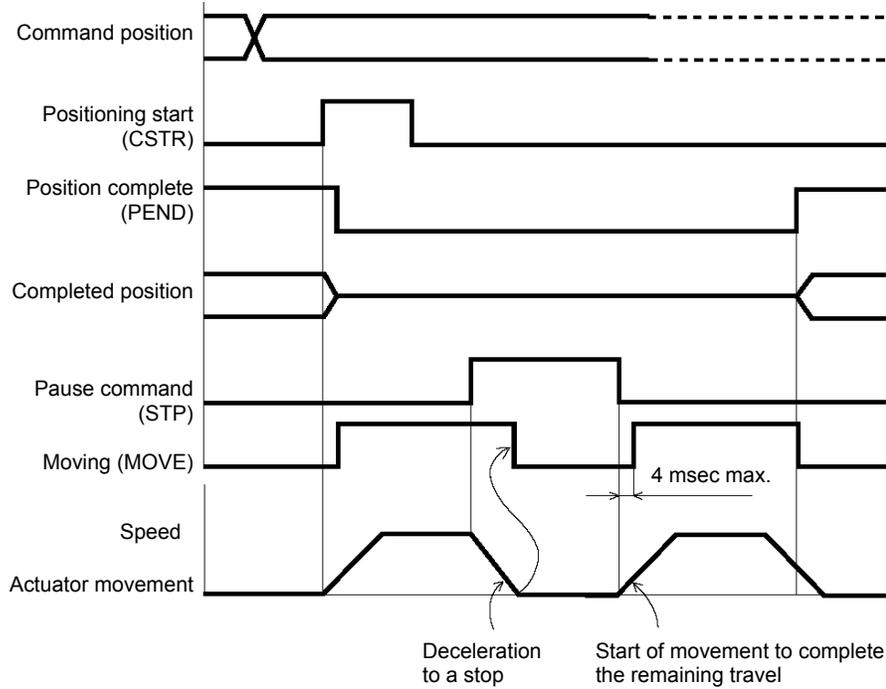
Changing the alarm reset (RES) bit to "1" while the actuator is paused will cancel the remaining travel. When a cancellation of the pause command (STP) is recognized thereafter, the position complete signal (PEND) will turn "1" in approx. 1 msec. (The remaining travel will be cancelled upon detection of the leading edge of the reset signal.)
