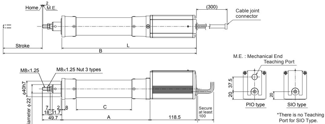
Appearance Figure for Brake-equipped Type
