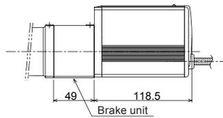
(note) The angle of the 2 faces on the actual product would not be as shown in the drawing.
