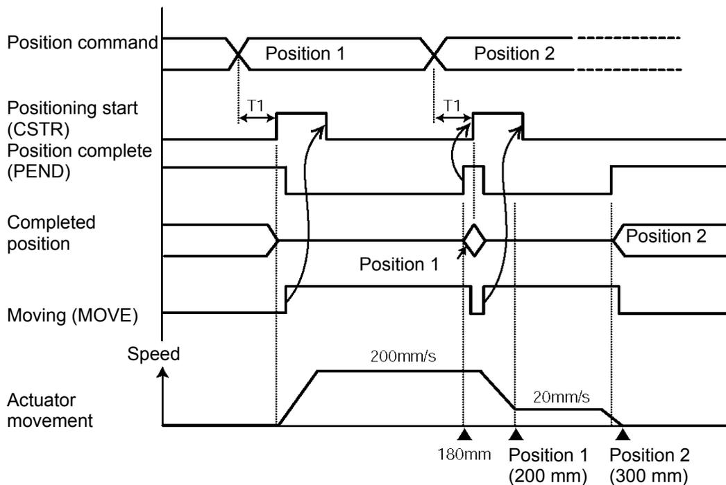
\*T1: Set to  $T1 \geq 0$  (ms) by considering the scan time of the host controller.
