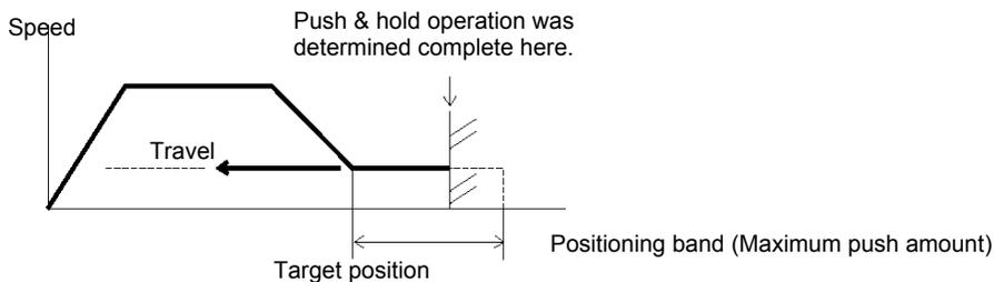
(Note) If the actuator is pushed back to the target position, an alarm will generate.
