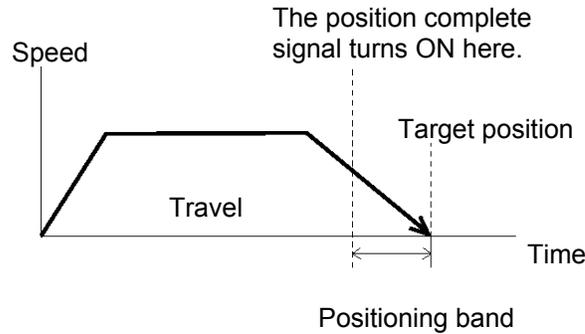
When the servo turns on after the power on, the current position will become the target position. As a result, this signal bit will turn "1." It will turn "0" if positioning operation is started thereafter with the CSTR signal bit changing to "1."
