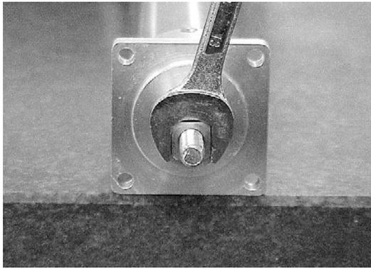
Note) Apply a spanner wrench at the rod end bracket to prevent the rod from receiving any rotating moment when the load is installed. Applying excessive rotating moment to the rod may damage the rod.
