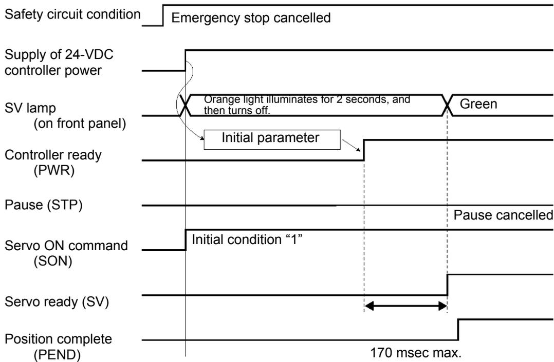
**⚠ Caution:** When the power is turned on while an emergency stop is actuated, and then the emergency stop is cancelled, the servo will turn on with a maximum delay of 170 msec after the cancellation of emergency stop.
