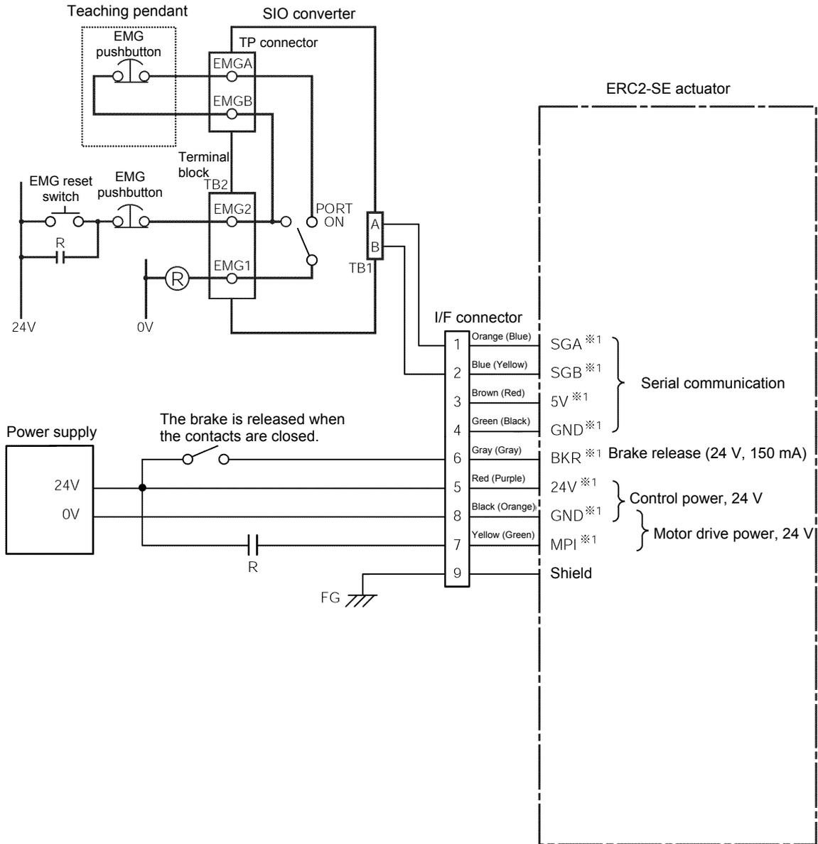
\*1 The wire colors for standard cables and robot cables are different. The colors in parentheses are for robot cables.
