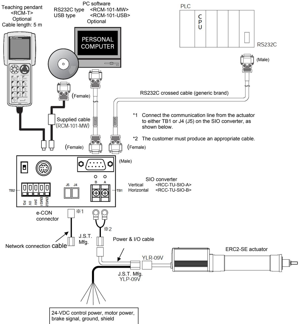
**⚠ Caution:** Do not connect any device to the mini-DIN connector and D-sub connector at the same time. If a device is connected to these connectors at the same time, a communication error (message level) will occur.
