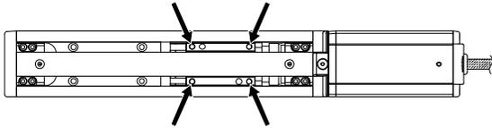
Four tapped holes are provided in the slider, so affix the load using these holes (indicated by arrows in the figure shown to the left).
