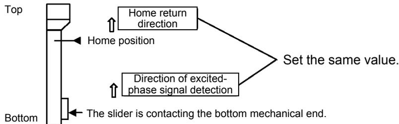
(Example 2) Power was turned on when the slider was contacting the bottom mechanical end in a configuration where the actuator is installed vertically with the motor at the bottom.
