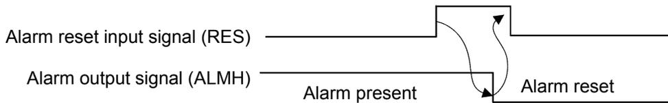
**⚠ Caution:** Before resetting an alarm, always identify and remove the cause of the alarm. If the cause cannot be removed or the alarm still persists after removing the cause, contact IAI. If the same error occurs again after resetting the alarm, the problem that caused the alarm in the first place is still present.
