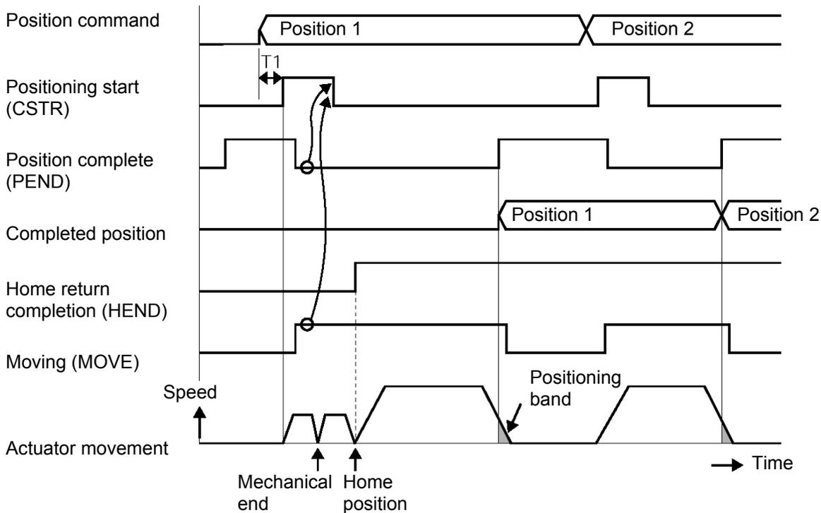
\*T1: Set to  $T1 \geq 0$  (ms) by considering the scan time of the host controller.
