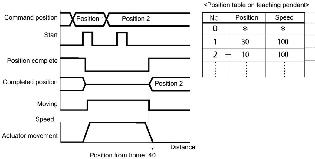
If a start signal is input multiple times for a position number by incremental specification while the actuator is performing positioning operation, the actuator will move to the position representing the initial position plus the "incremental travel x number of times the signal was input."
