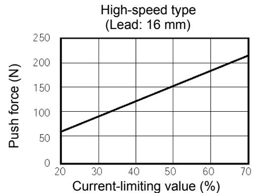
⚠ Caution: The precision of push force at standstill is not guaranteed. The above graphs are provided for reference purposes only. If the push force is too small, malfunction may occur during push & hold operation due to slide resistance, etc., so exercise caution.
