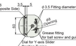
Detailed view of V2 Y-axis Slider Grease Supply Inlet Y-axis Slider End Side
