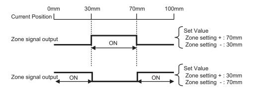
Caution : The signal cannot be output unless the range of the zone detection is set to a value greater than that of the minimum resolution (actuator lead length/800).
