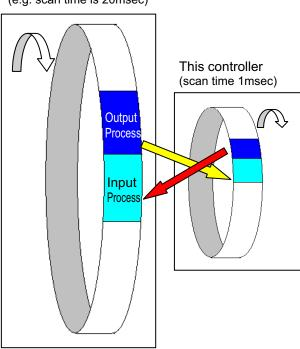
As shown in the diagram, the input and output timings of two devices that have different scan time do not match, of course, when transferring a signal.
