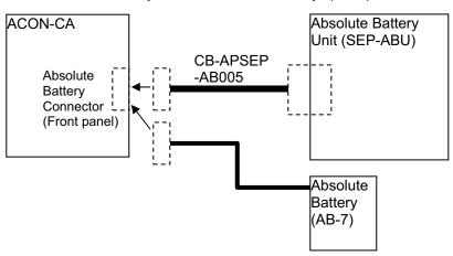
2) For Serial Absolute Type (ACON-CA Only) Connect to the "Absolute battery" (AB-5).
