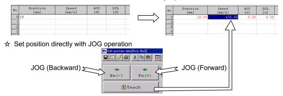
• Procedure 6 : Transfer the information such as Position that is written in Position Table to the controller.
