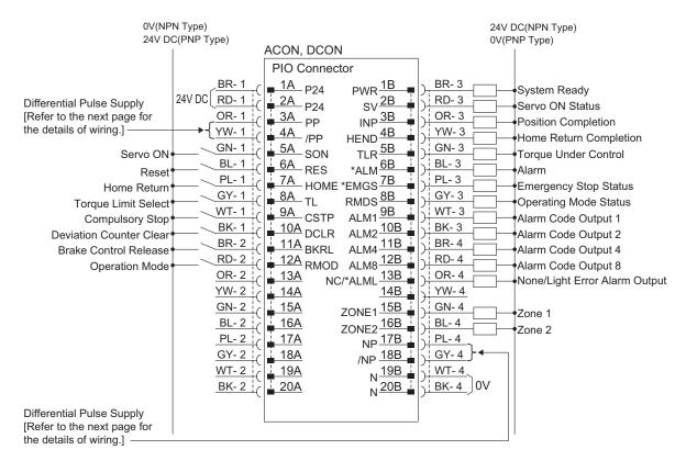
"\*" in codes above shows the signal of the active low. Processing occurs when an input signal of the type is turned OFF. An output signal of the type is normally ON in the power-on status and turned OFF at signal output.
