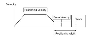
Caution : If the velocity of the positioning of the position table is set below this parameter, the pressing speed will become the same as the positioning speed.
