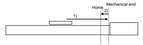
1) With the HOME signal being ON, the actuator moves toward the mechanical end at the home return speed.
