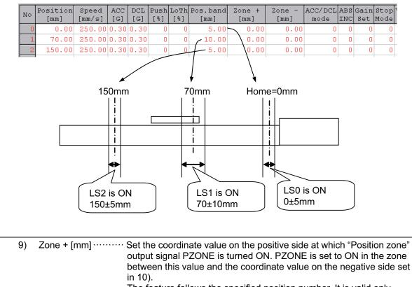
The feature follows the specified position number. It is valid only when the position is specified but invalid in another position operation.
