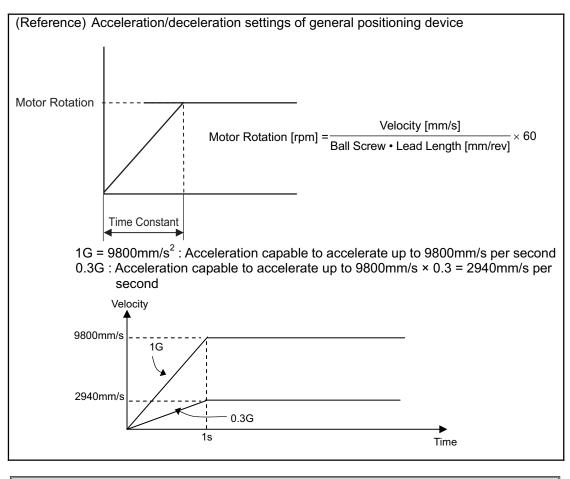
Caution : Set the acceleration/deceleration speed not to exceed the maximum acceleration/deceleration speed of the actuator. An operation with exceeding condition may cause a malfunction.
