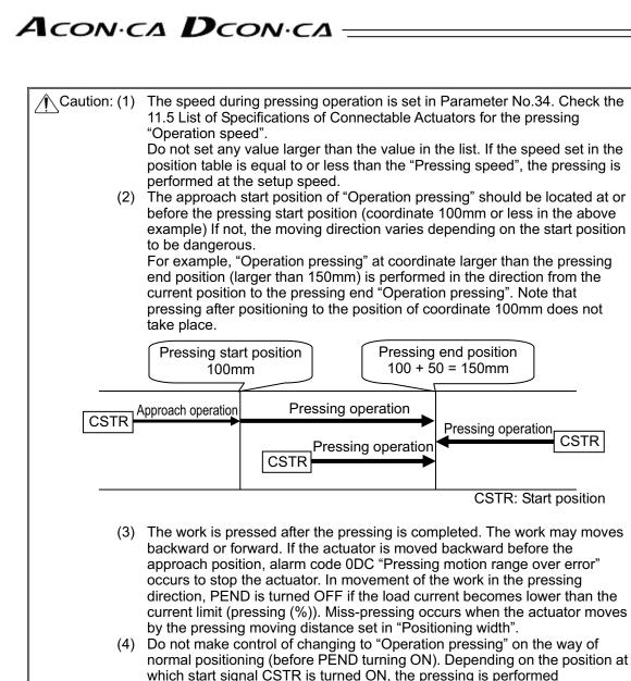
(5) If the actuator gets pressed to the work during the approach operation, 0DC "Pressing Operation Range Over Error" would be issued.
