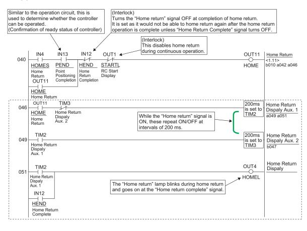
[6] Decode Circuit of Positioning Complete Position No.
