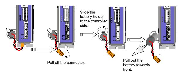
Follow the steps in the back order to detaching when attaching a new battery.
