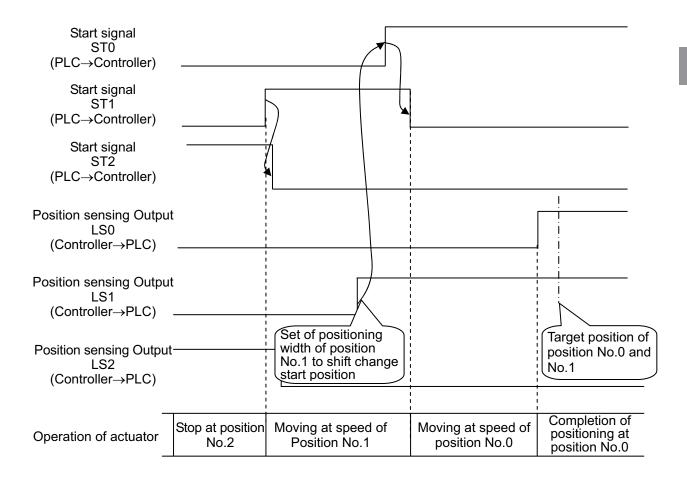
[5] Pause and Operation Interruption (ST\*, \*STP, RES, PE\*, PEND) Turning start signal ST\* OFF allows the actuator to be paused while it is moved. To restart it, turn the same ST\* signal ON.
