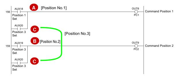
[13] Start Signal Output Circuit
