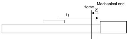
1) With the HOME signal being ON, the actuator moves toward the mechanical end at the home return speed.
