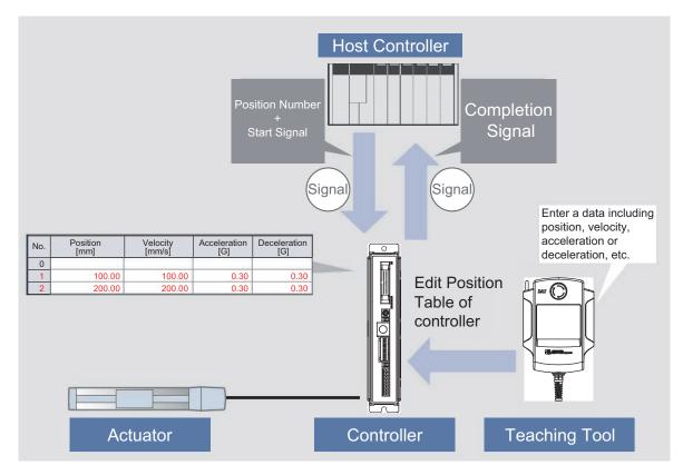
●Operation Ready • • Registration of Position Data (Example of Registration of PC software) • Procedure 1 : Turn ON the controller.
