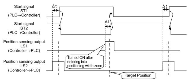
$\Delta t$ : Time required to certainly reach the target position after the position sensing output LS1 or 2 is turned ON.
