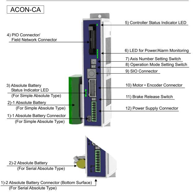
DCON-CA 5) Controller Status Indicator LED 4) PIO Connector/ Field Network Connector 6) LED for Power/Alarm Monitoring 7) Axis Number Setting Switch 8) Operation Mode Setting Switch 9) SIO Connector 3) Absolute Battery 10) Motor • Encoder Connector Status Indicator LED (Not to be used) 11) Brake Release Switch 2) Absolute Battery 12) Power Supply Connector (Cannot use) 1) Absolute Battery Connector (Not to be used)
