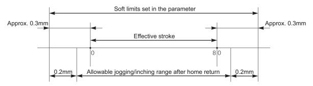
The operational range for jog and inching after the home return is 0.2mm [deg] less than the set value.
