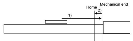
1) With the ST0 signal being ON, the actuator moves toward the mechanical end at the home return speed.
