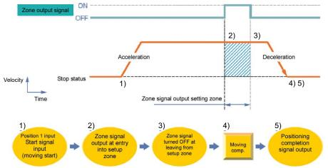
The relevant signal can be turned ON while the actuator passes or stops in the zone range in either of the following 2 types:
