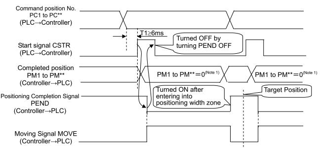
(Note 1) The "Completion position No." output is set to 0 during movement of the actuator.
