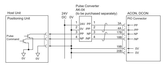
Caution : 1) Use the same power source for the host open collector input and output, AK-04.
