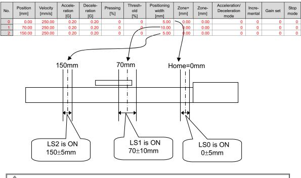
Caution : LS\* signal would not be output if the positioning width is set less than the minimum resolution.
