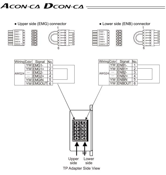
(3) Connection of dummy plug of TP adapter
