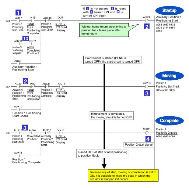
• Circuit 10 is designed to start positioning to position No.1 again after positioning to position No.3 is completed.
