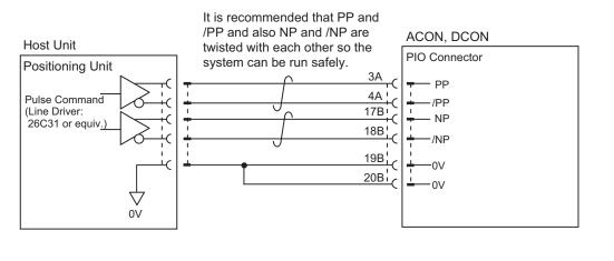
Caution : Make short-circuit between the host (positioning unit) and the 0V on PIO connector.
