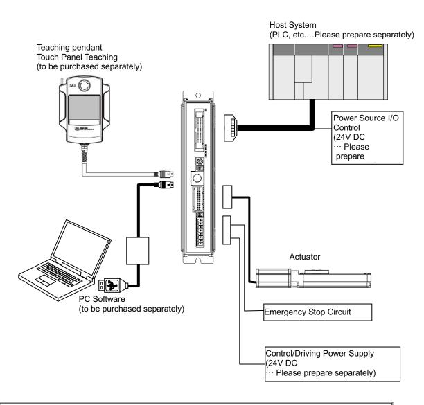
Caution : Make sure to turn the power to the controller OFF when inserting or removing the connector that connects the "PC software" or teaching pendant to the controller. Inserting or removing the connector while the power is turned ON causes a controller failure.
