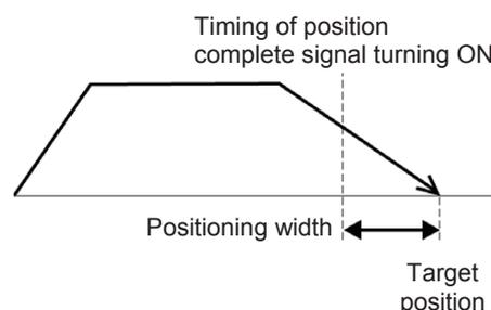
However, it defines the width of the position complete signal to turn ON for the 3-point type of PCON-C/CG/CF, PCON-CA, ACON-C/CG, ACON-CA, DCON-CA, SCON and ERC3 PIO Converter and the proximity switch type of PCON-CY and ACON-CY.
