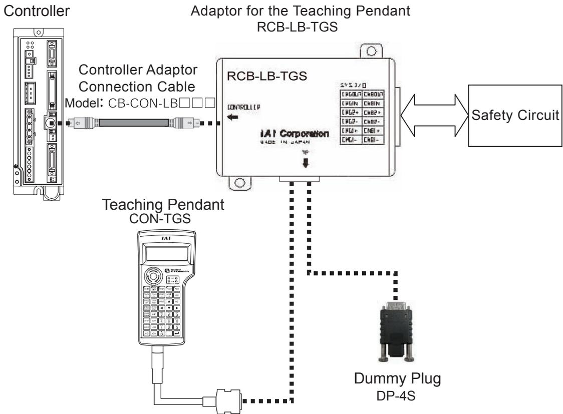
**Caution:** When the teaching pendant CON-TGS is not to be connected, make sure to insert the dummy plug DP-4S into the adaptor for the teaching pendant.
