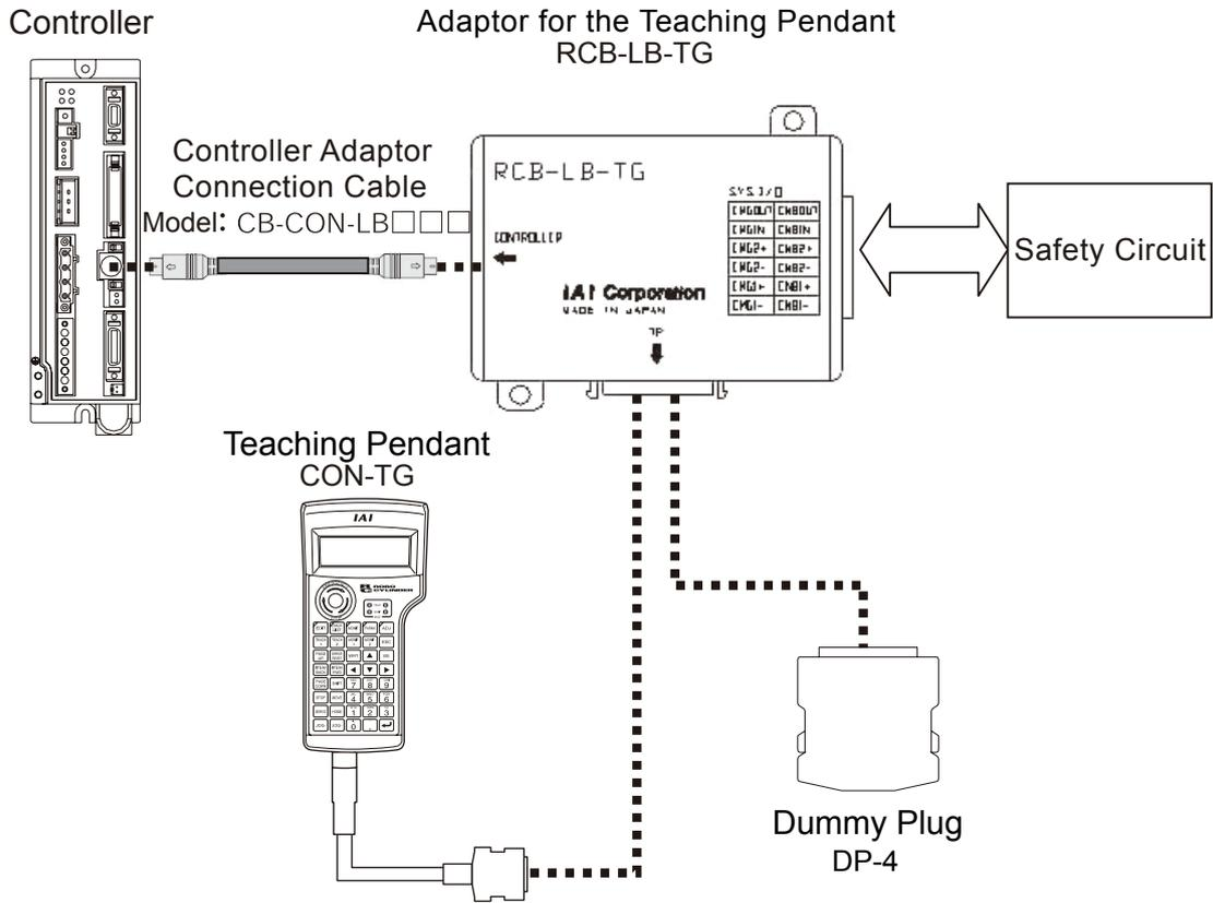
**Caution:** When the teaching pendant CON-TG is not to be connected, make sure to insert the dummy plug DP-4 into the adaptor for the teaching pendant.
