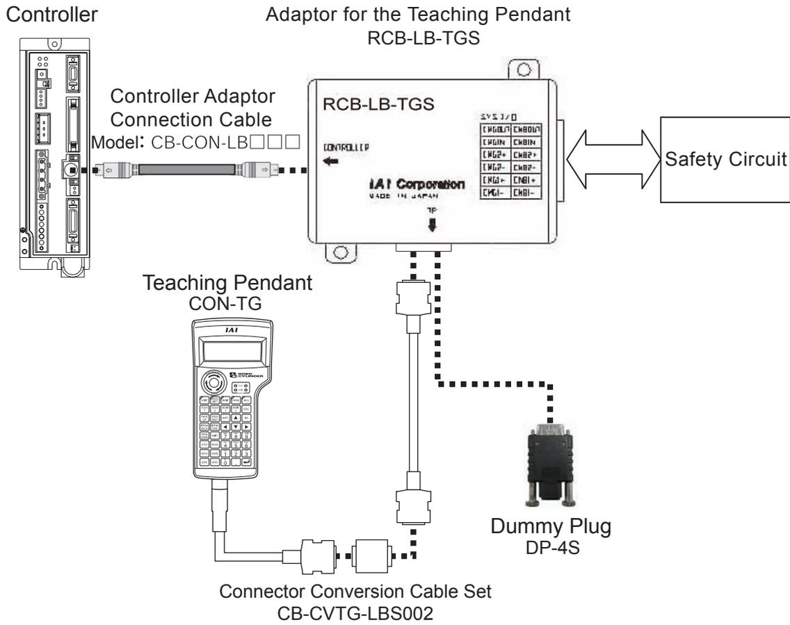
**Caution:** When the teaching pendant CON-TG is not to be connected, make sure to insert the dummy plug DP-4S into the adaptor for the teaching pendant.
