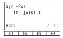
Press the WRT key to transfer the symbol data to the controller. The display returns to the previous edit screen.
