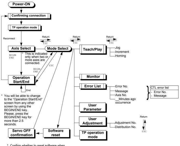
\* Confirm whether to reset software when going through the mode with the ESC key if changing the parameter.
