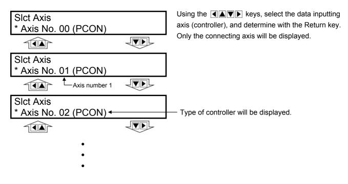
**Caution:** In the case of a controller with the PORT switch, when power is supplied with the PORT switch ON and power is present on the Easy type teaching pendant, only powered controllers will be detected.
