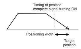
However, it defines the width of the position complete signal for the 3-point type of PCON-C/CG, ACON-C/CG, and SCON and the proximity switch type of PCON-CY and ACON-CY.
