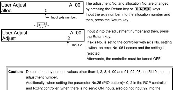
adjustment number. Since there is no servo ON input, operation cannot be made.
