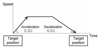
The acceleration will become sudden if the numeric value is made larger, and it will become gradual if the numeric value is made smaller.
