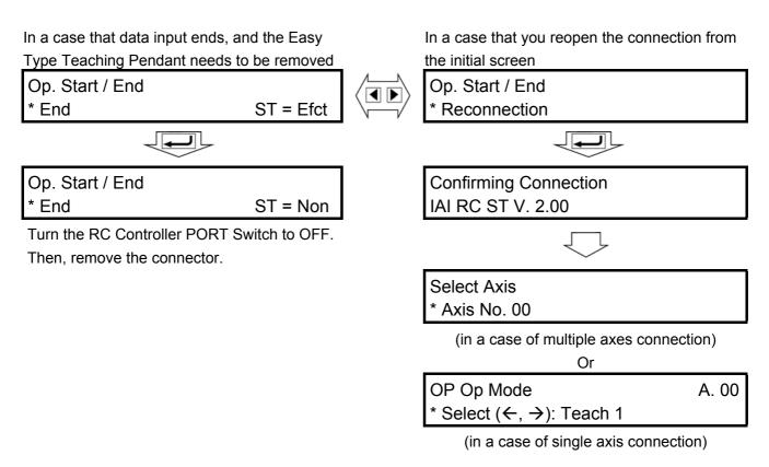
**Caution:** When multiple axes are connected with a controller link cable, after recycling power of a controller that is not directly connected to the Easy Type Teaching Pendant, please execute a reconnect.
