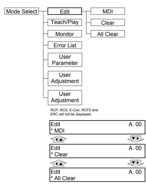
You can change the screens by using the arrow keys ( $\blacksquare$   $\bigcirc$ ) and press the return key.
