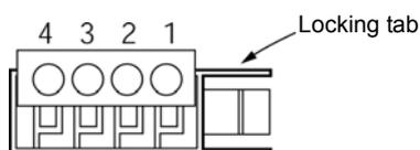
Be sure to insert the terminal resistor ( $220\Omega$ ,  $1/4W$ ) into the end of the communication main line. (between No. 1 and No. 2 of the e-CON connector)
