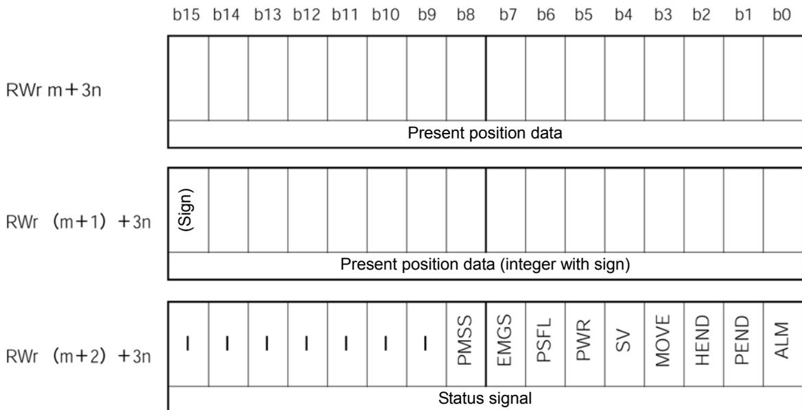
m is a head address assigned as simple direct value axis.
