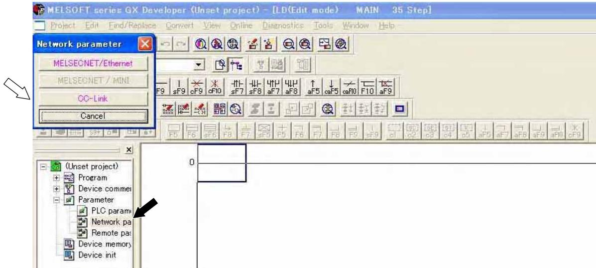
[2] Network parameter setting screen for CC-Link appears, then set the unit sheet number to one. (Master station is one sheet in this operational example.)
