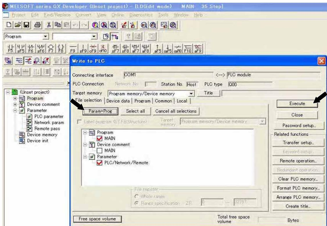
Click **Param+Prog** button on the PLC write screen, and select the “MAIN” for program and the “PC/Network” for parameter.
