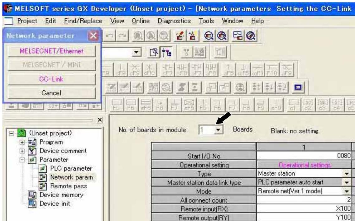
[3] Set parameters as shown below from now. Mode setting should be "Remote net [Ver. 1 mode]."
