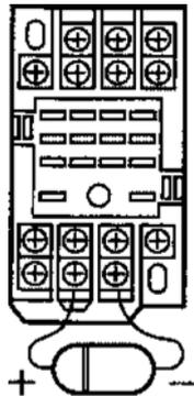
In a DC circuit, connecting a diode in reverse polarity will damage the diode, internal parts of the controller and/or DC power supply, so exercise sufficient caution.
