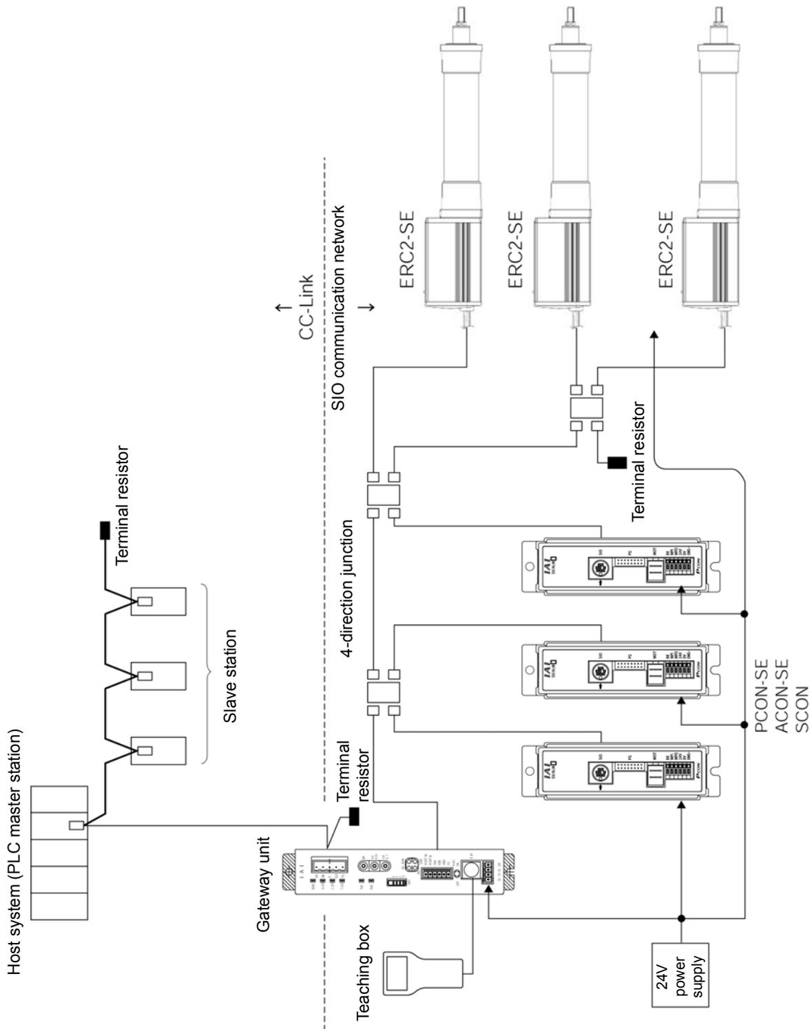
SIO communication connection is allowed even by multi-drop method using terminal blocks as follows.
