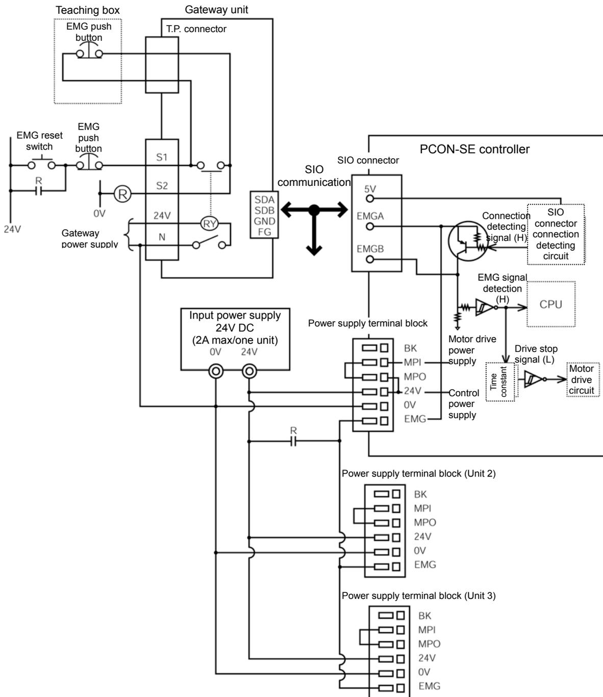
**⚠ Caution:** [1] The input current to the EMG terminal of PCON-SE is 5 mA. When connecting the contact of the EMG relay R to the EMG terminals of multiple controllers, check the current capacity of the relay contact.
