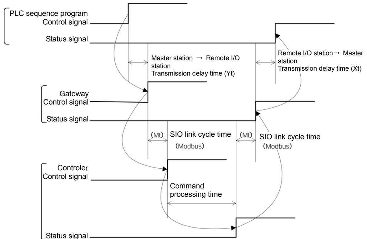
(Note) When communication error is caused due to a problem on the transmission path, communication retry (retry times = 3) occurs and a longer SIO link cycle time ( $M_t$ ) than normal may occur.
