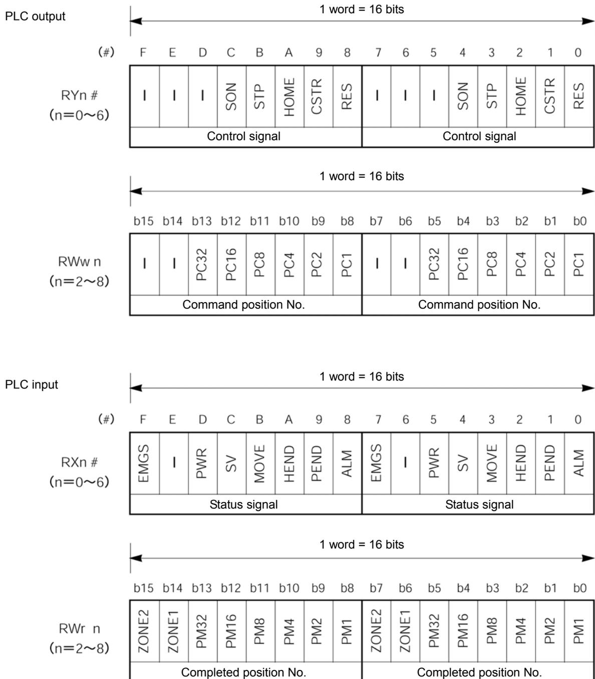
Details of input and output signal
