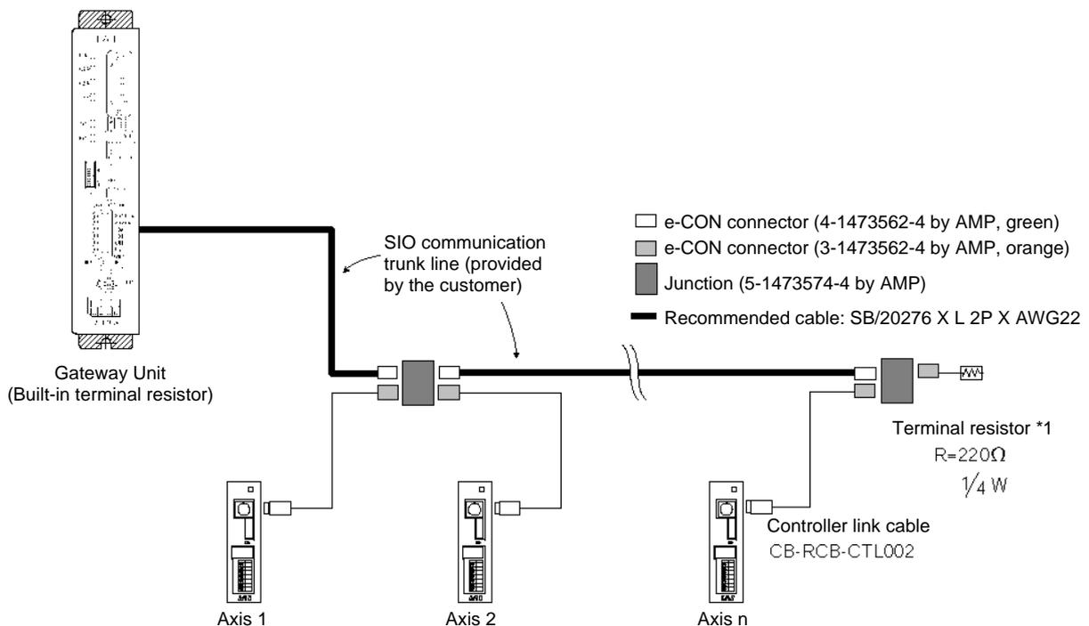
\*1 A terminal resistor (220 Ω, 1/4 W) is supplied with the controller link cable.
