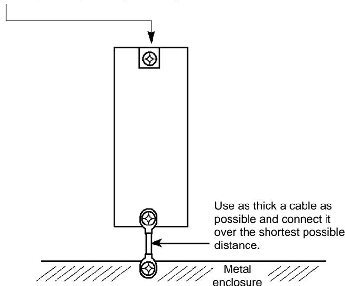
\* Provide class D (3) grounding for the enclosure.
