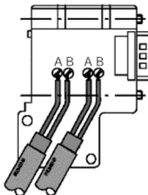
If the connector has a terminal resistor, turn the terminal resistor switch ON only for the terminal slave, and turn the switch OFF for all other slaves.
