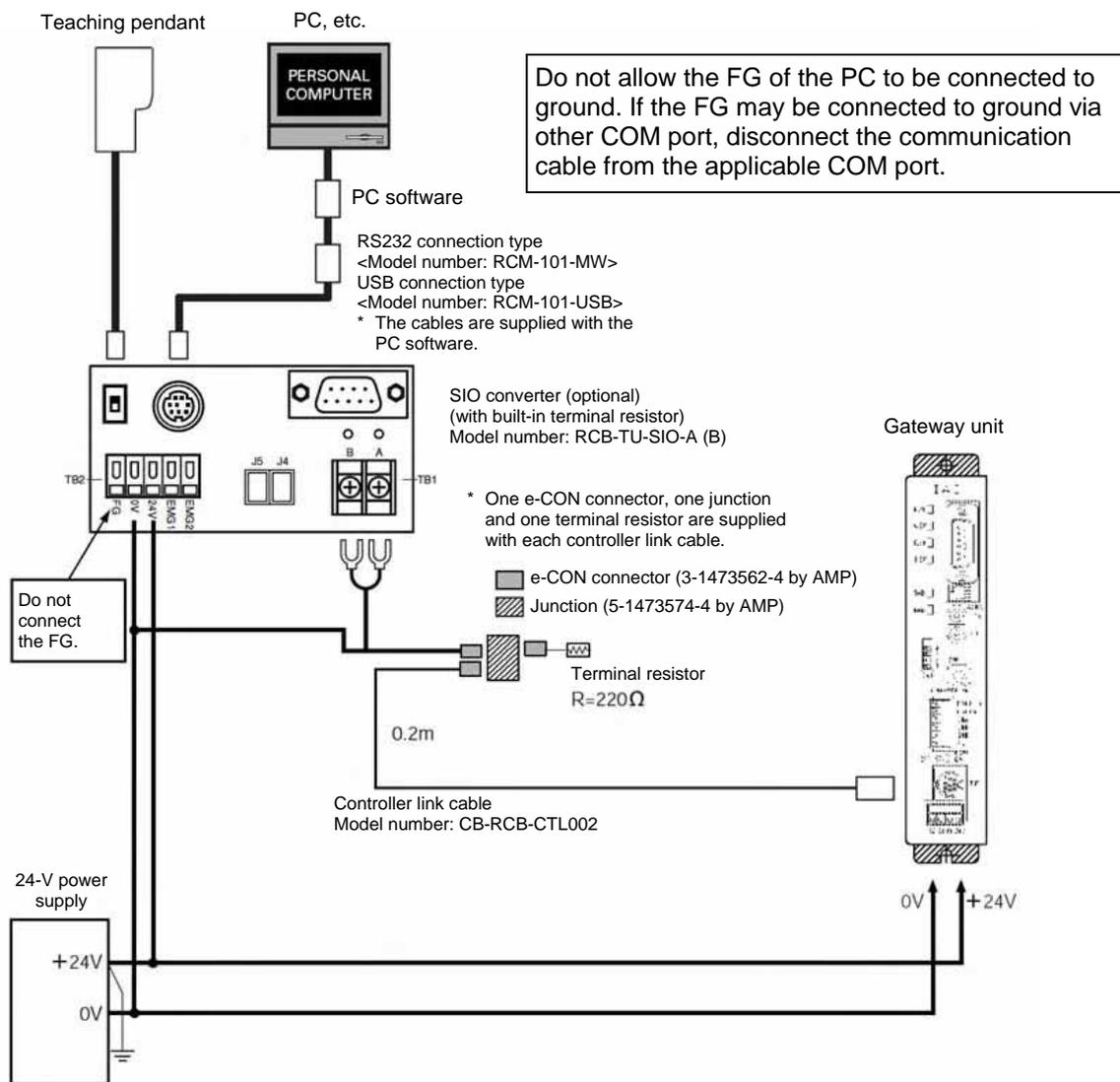
With the gateway unit system, the negative terminal of the 24-V power supply should be grounded (= 0 V should be grounded), as a rule. Since most teaching pendants and PCs have their communication ground line and FG (frame ground) shorted internally, grounding the positive terminal of the 24-V power supply (= grounding +24 V) will cause shorting of the 24-V power-supply circuit when a teaching pendant or PC is connected to the gateway unit, thereby damaging the teaching pendant or PC.
