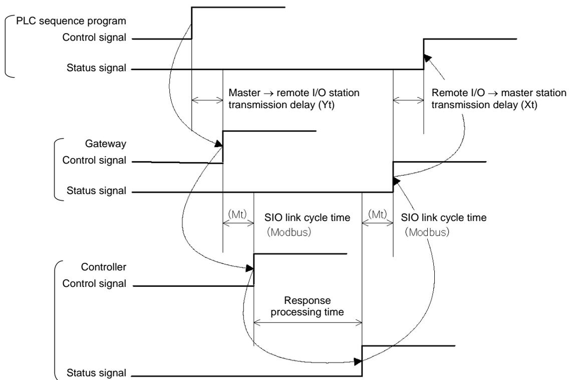
(Note) If a communication error occurs due to a problem along the transmission path, etc., a communication retry or retries (up to three times) may occur, in which case the SIO link cycle time (Mt) will be extended.
