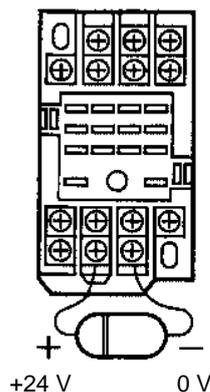
In a DC system, connecting the diode in reverse polarities may damage the diode, internal controller parts, and DC power supply. Exercise due caution.
