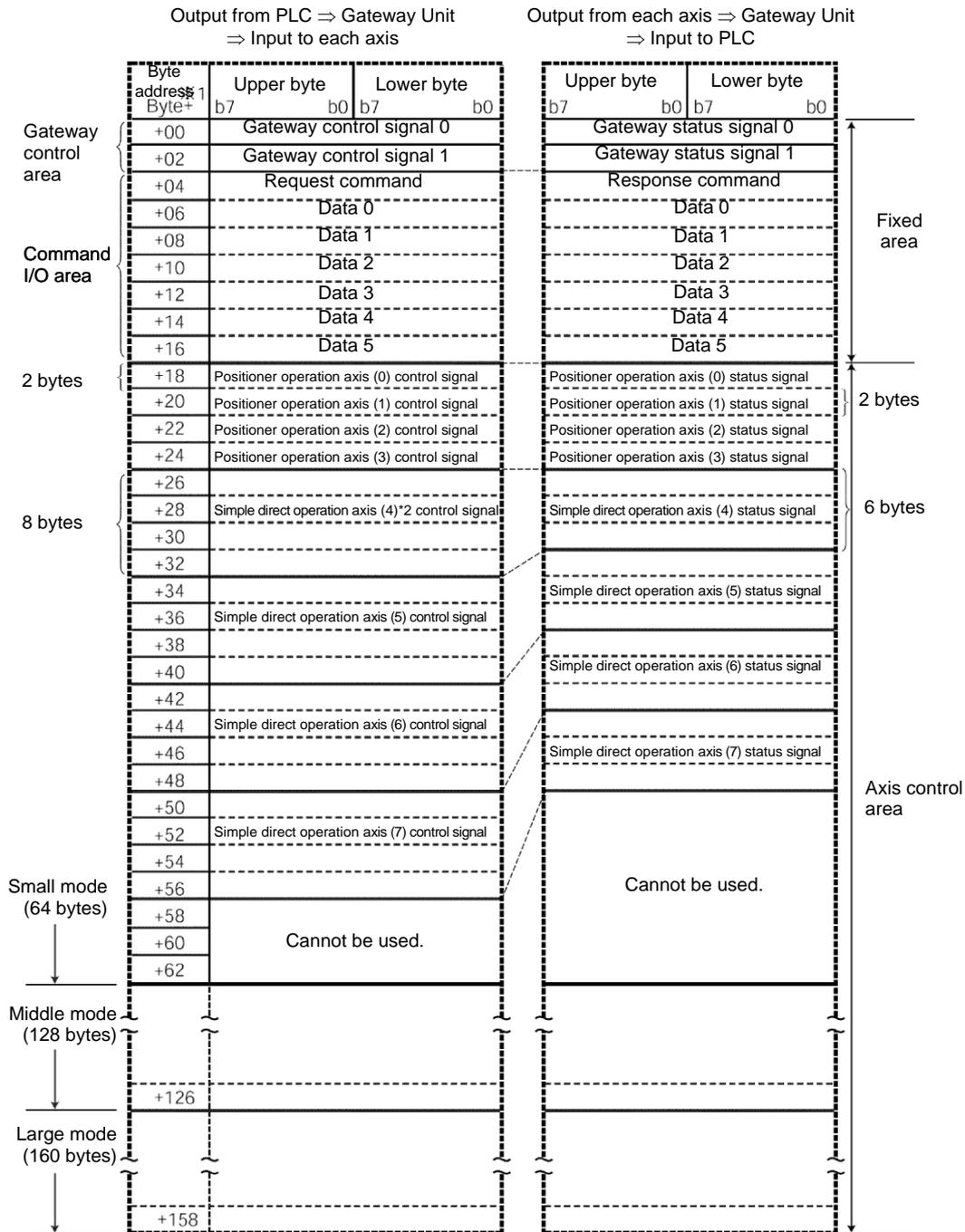
\*1 The byte address Byte+ indicates a relative address from the initial byte address of the gateway.
