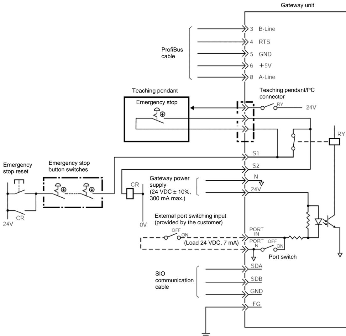
(3) I/O signal specifications and wires
