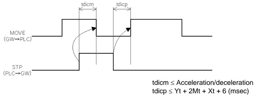
(6) Moving (MOVE) PLC input signal
