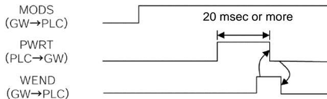
**(18) Forced brake release (BKRL) PLC output signal**
