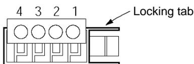
Always insert a terminal resistor (220 Ω, 1/4 W) at the end of the communication trunk (between pins 1 and 2 of the e-CON connector).
