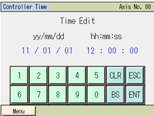
The numeric key pad appears. Enter a desired value, and then press [ENT].
