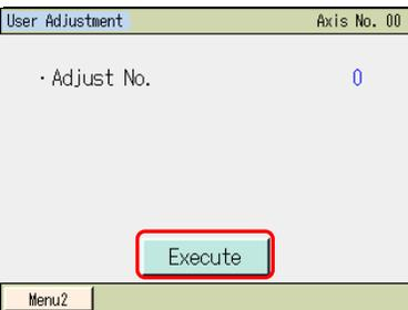
Touch [Adjust No.] and the numeric key pad opens. Set [Adjust No.] and touch [Execute.]
