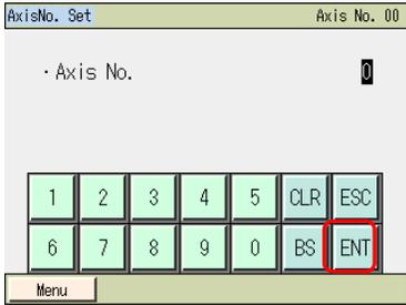
When the numeric keypad appears, enter a desired value and then touch [ENT].
