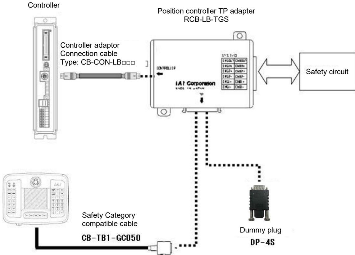
*Note: When not connecting the TB-01D/TB01DR, always insert a dummy plug DP-4S into the position controller's TP adapter.*
