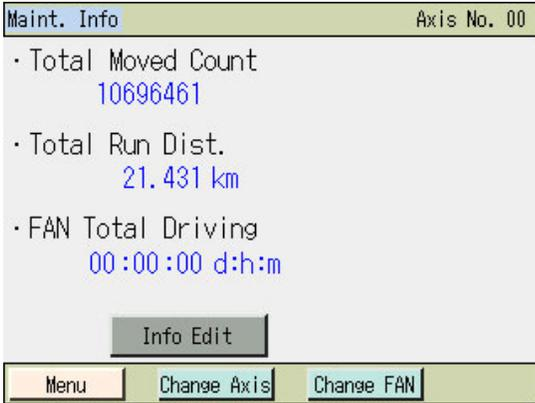
The FAN Total Driving time is reset to 0.
