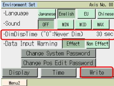
Touching [Dim Display Time ("0": Never Dim) 30 sec] displays the numerical keypad.
