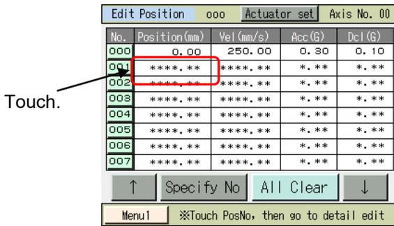
Touch a value in the target position or other field of the desired position data number.
