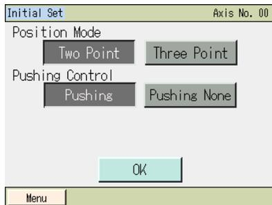
Select and touch either [Two Point] or [Three Point]. To perform positioning operation, select and touch [Pushing None]. To perform push-motion operation, select and touch [Pushing]. To stop at 3 points, select [Both OFF] or [Both ON] as the position specification method.
