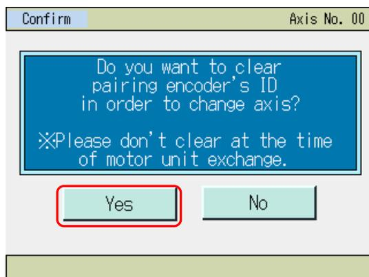
The controller has the mechanism that if the encoder ID is different after checking the ID, then the absolute encoder error is output.
