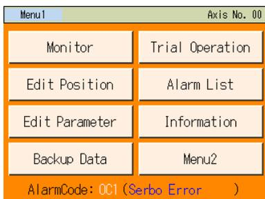
When an alarm generates, the corresponding alarm code and message will appear at the bottom of the screen and the backlight color will change to orange. If an emergency stop is detected, the background color will change to red.
