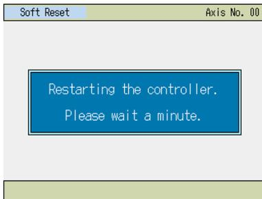
Touch [No], and the controller will not operate according to the factory-set parameters until restarted.
