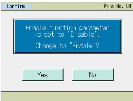
This screen appears when the enable function parameter of the controller, other than TB-01, is set to [Disable]. Select and touch [Yes] (Enable) or [No] (Disable) for the enable function.
