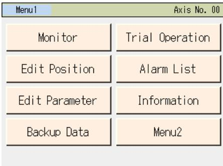
When connection with the controller is established, the Menu 1 screen appears.
