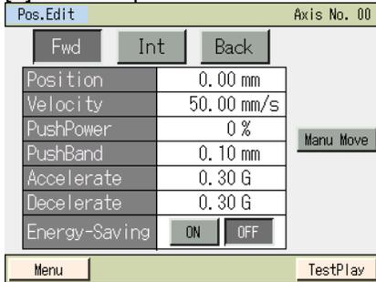
Touch the value field of each setting item such as position. When the numeric keypad is displayed, enter a desired value and then touch [ENT].
