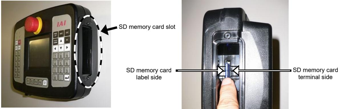
The SD memory card can also be inserted and removed with the following method.
