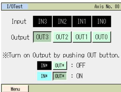
You can monitor the ON/OFF statuses of input signals.
