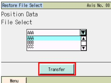
Touch ▲ and ▼ to select a file to transfer to the controller from the list of the backed up file names.
