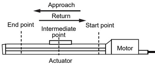
\* In the figure, the home is located on the motor side.
