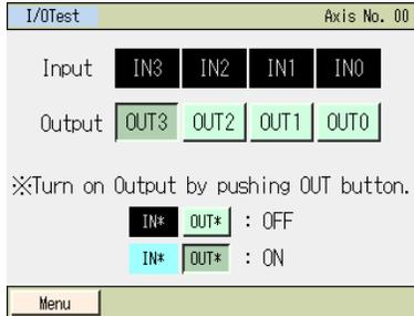
ON/OFF of input signals can be monitored.
