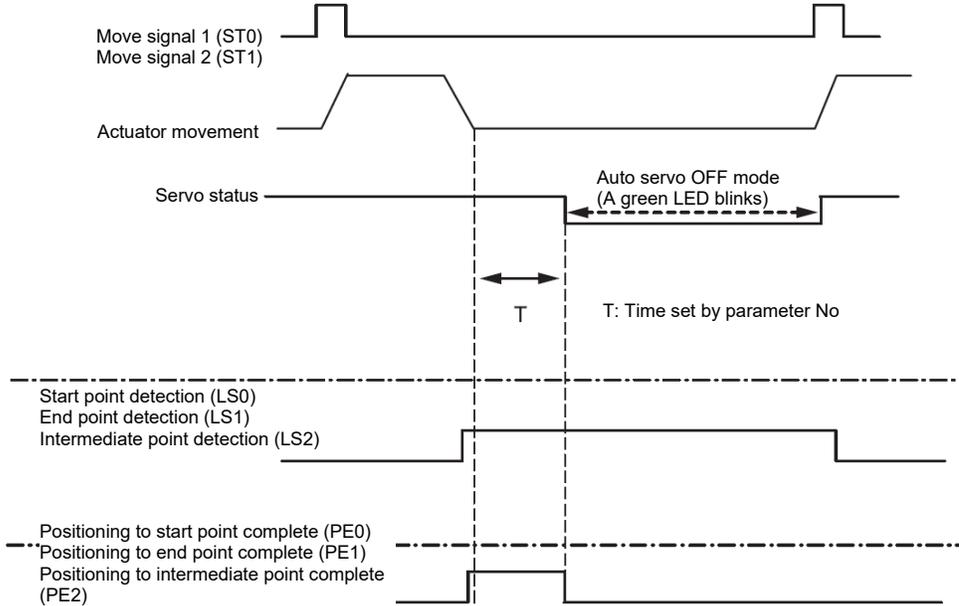
**[Statuses of position detection output signals when the push function is not used]**
