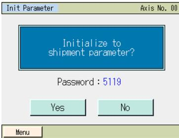
Touching Password displays the numerical keypad. Input "5119" and touch [ENT].
