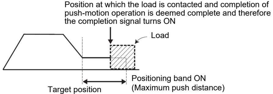
(Note) Depending on the combination with the actuator, PCON-CA/CFA/CB/CFB, SCON-CA/CAL/CB and ERC3 may not be able to set a value smaller than the minimum positioning width.
