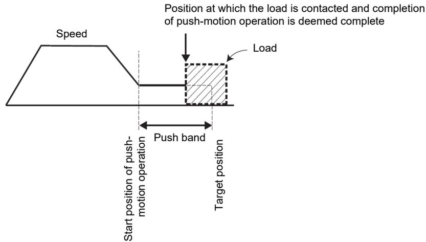
If CON method pressing in Fieldbus Type of MSEP Controllers is selected, the maximum pressing amount in the pressing operation from the target position is defined in Position Mode. While considering the mechanical inconsistency of the work piece, set the positioning band so the positioning would not end before the work piece gets pressed towards the target.
