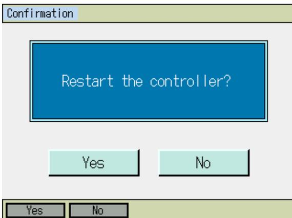
Restart the controller. Touch **Yes** button or press **F1** (OK) key. The display returns to the main menu when the reboot is finished.
