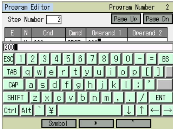
Touch **Keyboard** button to show the touch panel keyboard, input 200 and touch **ENT** button. Or, use the hardware numeric key, input 200 and then press the return key.
