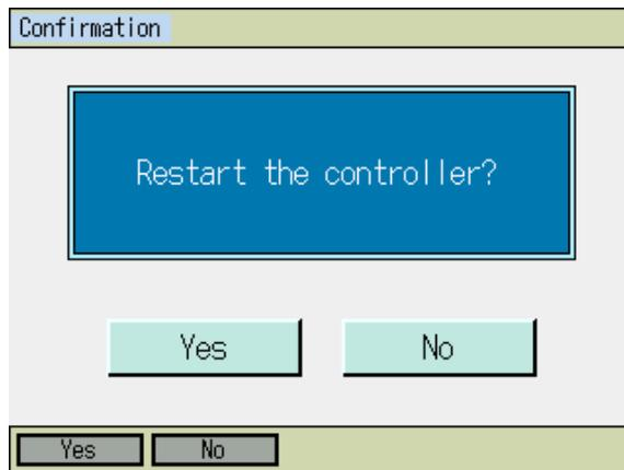
11) After flash ROM writing is complete, the display changes to the Software Reset screen. To activate the parameters that you had changes, it is necessary to have a software reset. Either press **Yes** button in the touch panel or press **F1** (Yes) key.
