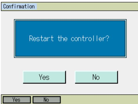
7) After flash ROM writing is complete, the display changes to the Software Reset screen. To activate the parameters that you had changes, it is necessary to have a software reset. Either press **Yes** button in the touch panel or press **F1** (Yes) key.
