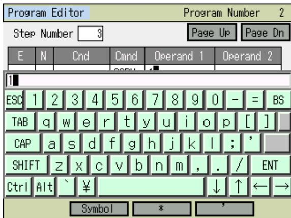
With the cursor being in Operand 1 box, touch **Keyboard** button to show the touch panel keyboard. Input 1 and touch **ENT** button.
