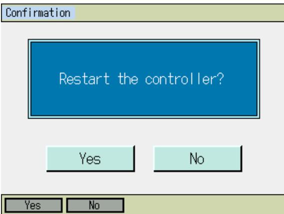
After flash ROM writing is complete, the display changes to the Software Reset screen. To activate the parameters that you had changes, it is necessary to have a software reset. Either press **Yes** button in the touch panel or press **F1** (Yes) key.
