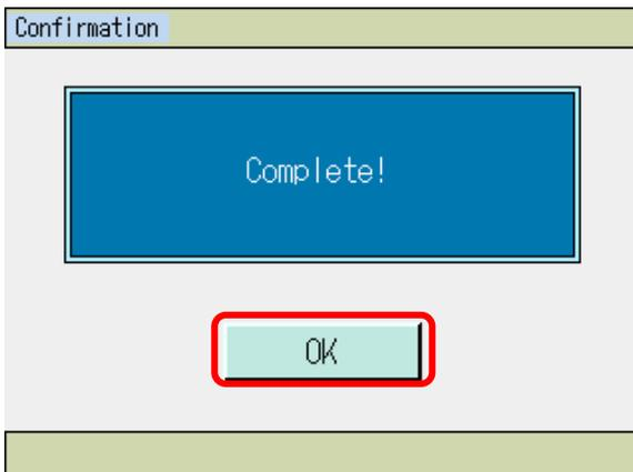
The display shows this screen when the flash ROM writing is finished. If you touch **OK** button, or press **ESC** or **↵** key, the display returns to the restore menu screen.
