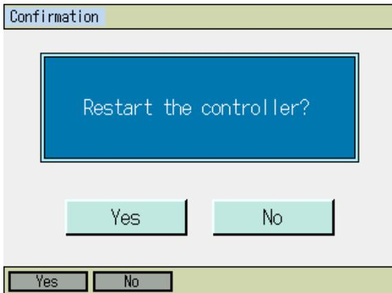
12) Once the flash ROM writing is finished, the screen changes to the window for software reset. Either touch **Yes** button or press **F1** (Yes) key to reflect the pressing position.
