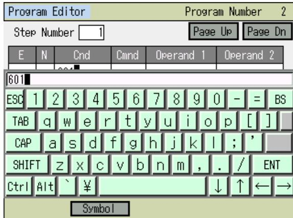
When you use the touch panel keyboard, also input 601 and touch **ENT**. The touch panel keyboard closes and 601 is input in Cnd.
