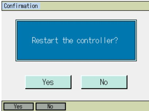
Either touch **Yes** button or press **F1** (Yes) key when you want to have a software reset. When the software reset is not necessary, touch **No** button or press **F2** (No) key. The display returns to Controller Menu.
