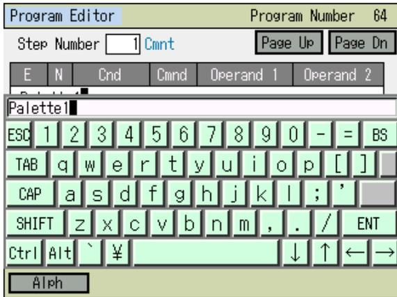
Input desirable letters on the keyboard. Shown in the figure on the left is an example for when Palette1 is input. (To input capital letters, touch **CAP** key or **SHIFT** key to switch the mode.) Touch **ENT** for confirmation. It is also available to input on the hardware numeric keys without displaying the touch panel keyboard.
