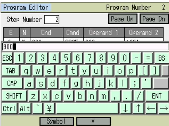
Touch **Keyboard** button to show the touch panel keyboard, input 900 and touch **ENT** button. Or, use the hardware numeric key, input 900 and then press the return key.
