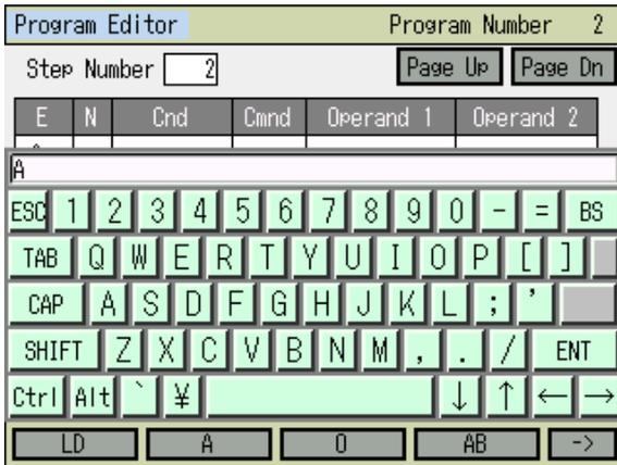
Touch **Keyboard** button to show the touch panel keyboard, input A and touch **ENT** button. When you want to input with the function keys, press **F2** (A) key and then press the return key for confirmation.
