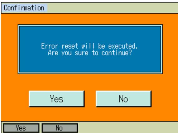
Either touch **Yes** button or press **F1** (Yes) key when you want to have an error reset. When the error reset is not necessary, touch **No** button or press **F2** (No) key.
