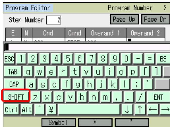
Touch **Keyboard** button to show the touch panel keyboard. Touch **SHIFT** button to switch the letters displayed on the keyboard.
