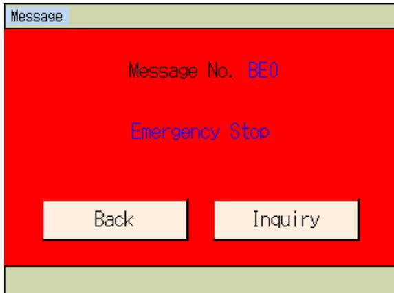
Pressing the EMERGENCY STOP button switches the display to the emergency stop screen.
