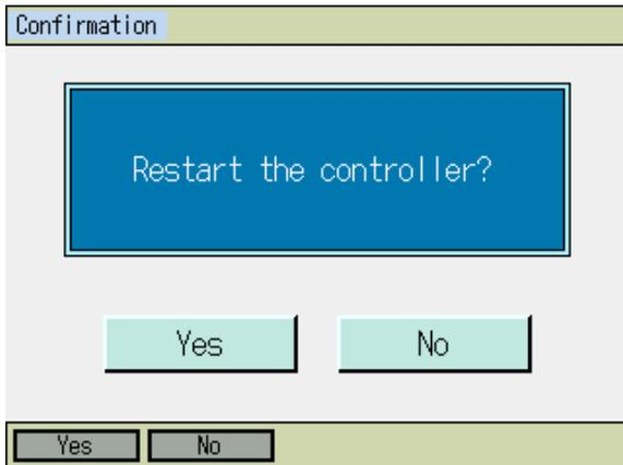
12) Once the flash ROM writing is finished, the screen changes to the window for software reset.
