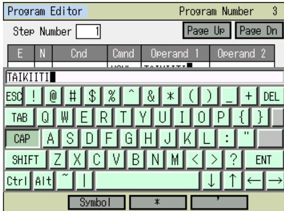
With the cursor being in Operand 1 box, touch **Keyboard** button to show the touch panel keyboard. Input 'TAIKIITI' and touch **ENT** button.
