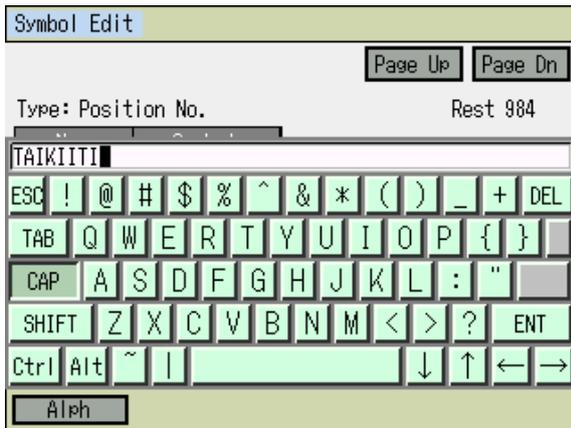
With the cursor being in the symbol input box, touch **Keyboard** button. Input 'TAIKIITI' on the touch panel keyboard and touch **ENT** button. (If you touch **CAP** button, the keyboard changes to capital-letter input. If you touch **CAP** button again, it goes back to small-letter input.) Without showing the touch panel keyboard, it is available to input on the hardware numeric keys.
