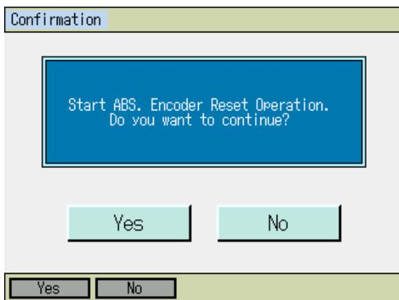
3) To have an encoder error reset, either touch **Yes** button or press **F1** (Yes) key.
