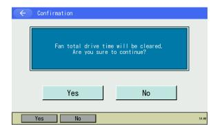
Touch the Yes button when required to clear the fan total drive time. Touch the No button when not required to clear the fan total drive time.
