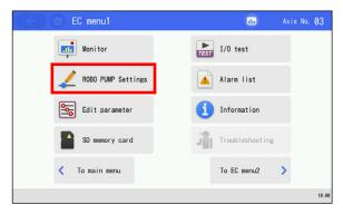
Touch [ROBO PUMP Settings] button on the EC Menu 1 window.
