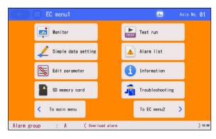
While an alarm is generated, the alarm group (Alarm code for ROBO PUMP) and the alarm name should be displayed at the bottom of the window, and the background should turn into orange.
