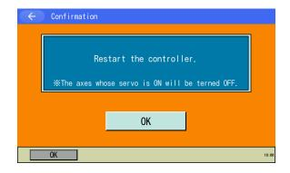
Once the axis number assignment writing is complete, a confirmation window for controller reboot shows up. Touch the OK button. The software reset will be executed.
