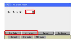
RC alarm reset screen is displayed if <u>Alarm Reset</u> button is touched in RC Monitor screen.
