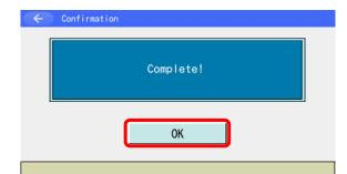
The display shows this screen when the alarm reset is finished. Touch OK button, to return to the RC monitor screen.
