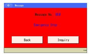
Pressing the EMERGENCY STOP button switches the display to the emergency stop screen. Touch Back button to return to Teaching screen.
