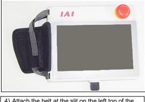
4) Attach the belt at the slit on the left top of the main unit and attach the belt to the grip part with the fabric hook-and-loop fastener.
