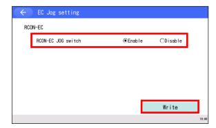
Touch the radio buttons of Enable or Disable for the jog switch, and touch the Write button to transfer the contents of the setting to the controller.
