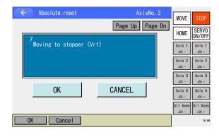
8) Stopper Pressing Movement of Vertical Axis (in Motor Drive) Touch OK button.
