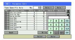
Input 0 on the touch panel numeric keys, and then touch ENT to confirm the input.
