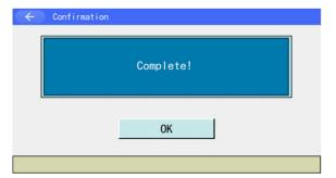
If the initialization of the position data is finished, the display changes to the screen shown on the left
