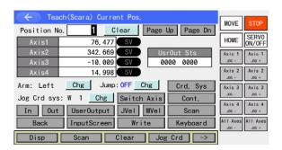
The coordinate values displayed indicate the tool tip position of the tool coordinate system No. 1 on the work coordinate system No. 1.
