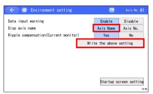
Touch the Axis Name button to switch the setting to the axis name, and then touch the Write the above setting button.
