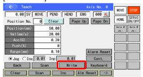
After data input is complete, touch Write button on the touch pane to transfer the data to the controller.
