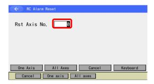
When you want to have an alarm reset only on the indicated axis, set the axis number.
