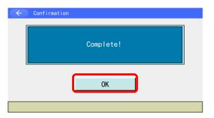
The display shows this screen when the initializing in the user data retaining memory is finished. Touch OK button, to return to the memory initialization menu screen.
