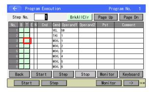
4) Touch a T Button with E being shown while E is shown in the T Button, and the display of E disappears as shown in the figure in the left and the execution time measurement start and end points become not set.
