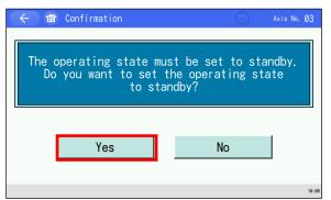
Touch the [Yes] button during suction or release of ROBO PUMP, and the standby confirmation window should appear.
