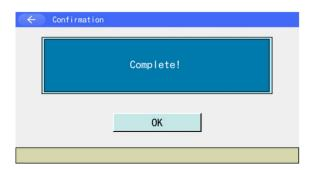
If the recovery of the position data is finished, the display changes to the screen shown on the left. Touch  $\overline{OK}$  button to return to Memory Initialization Menu screen.
