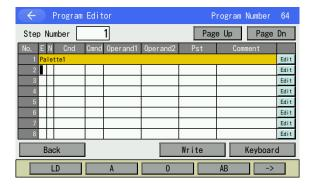
Once the transfer to the controller is complete, the background color in the step number display column will turn to the normal condition.
