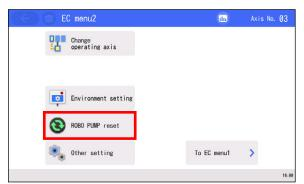
Touch ROBO PUMP reset button on the EC menu 2 window.
