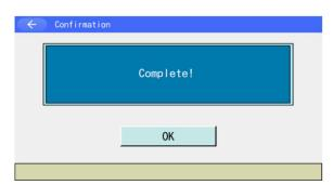
Once the process is complete, the window changes as shown in the figure in the left. Touch OK button, and returns to the memory initializing menu window.
