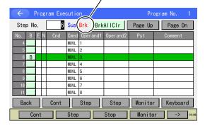
When the continuous operation is carried out with the break point setting established, the program gets paused before executing a command in the step number that the setting is conducted in. To resume the continuous operation after the pause, touch Cont button. Also, if you touch Step button, the step operation starts executed. The break points are all cleared if the power supply to the controller is turned OFF/ON or the software reset is conducted.
