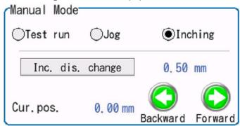
Touch Backward button and an actuator should move backward in a certain distance. Regardless of the backward end setting, the actuator should move backwards till the home position.
