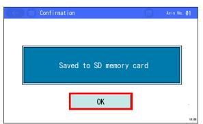
A message to tell the data transfer is complete pops up and the backup process is finished.
