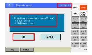
The synchronizing axis absolute reset window should show both of the master axis number and slave axis number as shown in the figure on the left.
