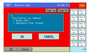
Take the positioning tool off. After taking it off, lock the brake and then cancel the emergency stop button.
