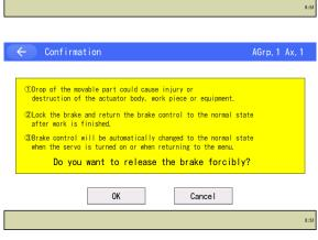
As the screen shifts to the confirmation window, confirm the contents and touch the OK button when having a compulsory release, and touch the Cancel button when cancel.
