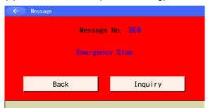
Touch SERVO ON/OFF button and then touch Servo all axes OFF button to turn the servo OFF. Press the EMERGENCY STOP button.
