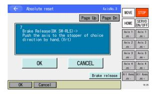
9) Stopper Pressing Movement of Vertical Axis (in Manual) Set the brake release switch to the RLS side or touch the Brake release button (when the button is activated) to release the brake in the confirmation window. Push the vertical axis against the stopper with hand.
