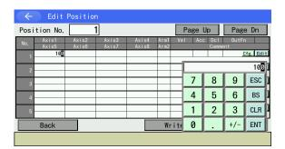
If you want to input 100 to Axis1 (1st axis), touch Keyboard button to show the touch panel numeric keys, and touch 100ENT on the touch panel numeric keys.
