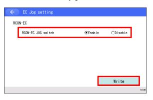
Touch the radio buttons of Enable or Disable for the jog switch, and touch the Write button to transfer the contents of the setting to the controller.
