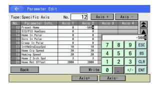
After touching ENT, touch Write button to transfer the data to the controller.
