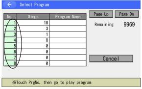
Touch the number box (where marked with a circle in the figure in the left) on the table of the program number that you would like to run the program in. To show No. 9 and further, use Page Up and Page Dn buttons to change the display.
