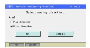
6) Selection for Moving Direction of Arm1 (2) The vicinity stopper position direction is selected as the moving direction in the initial setting.
