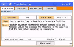
The figure shown on the left is detail display with an alarm code in the troubleshooting window.
