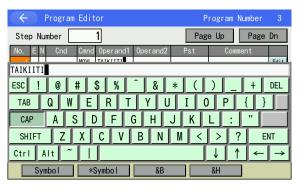
With the cursor being in Operand1 input box, touch Keyboard button to show the touch panel keyboard. Input 'TAIKIITI' and touch ENT.
