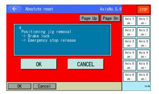
7) Take the positioning tool off. After taking it off, lock the brake and then cancel the emergency stop button.
