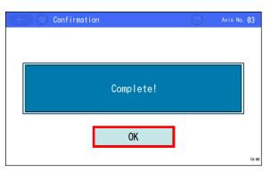
The complete confirmation window should appear once the data transfer of data for all of the ELECYLINDER or ROBO PUMP units is complete.
