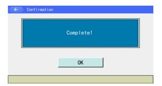
If the recovery of the program data is finished, the display changes to the screen shown on the left. Touch  $\boxed{\mathsf{OK}}$  button to return to Memory Initialization Menu screen.
