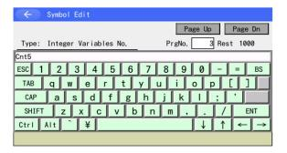
To input 'C', touch SHIFT and then touch C. The keyboard automatically returns to small letter input. Continue to type in 1 5, and touch ENT.
