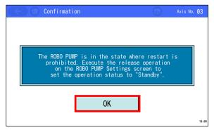
The reboot prohibited window should show up when reboot is conducted while ROBO PUMP is in suction or release.
