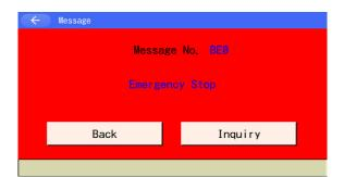
Pressing the EMERGENCY STOP button switches the display to the emergency stop screen.
