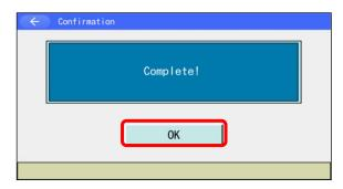
The display shows this screen when the data transfer is finished.
