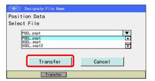
Touch ▲ and ▼ to select a file to transfer to the controller from the file list in a SD Memory Card.
