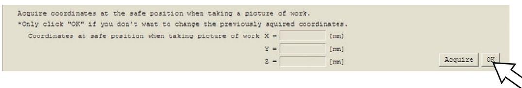
[Procedure 18] With the work held on the robot, transport it to a position near the calibration start point (point above the position 0 set in Procedure 8 (5)). Do not move the robot from where it released the work. Click “OK” button.
