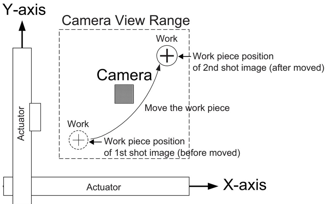
[Procedure 11] Capture an image of the work piece and input the vision system coordinates (X coordinate and Y coordinate) detected on the vision system side. After inputting, click “Acquire” button.
