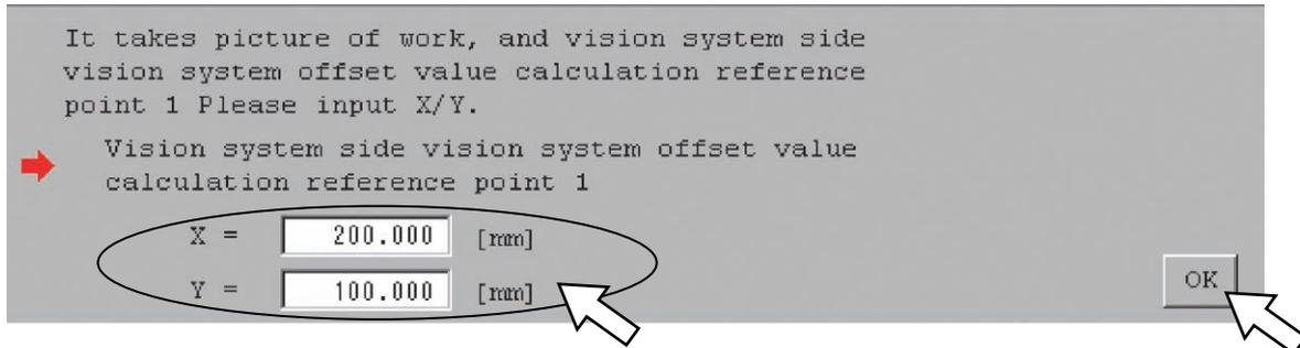
[Procedure 8] Match a tool head to the detection reference point. Click "OK" button.
