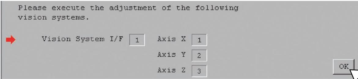
[Procedure 6] Move the robot to a position closest to the origin within the operation range. Set the work piece on the top left corner of the image capture range. Click "OK" button after the setting is complete.
