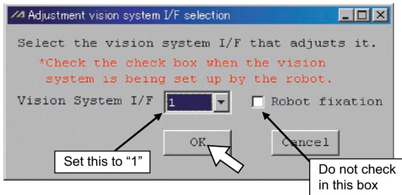
[Procedure 4] Confirm that the vision system is installed within the range of the robot operation and click "OK" button.
