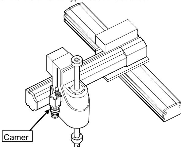
When Camera Mounted on Robot
