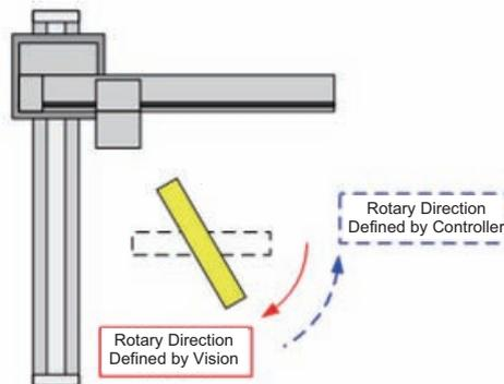
Figure: Example When Rotary Direction Unmatched
