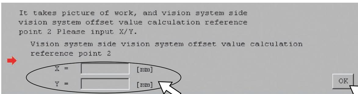
[Procedure 12] Match a tool head to the detection reference point. [Refer to [Procedure 8] in Section 5.8.4] Click “OK” button.
