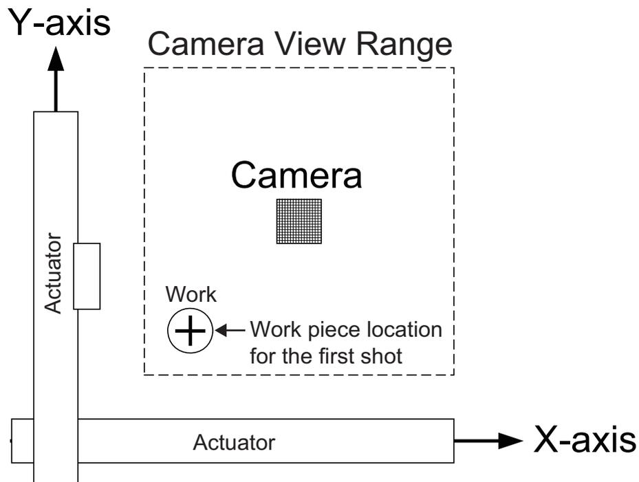
[Procedure 7] Capture an image of the work piece and input the vision system coordinates (X coordinate and Y coordinate) detected on the vision system side. After inputting, click "OK" button.
