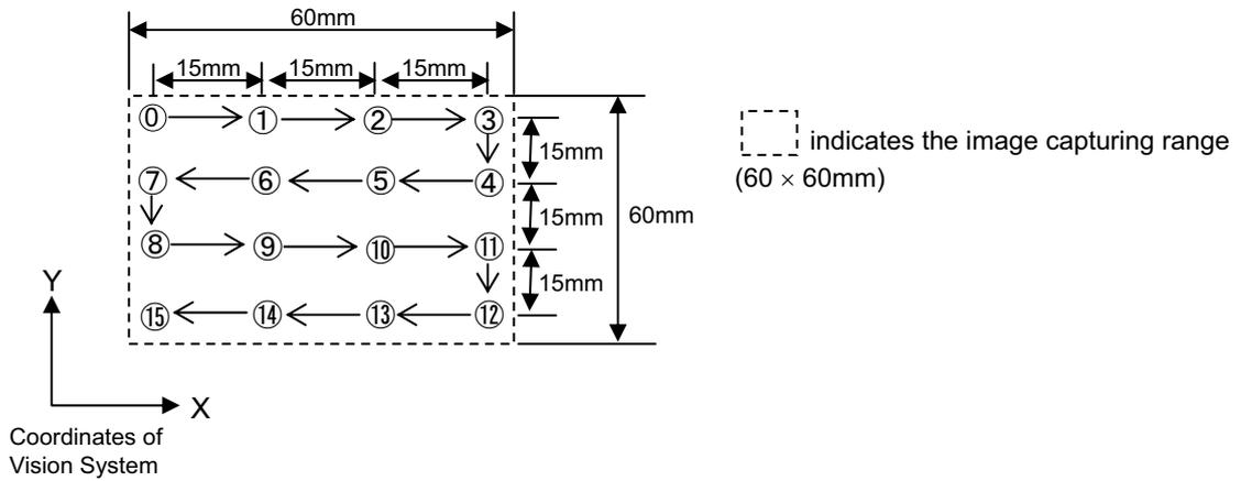
In this example, select the Move tag and set the values as shown below for Move1.X to Move15.Y in the right order.
