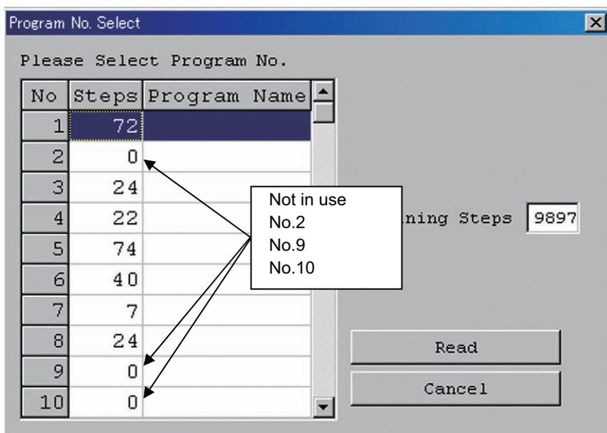
[Procedure 13] Input the position number not in use. (Select a position number that 10 positions in a row can be ensured.)
