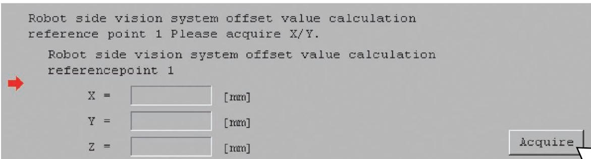
[Procedure 8] Capture an image of the work piece and input the vision system coordinates (X coordinate and Y coordinate) detected on the vision system side. After inputting, click "OK" button.
