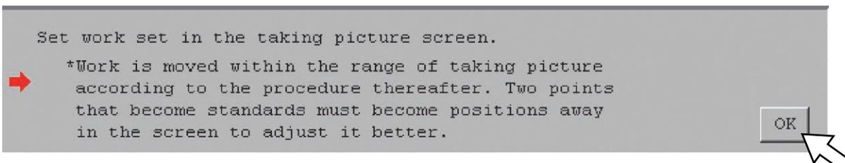
There will be 2 times that the image capturing is required in the vision system I/F adjustment procedure. Set the work piece within the image capture range considering it is placed as far as possible from the camera as shown in the following diagram.
