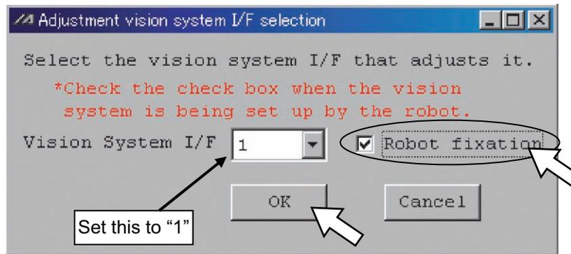
[Procedure 4] Confirm the vision system is installed on the camera and click “OK” button.
