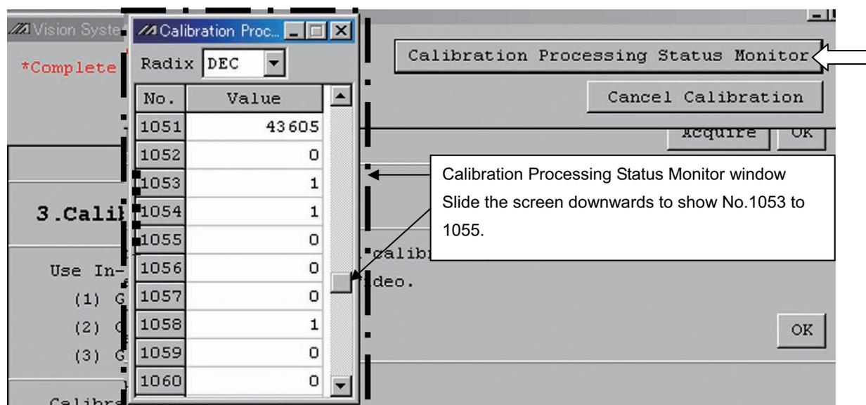
Check the value in No.1053 and find the corresponding error number to take an appropriate counteraction.
