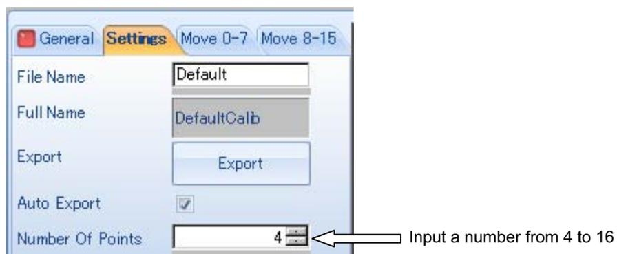
(7) Set the amount of robot movement<sup>(Note 1 and 2)</sup> considering the set points are in the image capturing range.
