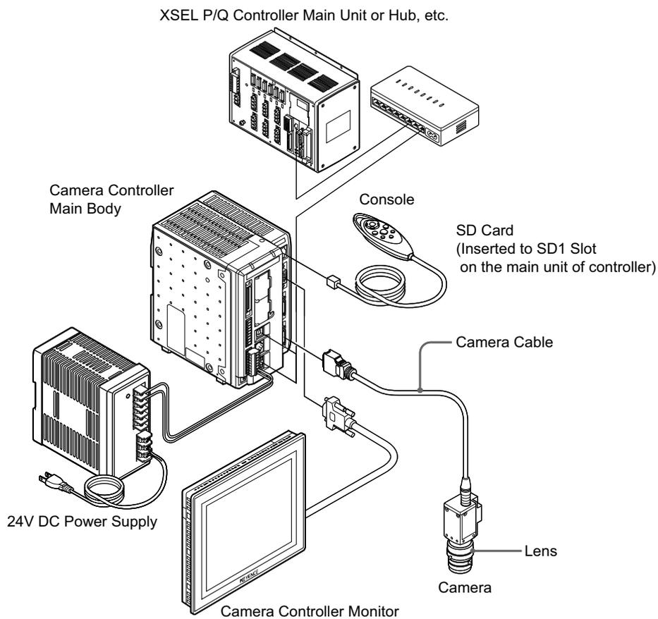
Example for Keyence Camera Controller Basic Construction
