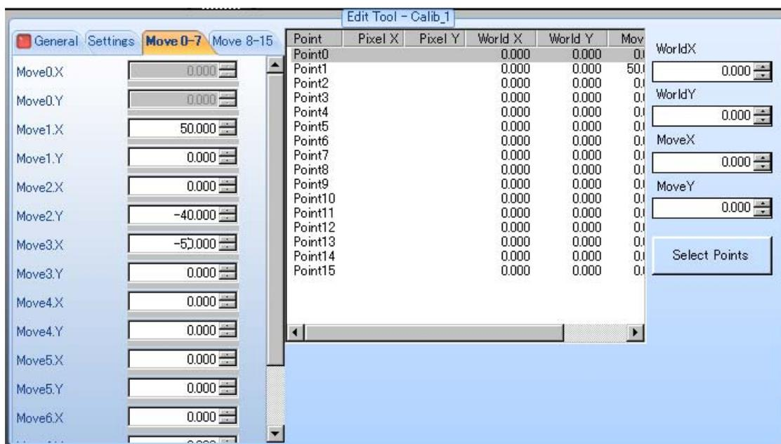
Example 2 : Number of Calibration Points = 16 points (When Camera Not Mounted on Robot)
