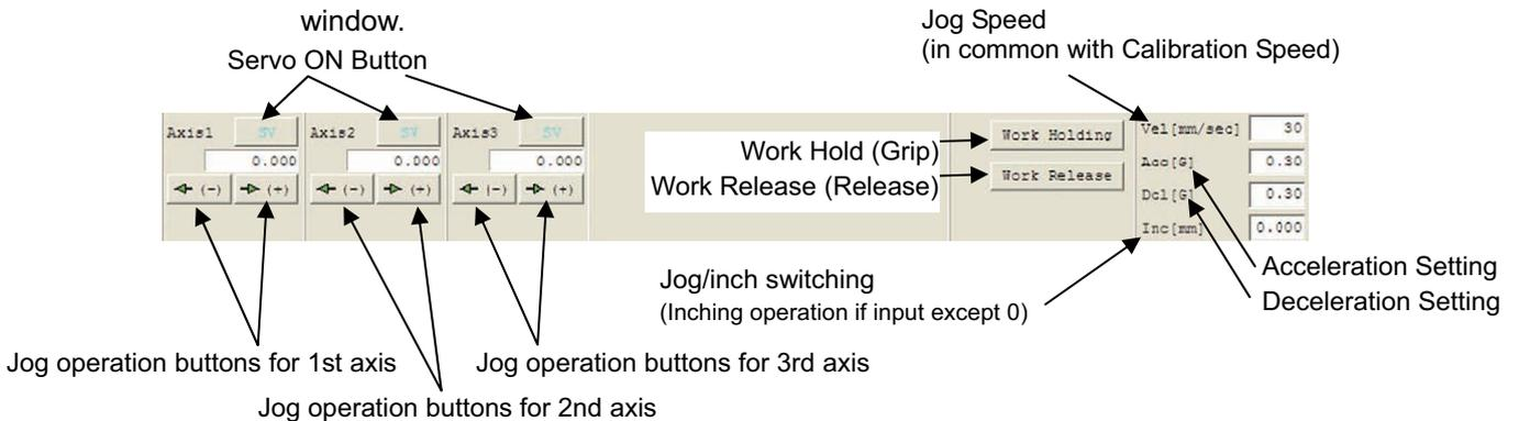
[Procedure 16] With the work held on the robot, transport it to a position near the calibration start point (point above the position 0 set in Procedure 8 (5)).
