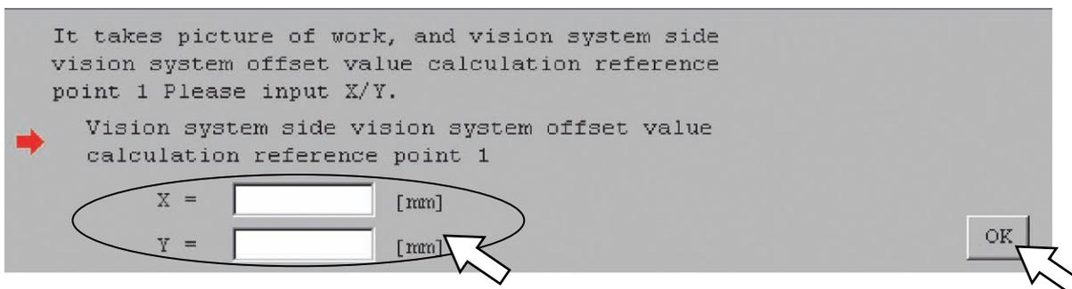
[Procedure 9] Move the robot so the work piece is placed on the bottom right corner of the image capture range. Click "OK" button after it is moved.
