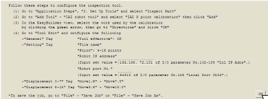
(1) In Application Steps in In-Sight Explorer, select “Set Up Tools” → “Inspect Part”.
