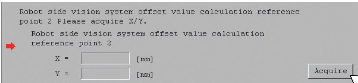
[Procedure 11] Capture an image of the work piece and input the vision system coordinates (X coordinate and Y coordinate) detected on the vision system side. After inputting, click “OK” button.
