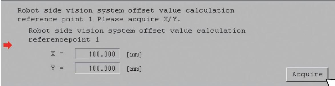
[Procedure 10] Set a work piece in the range of robot operation and also the top right (refer to the diagram below) of the image capture range, and then click “OK” button.
