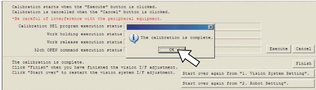
[Procedure 24] If desired to finish the calibration, click the "Finish" button.
