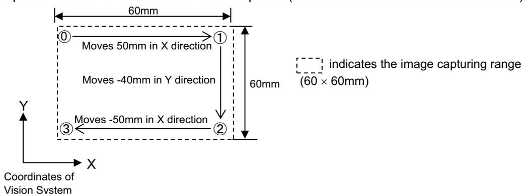
In this example, select the Move tag and set the values as shown below for Move1.X to Move3.Y in the right order.
