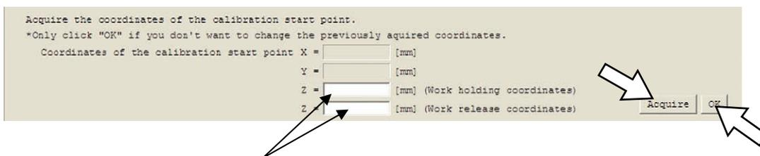
Put values directly when a fine-tuning is required for the Z-axis height.
