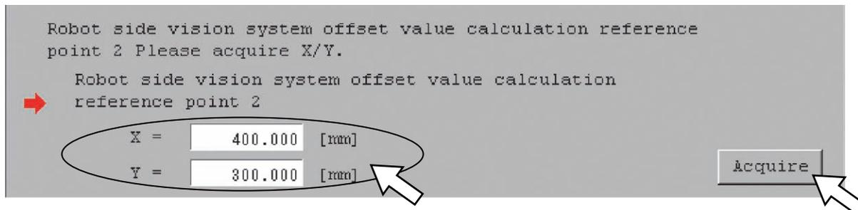
[Procedure 12] Match a tool head to the detection reference point.
