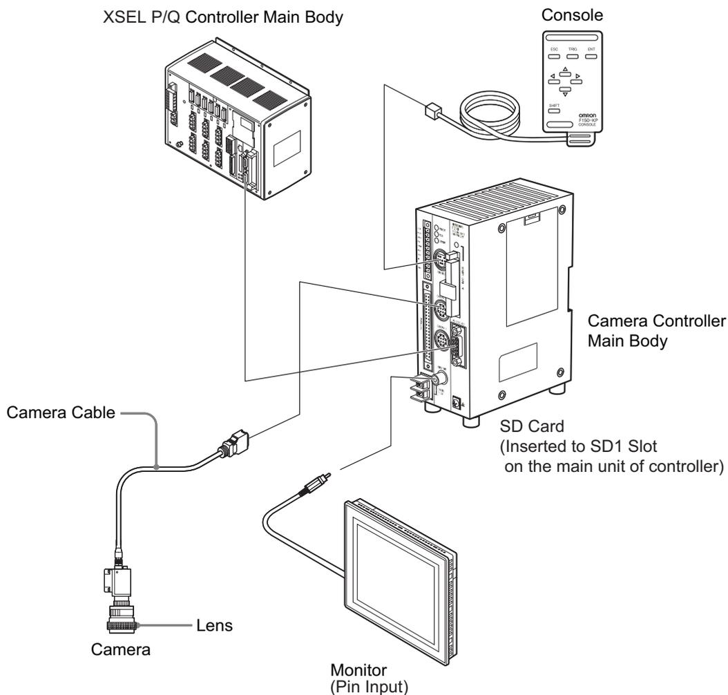
Example for OMRON Camera Controller Construction (for F210-C10)
