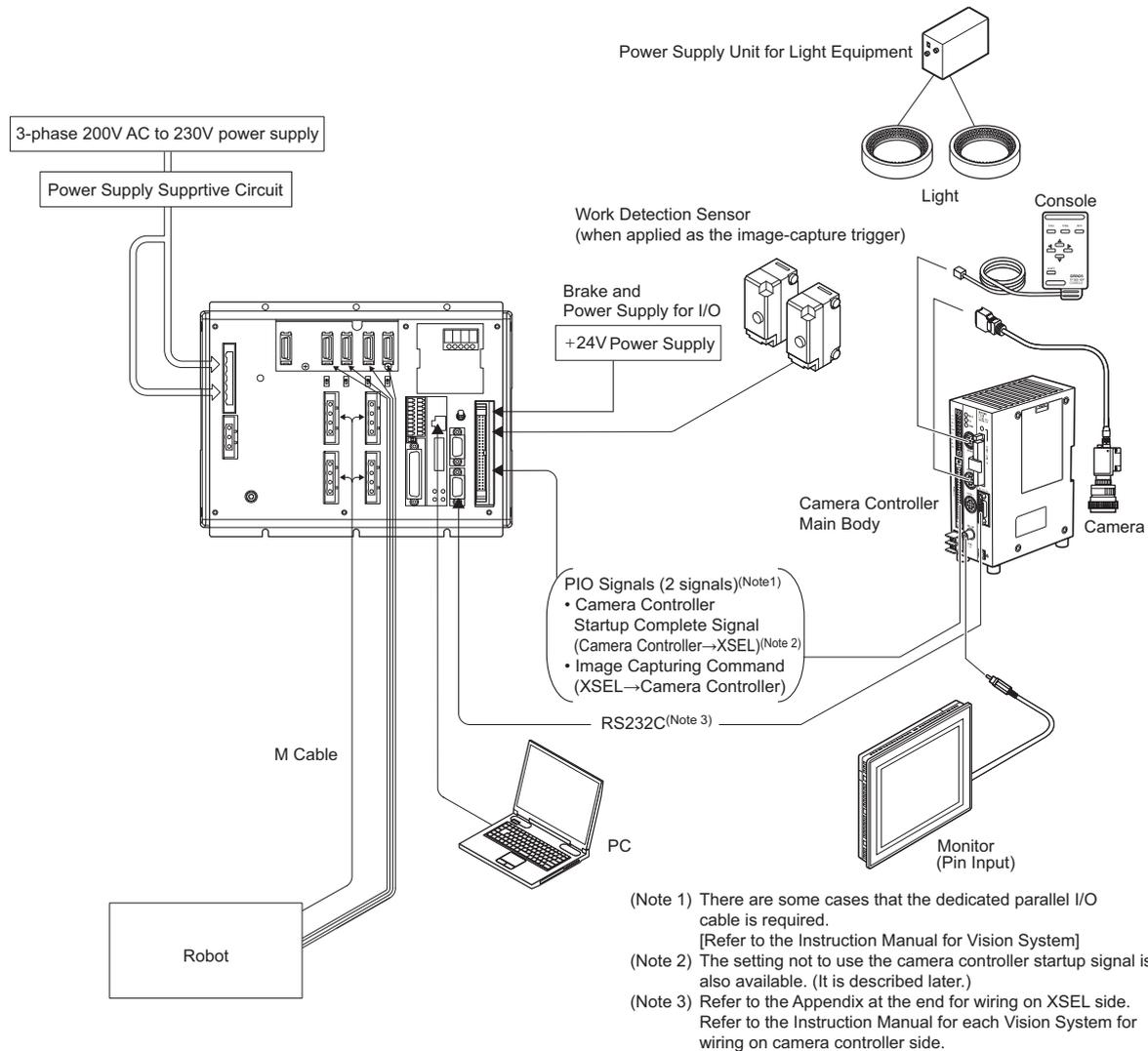
Example for Vision System Wiring (OMRON)
