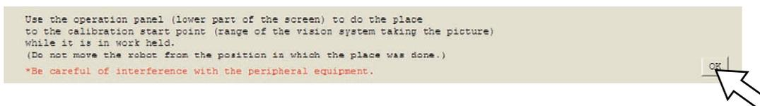
Perform the moving operation with the jog buttons at the bottom of the calibration window. [Refer to Procedure 15]
