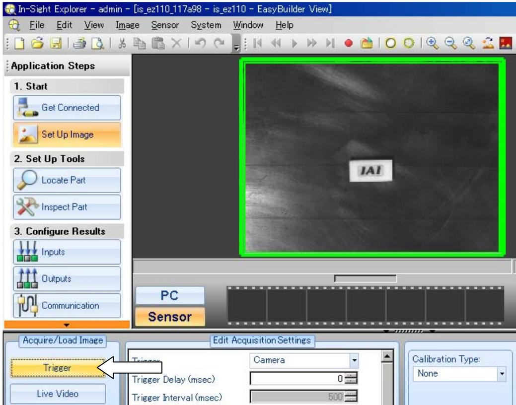
[Procedure 7] Select the necessary tools<sup>(Note)</sup> from the positioning or inspection of the tool setting.
