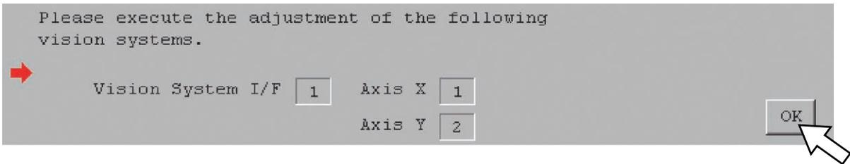
[Procedure 6] Set a work piece in the range of robot operation and also the bottom left (refer to the diagram below) of the image capture range. After the setting is complete, click "OK" button.
