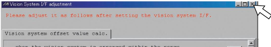
[Procedure 17] If the vision system adjustment is implemented, the following dialog box appears after Vision System I/F adjustment window is closed. Click “Yes” button.
