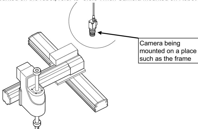
When Camera Not Mounted on Robot
