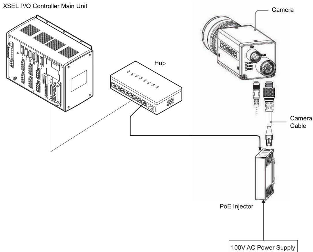
Example for Cognex Camera Controller Basic Construction
