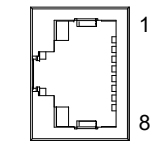
Front View of Connector on Controller side
