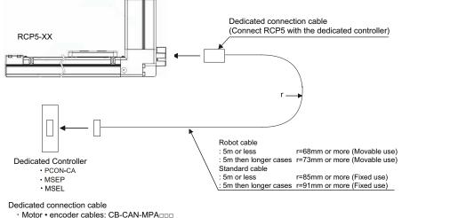
• Motor • encoder cables robot type: CB-CAN-MPA
