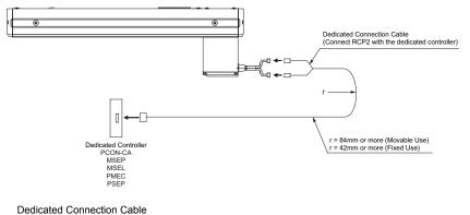
Motor Encoder Cable CB-PSEP-MPA □□□ shows the cable length. The max. length should be 20m.
