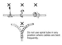
Separate the I/O line, communication line and power line from each other. Arrange so that such lines are independently routed in the duct.
