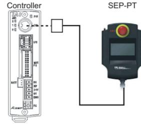
**Note :** Do not connect SEP-PT to the SIO converter. Failure to do so may result in a breakdown.
