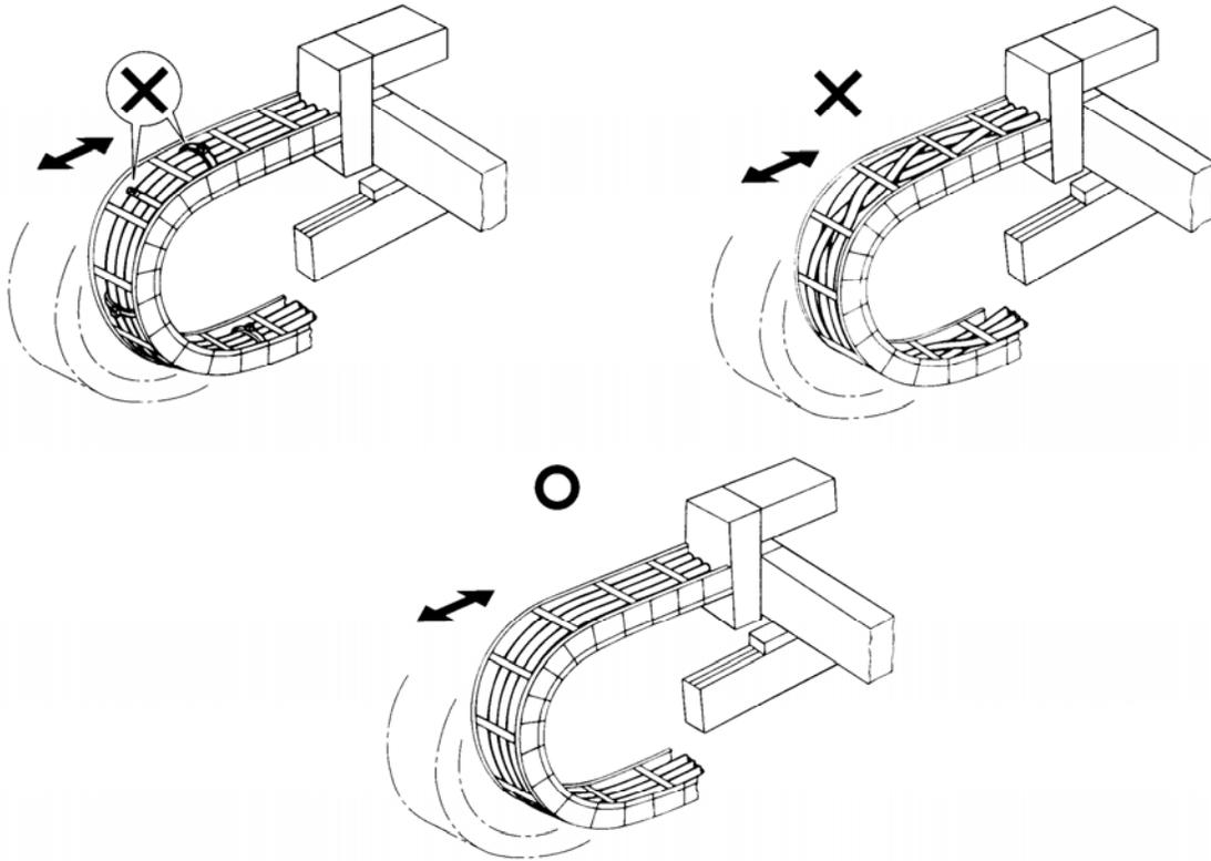
8. Do not cause the cables to occupy more than 60% of the space in the cable bearer. Do not place the connector in the cable bearer.
