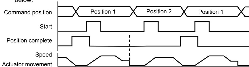
If the actuator has missed the load, the position complete output will not turn ON.
