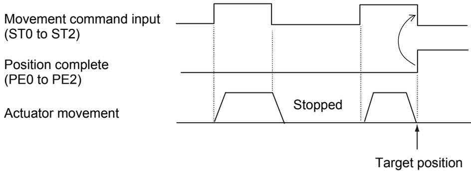
(Note) Turn OFF the movement command input after confirming that the target position has been reached.
