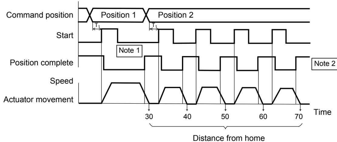
T1: 6 msec or more; time after selecting/entering a command position until the start input turns ON
