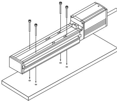
Install the actuator in the mounting holes provided in the base. Secure the actuator in place using M4 hex cap bolts.
