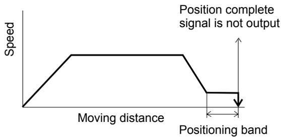
(1) After reaching the target position, the actuator will move at low speed. Even after contacting the load, the actuator will move to the end of the positioning band if the stepper motor current is yet to reach the current-limiting value. The position complete output will not turn ON even when the end of the positioning band is reached. (Provide a timeout check process after a sufficient period with a PLC.)
