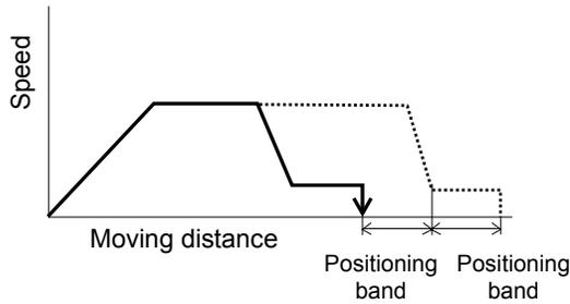
If the positioning band is entered with a wrong sign, the position will deviate by twice the positioning band, as shown to the left, so exercise due caution.
