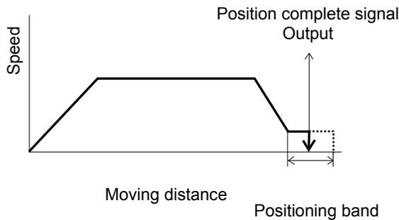
(1) After reaching the target position, the actuator will move at low speed (75 rpms). When the Pos. band set in the data table (see Note) is reached after the actuator contacts the load and the stepper motor current has reached the current-limiting value, the position complete output will turn ON.
