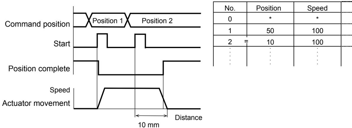
(3) Cumulative errors due to repeated incremental moves
