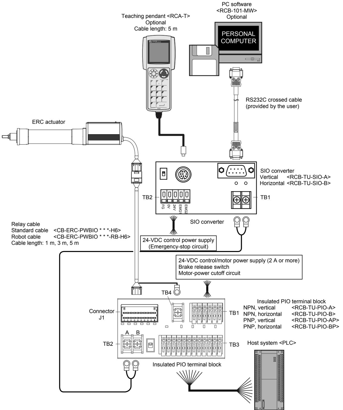
**Note:** Do not connect a teaching pendant and a PC at the same time. If both are connected at the same time, a communication error (message level) will occur.
