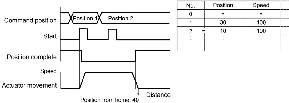
If the start signal for movement to an incremental position number is input multiple times during positioning, the actuator will move to the position corresponding to the initial position plus the "increment x number of times the signal was input."
