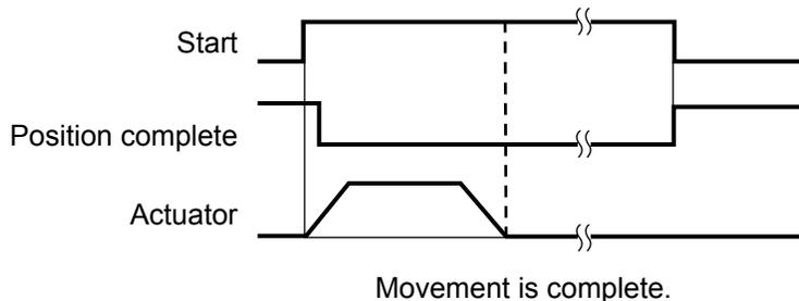
Note 2: When a soft limit is reached as a result of repeated incremental moves, the actuator will stop at that position and the position complete signal will be output.
