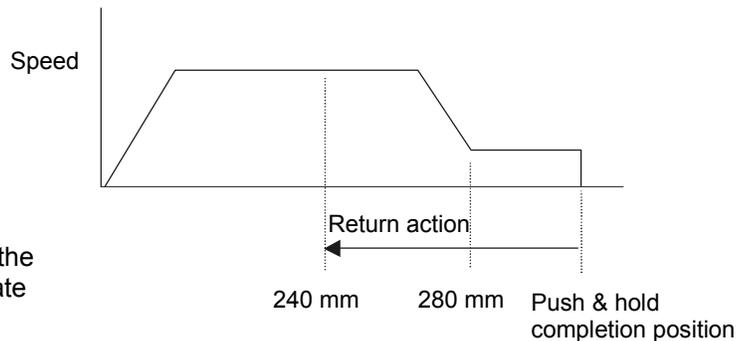
Note: When the start signal turns ON, the position complete output will turn OFF.
