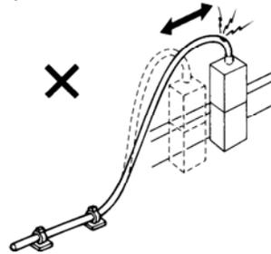
4. Do not let the cable receive a turning force at a single point.
