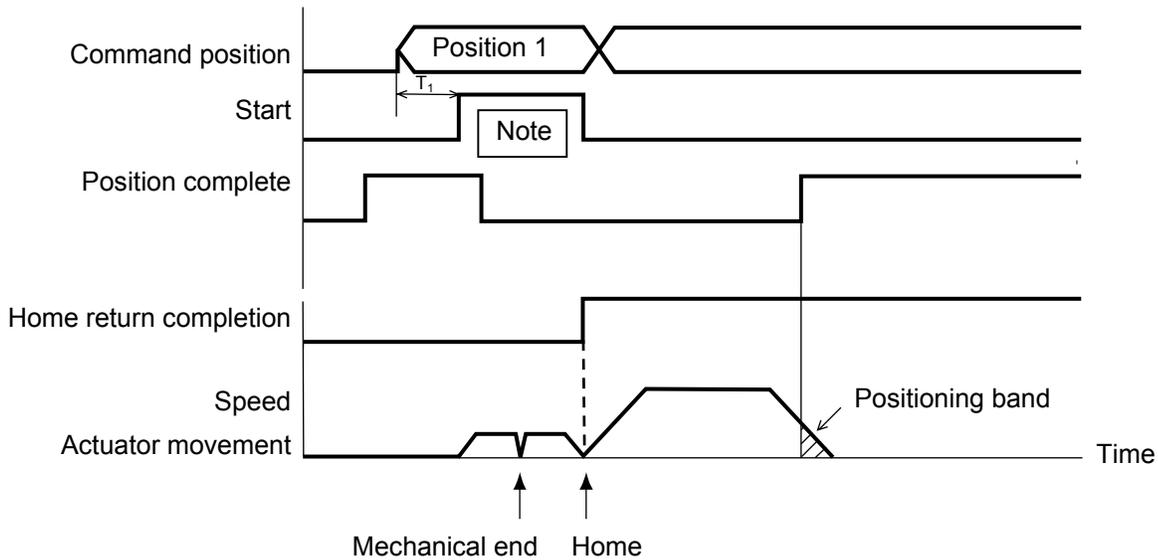
The position complete output will turn ON when the controller becomes ready following the power ON. To check if the controller is ready, always check if the position complete output is ON.
