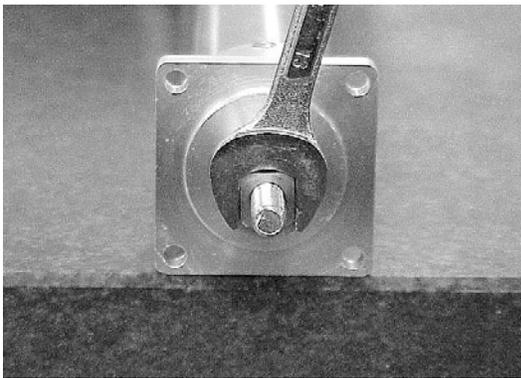
Note) Apply a spanner at the rod end bracket to prevent the rod from receiving any rotating moment when the load is installed. Applying excessive rotating moment to the rod may damage the rod.
