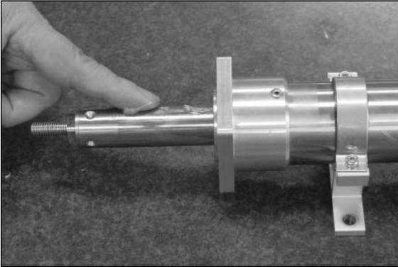
**!** Note to the user: Never use fluorine grease. If fluorine grease is mixed with lithium grease, the grease function will drop and it causes damage to the mechanism.
