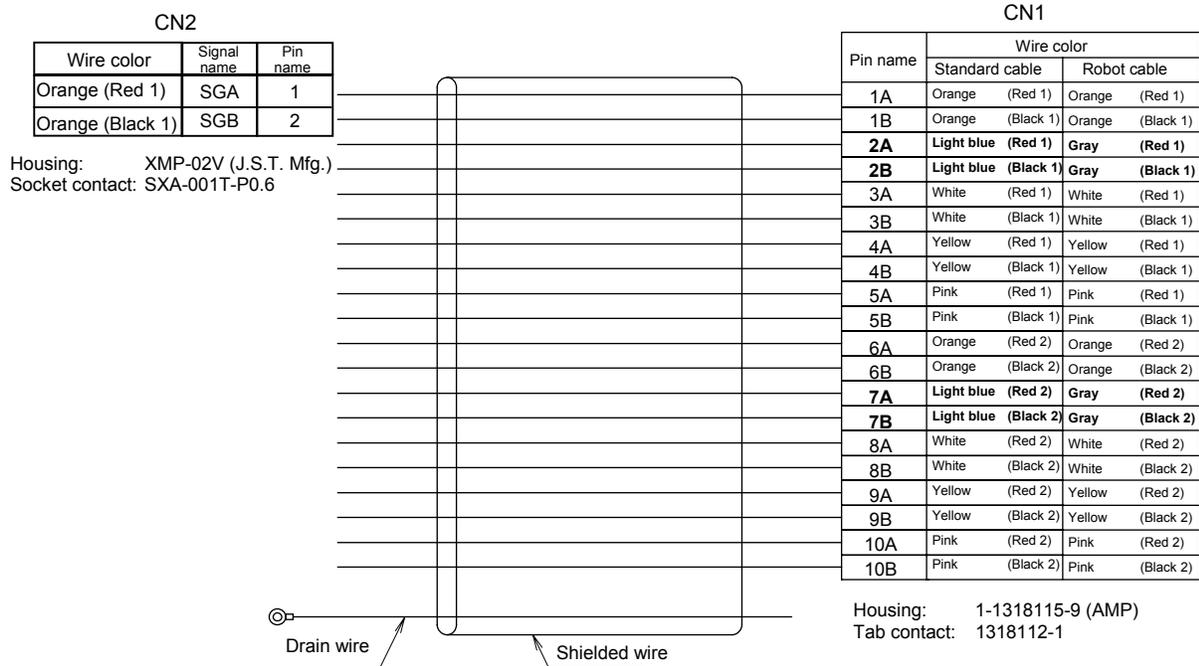
(Supplied cables to be connected to CN2)
