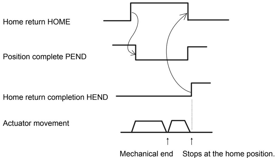
**Note:** When the home return signal turns ON, the position complete output will turn OFF. Always turn OFF the home return signal after confirming that the home return completion output has turned ON.
