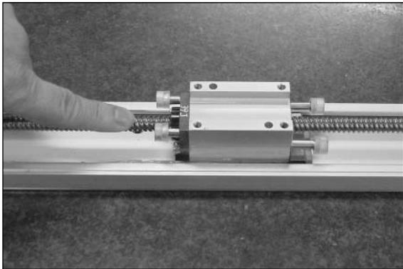
After cleaning the ball screw, apply grease and stroke the slider to let the grease spread evenly. As the final step, wipe off excess grease from the ball screw.
