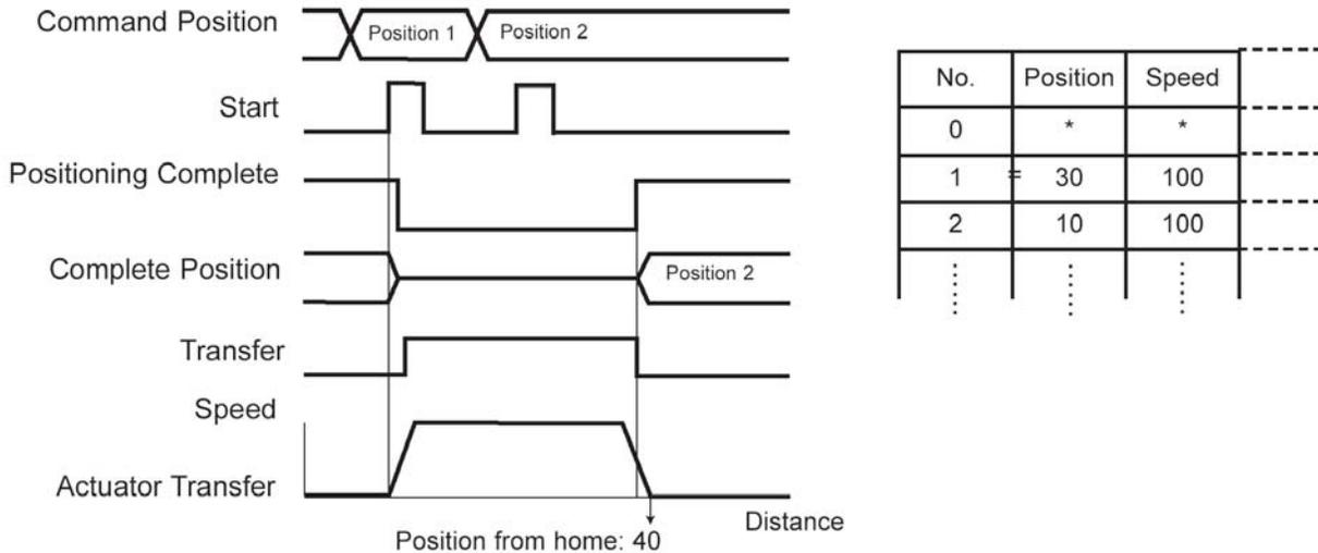
Position from home: 40 In addition, when the Start Input is executed numerous times during position movement, the actuator moves to a position that is five times the distance of the initial position input.
