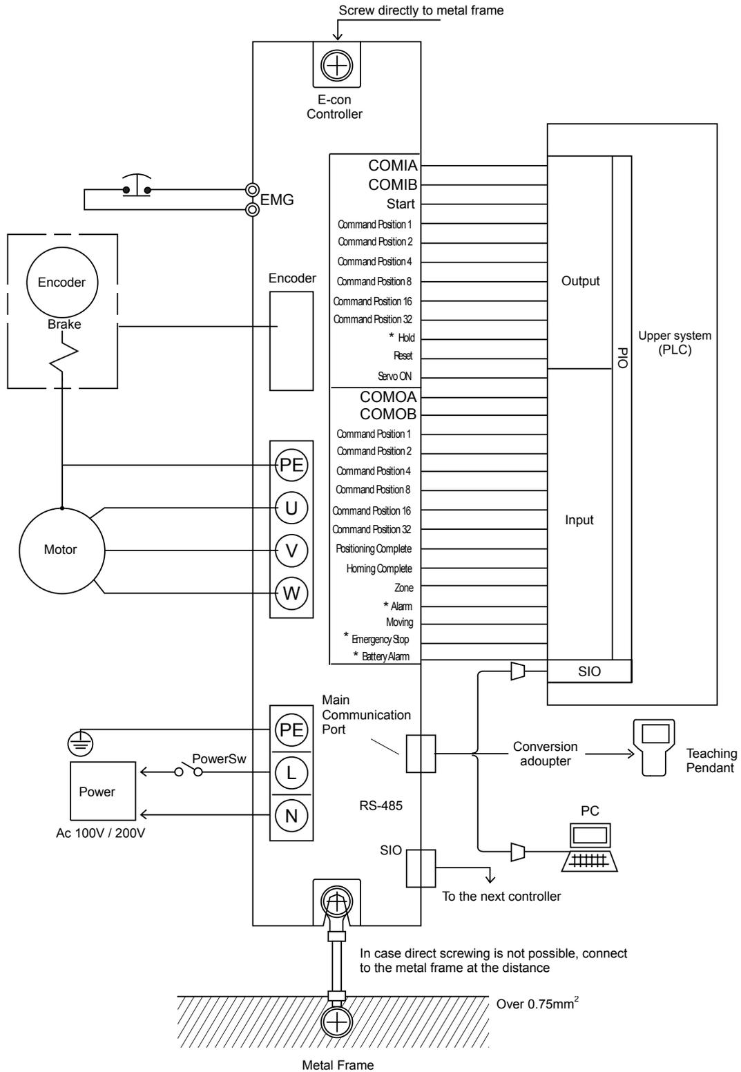
(Note) \*Hold, \*alarm, \*emergency stop and \*battery alarms are contact-b signals.
