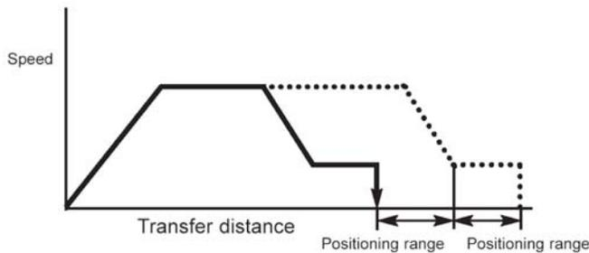
When a mistake is made in the code for the positioning width data, as the left diagram shows, only the width (positioning complete width x 2) will be off, so please be careful
