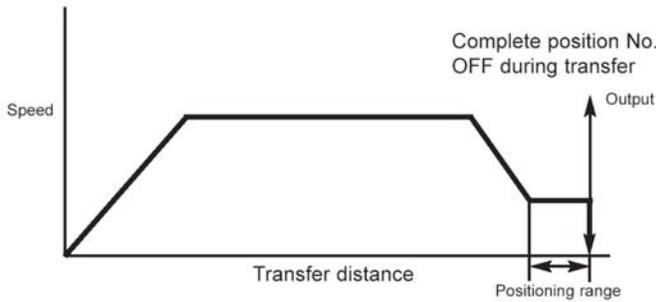
(1) Upon reaching the position, the actuator moves forward at a low rate speed. When the servo motor current does not reach the peak current restriction value in the positioning band, the positioning completion output will not turn ON even when the actuator moves to the positioning band range. In this case, only the complete position number outputs turn ON. To confirm stop status, check if output during transfer is OFF.
