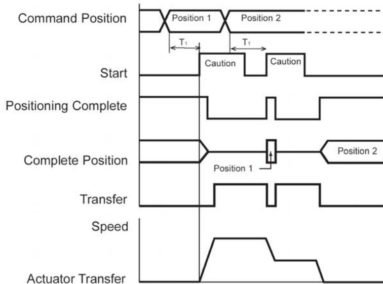
T1: Over 6 msec Time from Command Position Select Input to Start Signal ON
