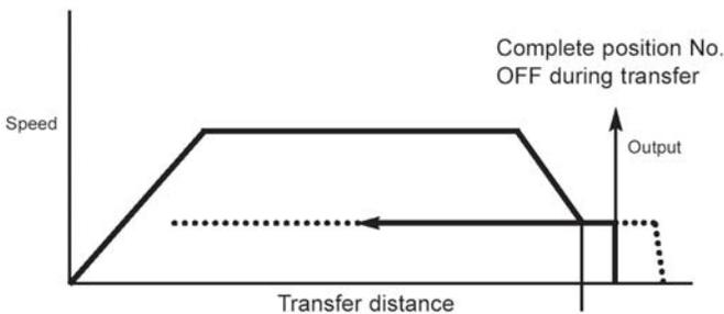
When the reaction force of the work is greater than the push force of the actuator, and the actuator is pushed back after the positioning complete output turns ON, the actuator will be pushed back until the forces balances out. The positioning complete ON and complete position number outputs will not change. In-motion output will remain ON until motion stops.
