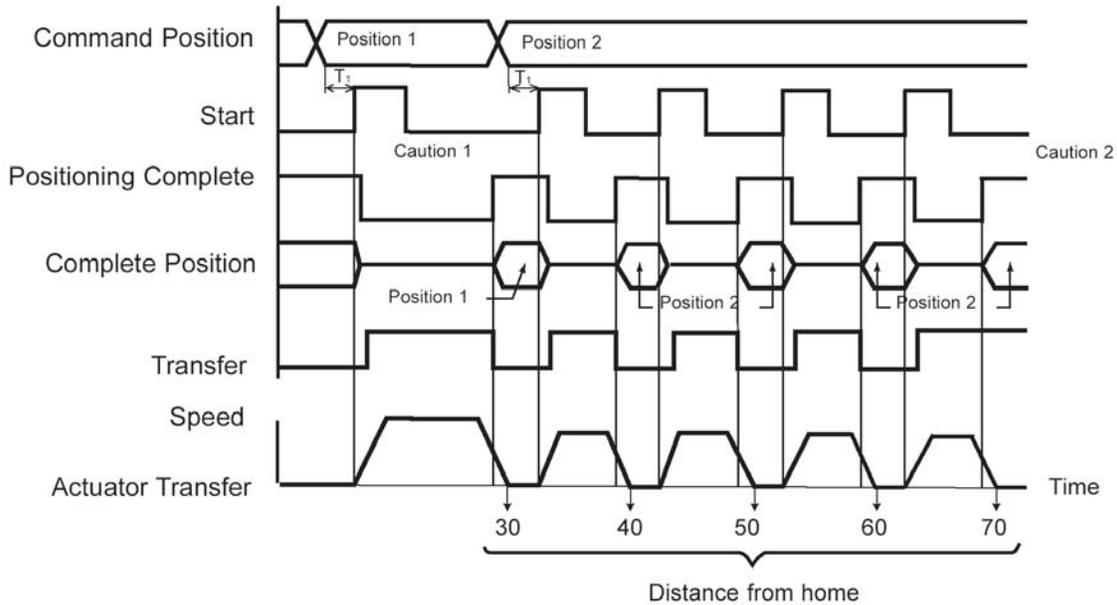
T1: Over 6 msec Time from command position select input to start input ON
