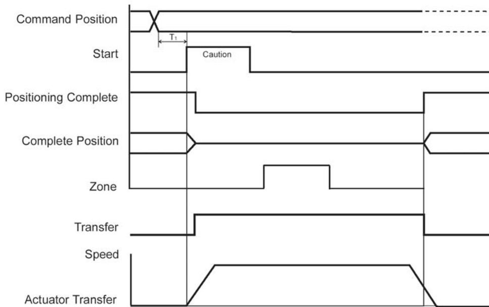
$T_1$ : Over 6 msec Time from command position select input to start input ON
