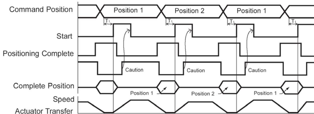
T1: Over 6 msec Time from Command Position Select Input to Start Signal ON
