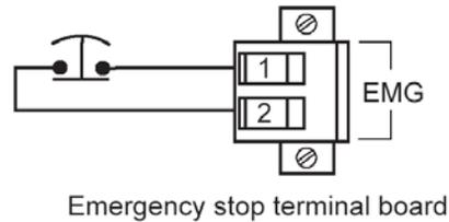
\* The two EMG terminals are for connecting an emergency stop switch. At the time of shipment, a jumper is used to short the two terminals. Do not remove it! If you remove, replace with a switch that is normally closed, or the system will always be in emergency status. 24 VDC is output to pin 1.
