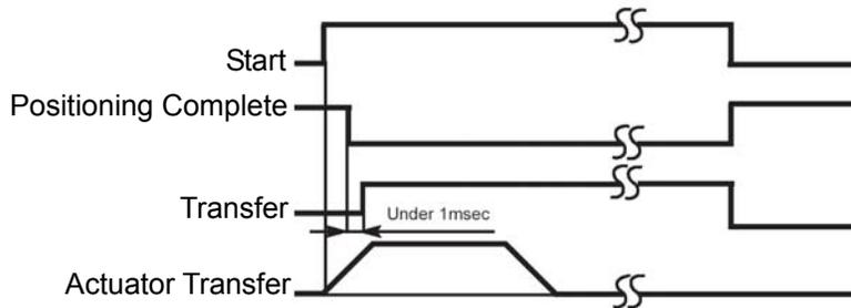
If an overload alarm occurs frequently when this function is used, disable the "acceleration only MAX" function.
