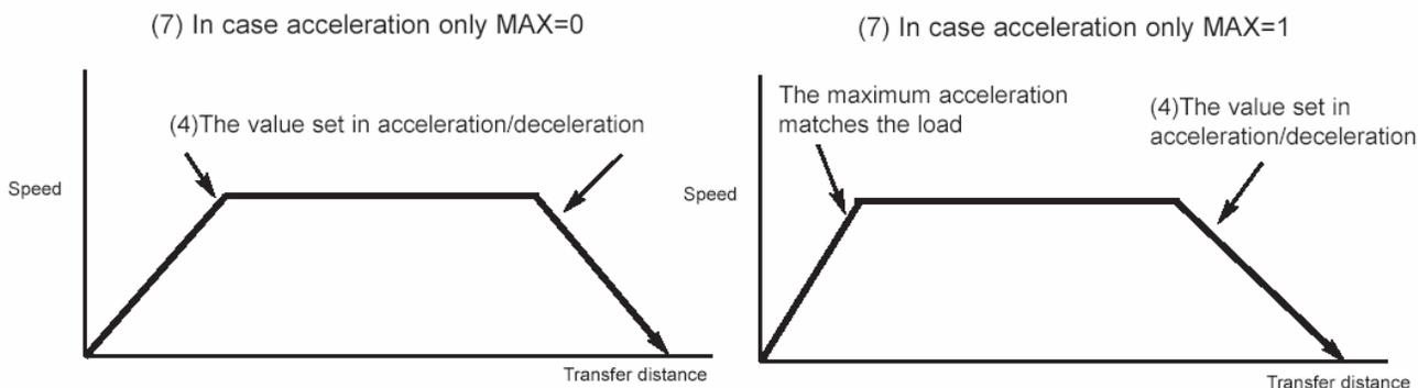
**Caution:** As a rough guide, enable the acceleration only MAX setting when the actual payload is no more than one-third of the rated loading capacity. Check the rated loading capacity of your actuator by referring to the supplied specification list of supported actuators.
