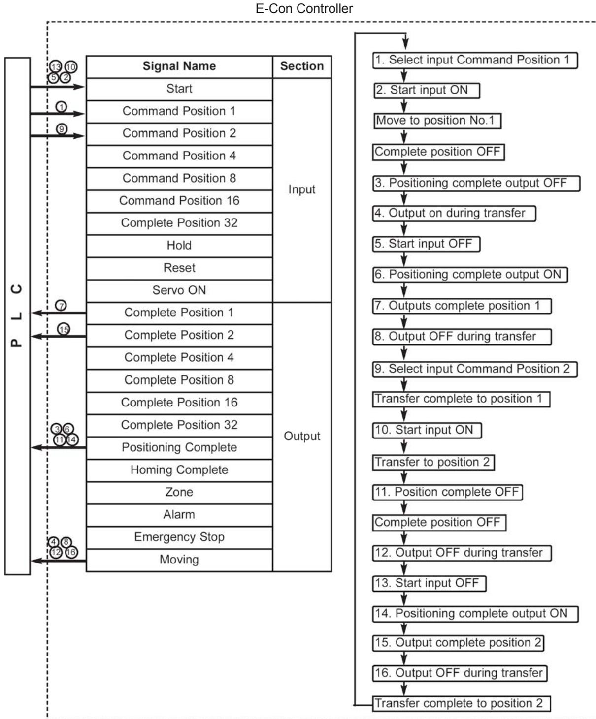
Position Data Table (Columns with the thick lines indicate the input insert)
