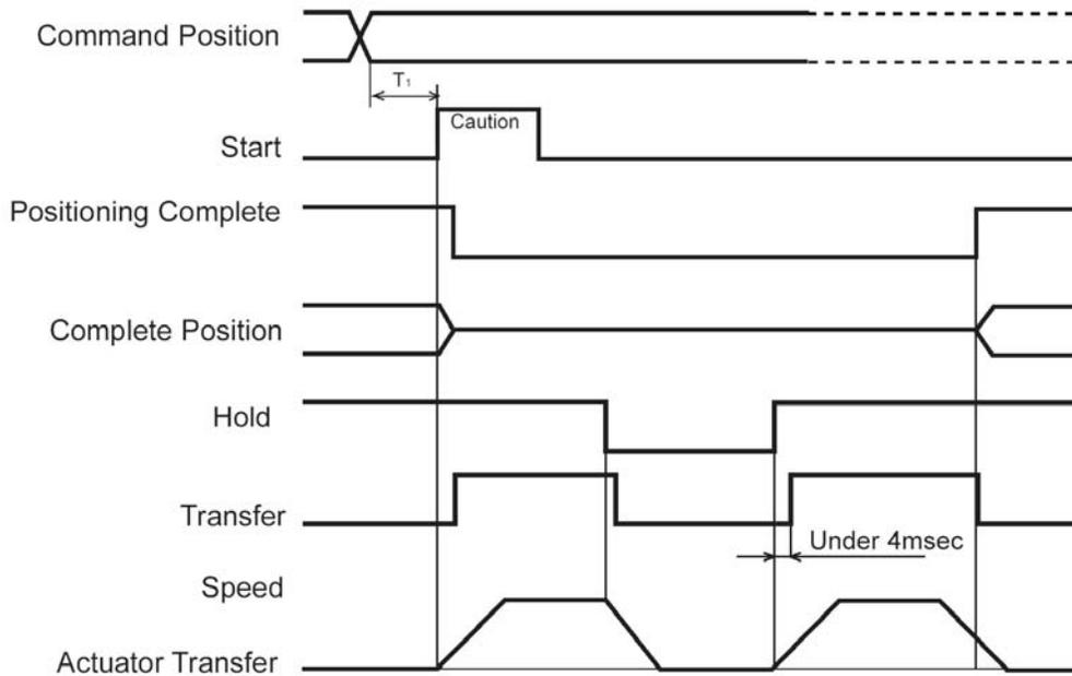
T1: Over 6 msec Time from Command Position Select Input to Start Signal ON
