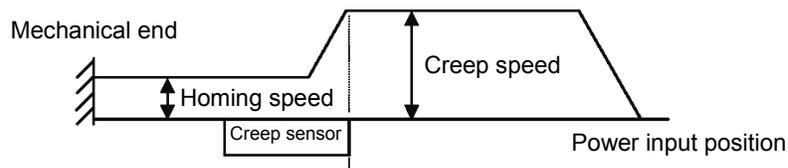
The actuator starts decelerating upon detection of a creep sensor.
