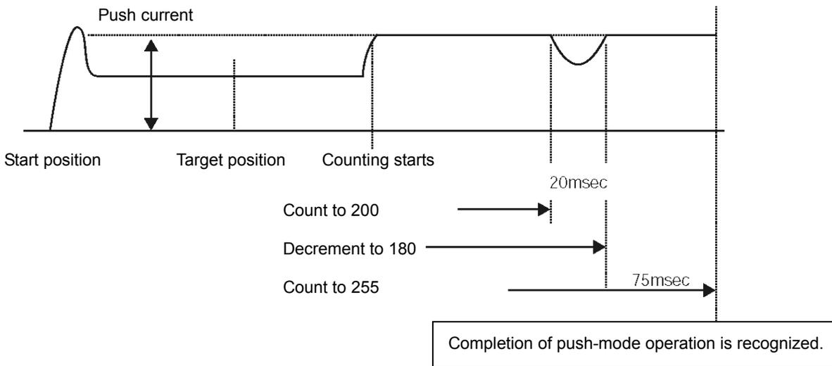
If the push current is maintained for 200 msec and then drops for 20 msec thereafter, the counter is decremented by 20. Upon recovery of the push current, counting resumes from 180. If the push current is maintained for 75 msec, the counter will have counted up to 255 and thus the controller will recognize completion of push-mode operation.
