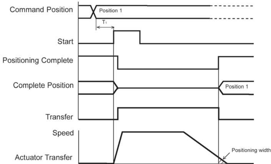
T1: Over 6 msec Time from Command position select input to start input ON.
