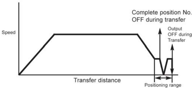
If the work moves to the push direction after the positioning complete output turns ON, the actuator will push the work within the positioning band range. The positioning complete ON and complete position number outputs will not change. In-motion output will turn OFF when motion stops.
