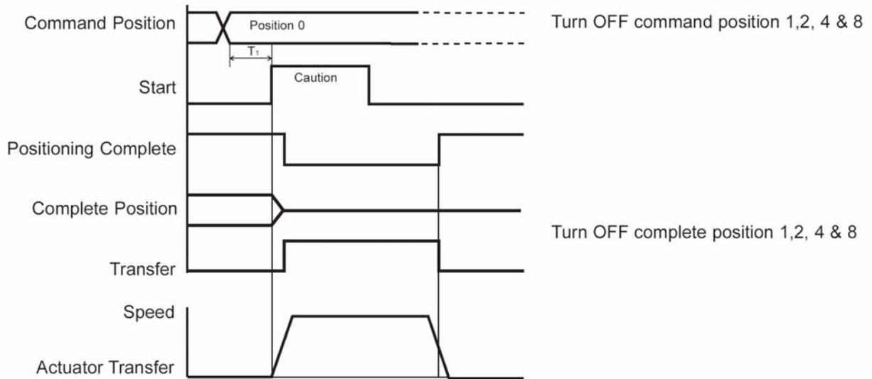
$T_1$ : Over 6 msec Time from command position select input to start input ON
