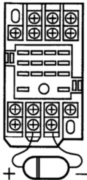
Careful attention should be paid in the case of DC current; if the polarity of the diode is mistaken, the diode, internal circuitry of the controller and/or DC power supply may be destroyed.
