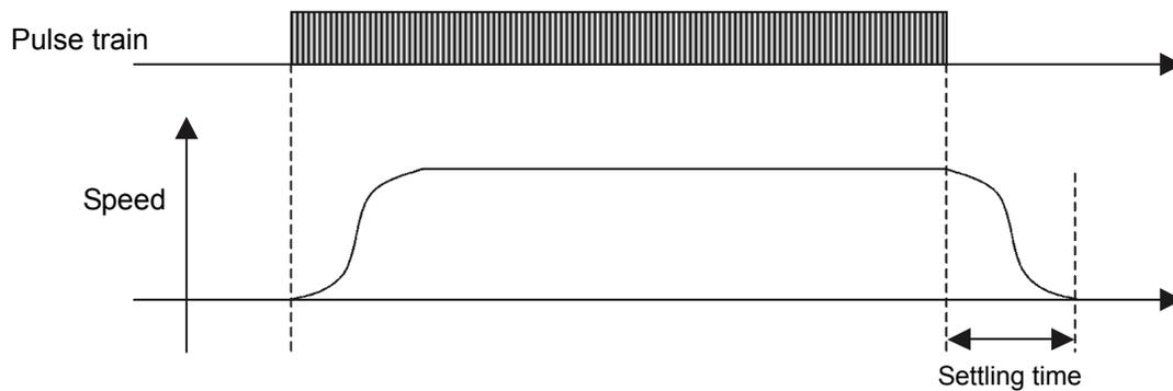
In case the host controller is not equipped with the acceleration/deceleration function or the frequency of pulse train changes sharply, if the command value is input as is, the speed command changes sharply, which may cause alarms such as “position deviation error” (alarm code: C6B) and “overload” (alarm code: D0A).
