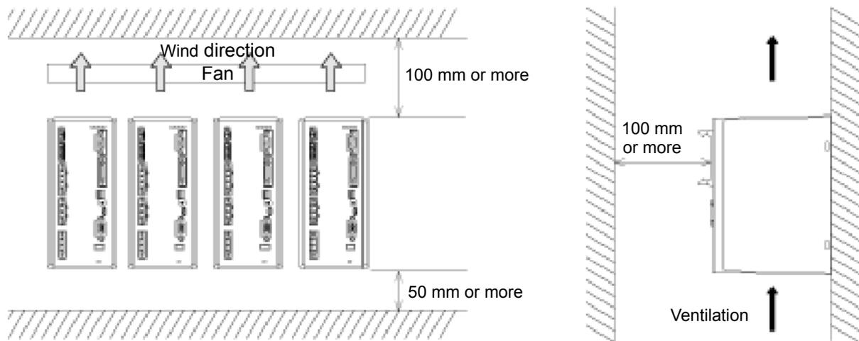
Ensure a clearance between controllers that allows easy installation and removal of individual controllers, regardless of the number of controllers.
