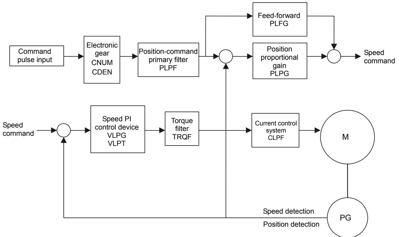
[Control Block Diagram and Parameters (Symbols) of P-Driver]
