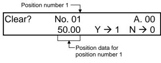
Using the Keys, change the position number into 2. Pressing 1 on the Numeric Key will clear position number 1 and then, the screen will return to the Edit/Teach Screen. To cancel, press 0. In either case, the screen will return to the previous screen.
