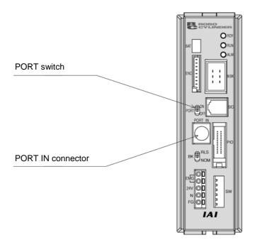
(2) After connecting, turn the controller PORT Switch ON.
