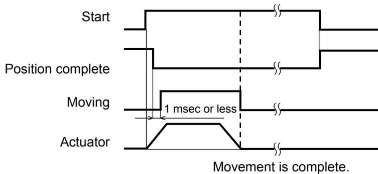
Note 2: When a soft limit is reached as a result of repeated incremental moves, the actuator will stop at that position and the position complete signal will be output.
