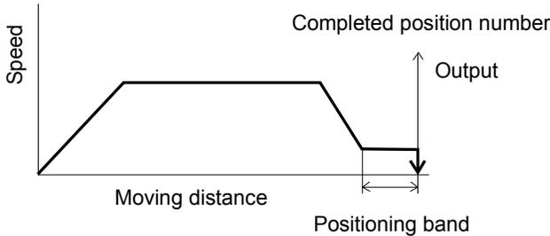
(1) After reaching the target position, the actuator will move at low speed. Even after contacting the load, the actuator will move to the end of the positioning band if the stepper motor current is yet to reach the current-limiting value. The position complete output will not turn ON even when the end of the positioning band is reached. In this case, only the completed position number will be output. (Provide a timeout check process after a sufficient period with a PLC.)
