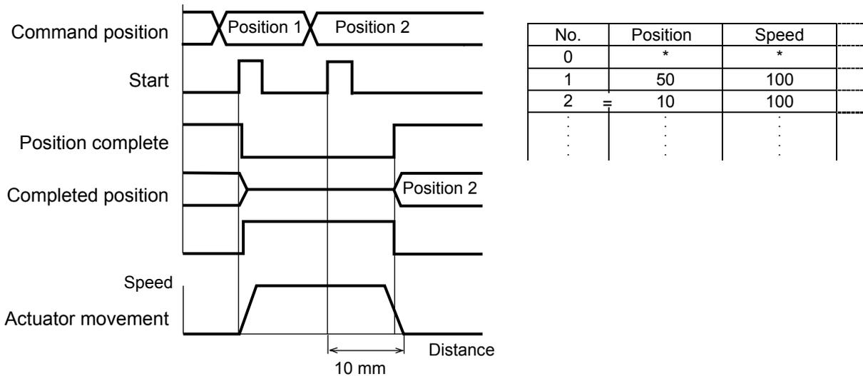
(3) Cumulative errors due to repeated incremental moves
