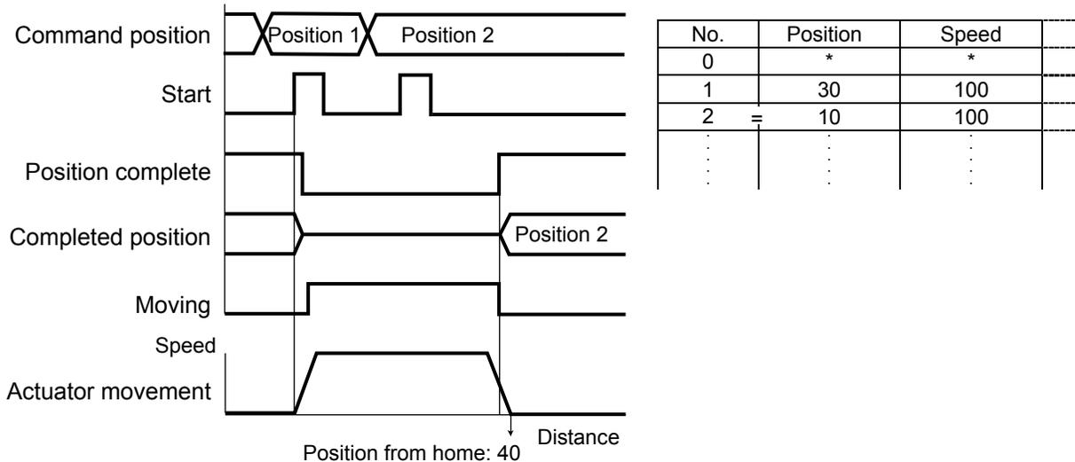
If the start signal for movement to an incremental position number is input multiple times during positioning, the actuator will move to the position corresponding to the initial position plus the “increment x number of times the signal was input.”
