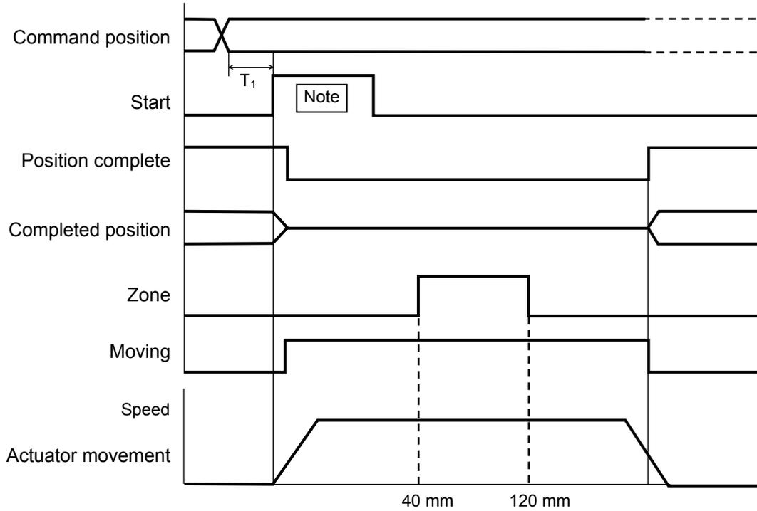
T1: 6 msec or more; time after selecting/entering a command position until the start input turns ON (The scan time of the host controller must be considered.)
