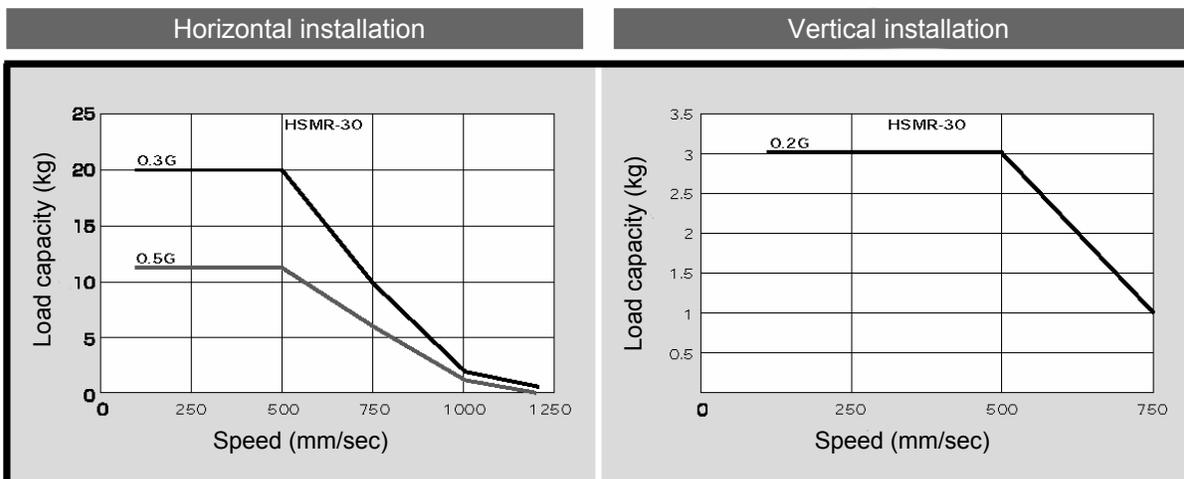
(Note) The load capacity varies depending on the acceleration.
