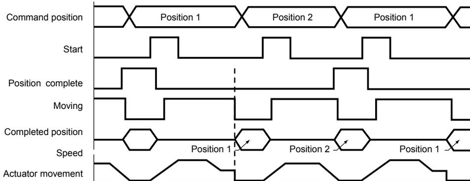
If the actuator has missed the load, the position complete output will not turn ON.
