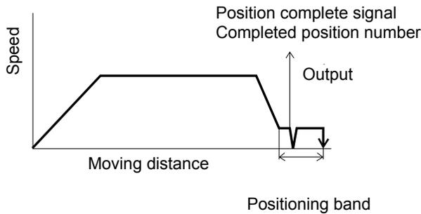
If the load moves in the pushed direction after the position complete output has turned ON, the actuator will push the load within the positioning band. If the current drops below the limiting value, the position complete signal will turn OFF. The signal will turn ON when the current rises to or above the limiting value.
