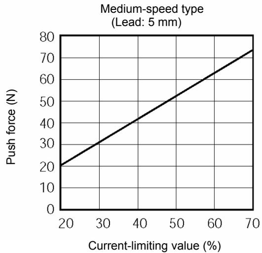
Note: The accuracy of push force at standstill is not guaranteed. The above graphs are provided for reference purposes only. If the push force is too small, malfunction may occur during push & hold operation due to slide resistance, etc., so exercise caution.
