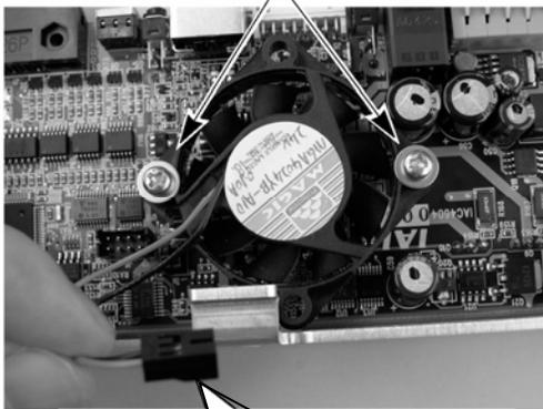
Pull out the connector by hand.
