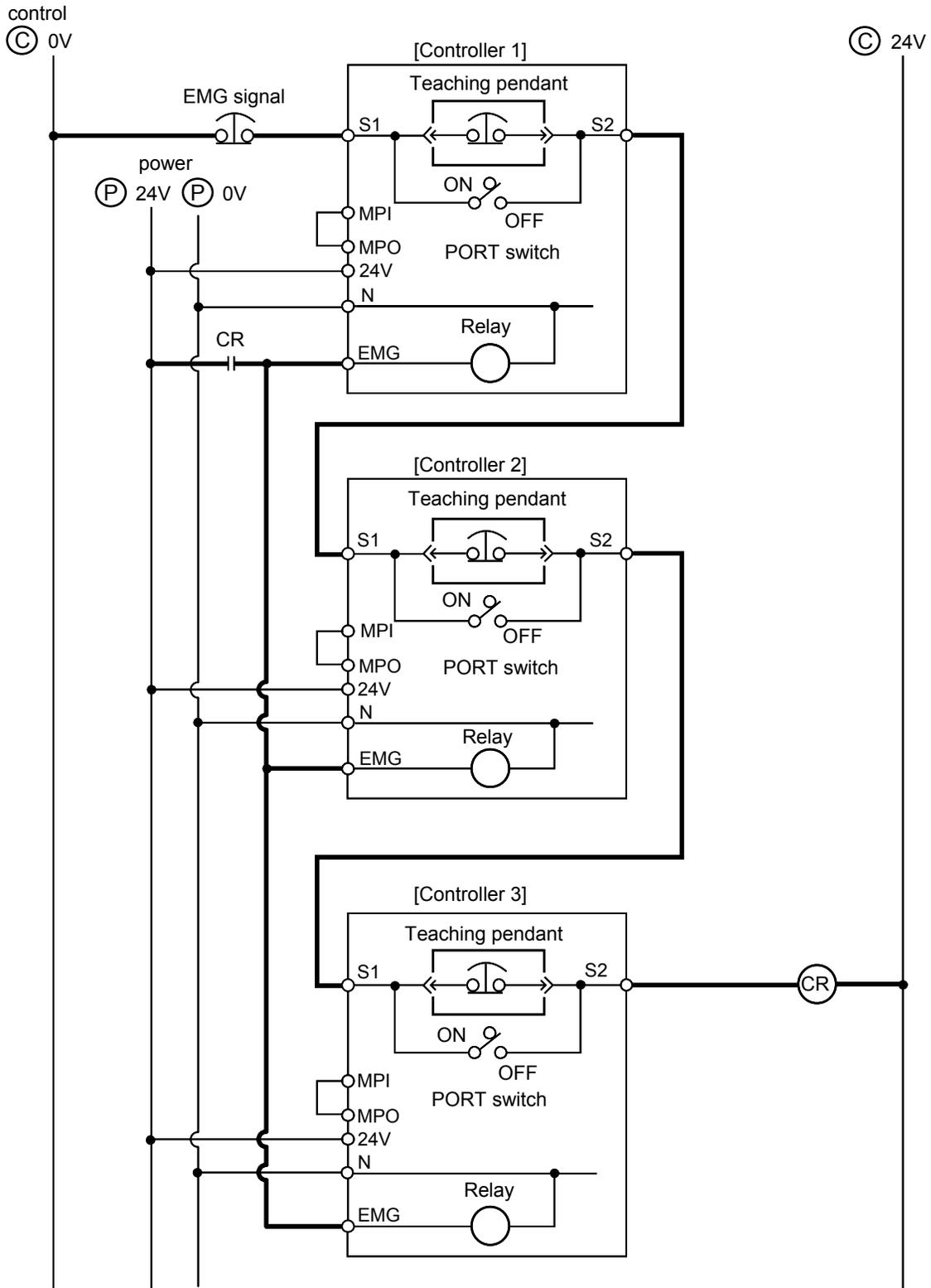
[3] Enabling the EMG switch on the teaching pendant for the connected axis or axes only
