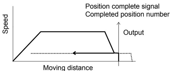
If the actuator is pushed back after the position complete output has turned ON because the actuator thrust is smaller than the reactive force of the load, the actuator will be pushed back all the way until its thrust balances out with the reactive force of the load. The position complete output will remain ON and the completed position number will be output continuously.
