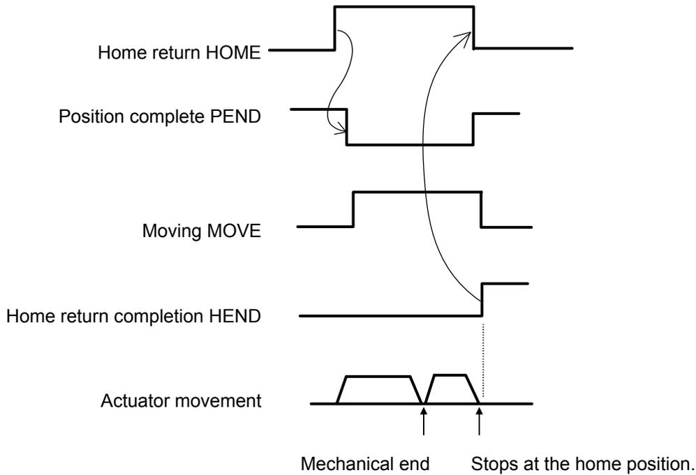
Note: When the home return signal turns ON, the position complete output will turn OFF and the moving output will turn ON. The home return signal must be turned OFF with the confirmation that the home return completion signal has turned ON while the home return signal remains ON.
