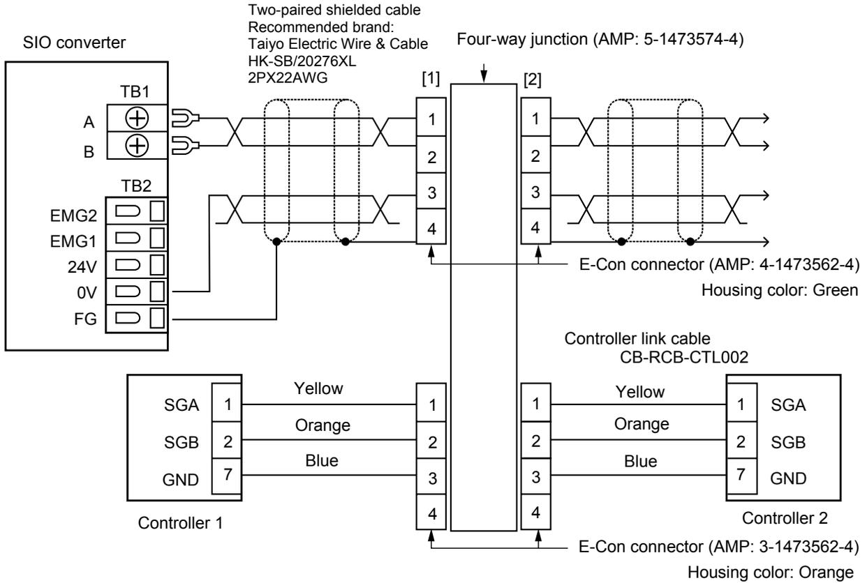
(Note) The user must provide the two-paired shielded cable.
