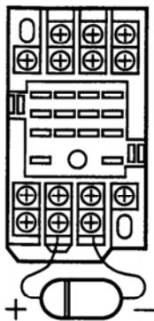
In a DC circuit, connecting a diode in reverse polarity will damage the diode, internal parts of the controller and/or DC power supply, so exercise due caution.
