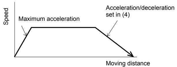
Note: Enable the acceleration only MAX setting when the actual payload is no more than one-third the rated load capacity.
