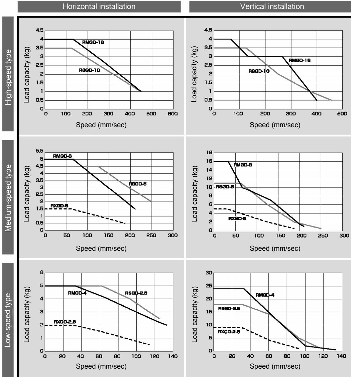
(Note) In the above graphs, the figure after each model type indicates a lead.
