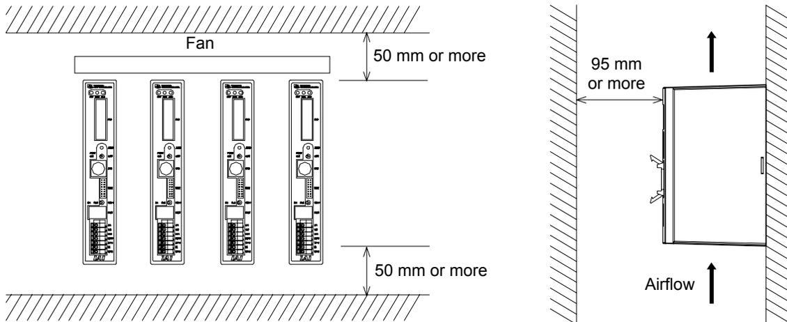
Regardless of whether your system consists of a single controller or multiple controllers, provide sufficient clearances around each controller so that it can be installed/removed easily.
