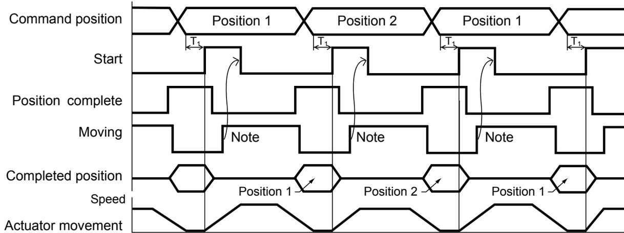
T1: 6 msec or more; time after selecting/entering a command position until the start input turns ON
