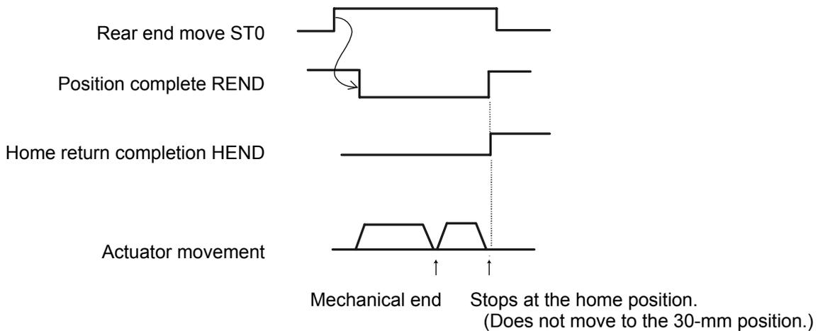
Note: With the absolute-specification controller, the actuator will not move to the target position if the set position is “other than 0.”
