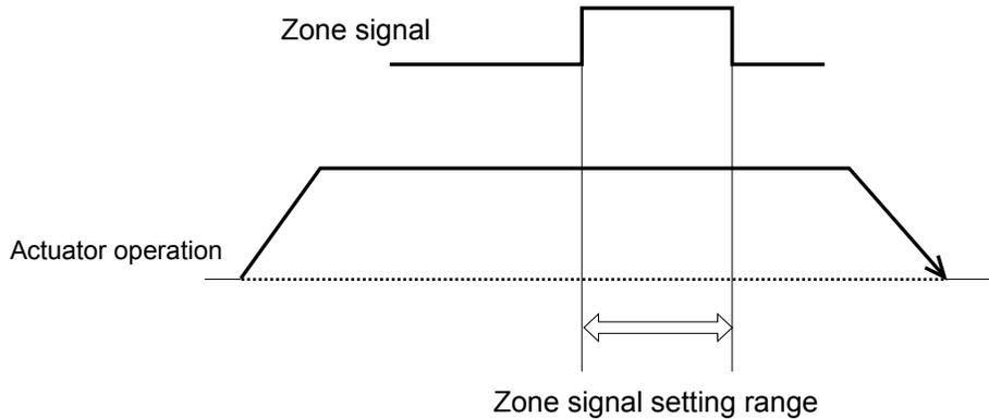
If parameter No. 25 is set to "3: [2 zone output signals]," two zone output signals can be set. The second zone value is set by parameter No. 23 (Zone 2+) and No. 24 (Zone 2-).
