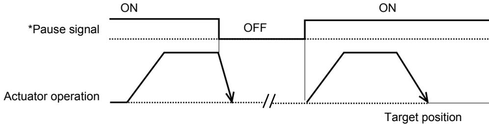
(Note) During deceleration, the acceleration/deceleration set in the position table under the currently executed position number is used.
