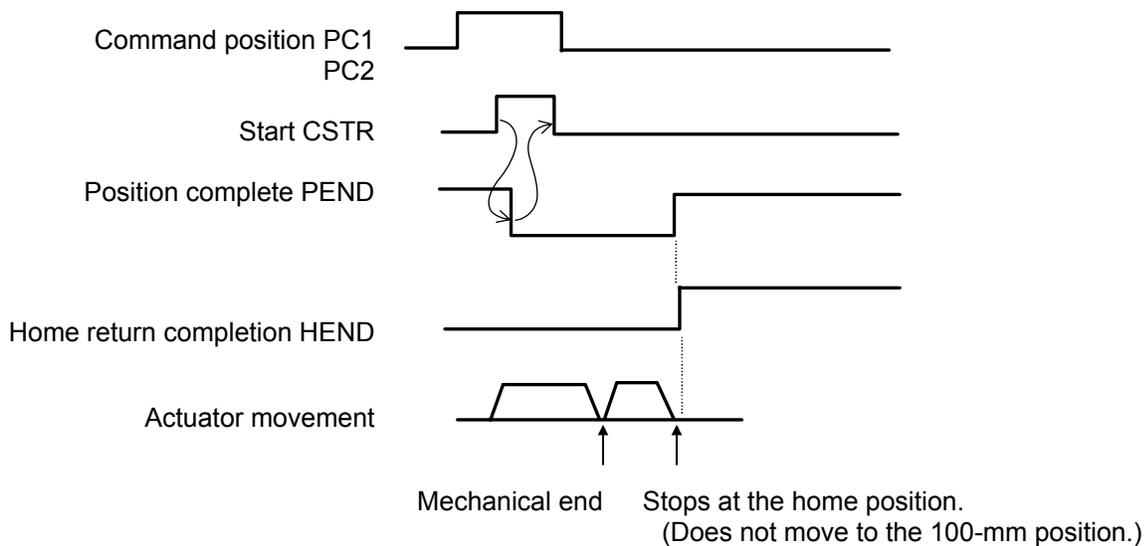
Note: With the absolute-specification controller, the actuator will not move to the target position if the set position is "other than 0."
