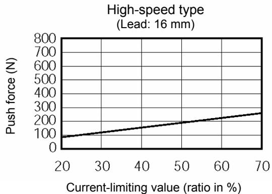
Note: The accuracy of push force at standstill is not guaranteed. The above graphs are provided for reference purposes only. If the push force is too small, malfunction may occur during push & hold operation due to slide resistance, etc., so exercise caution.
