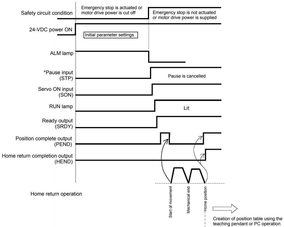
Note: If parameter No. 25 (PIO pattern) is set to “0: [Conventional],” “2: [64-point positioning]” or “5: [4 points],” the servo ON input and ready output are not provided.
