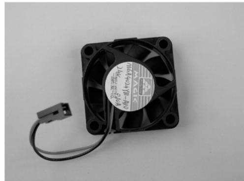
[2] Affix the new fan using the pan-head screws, and then plug in the connector.
