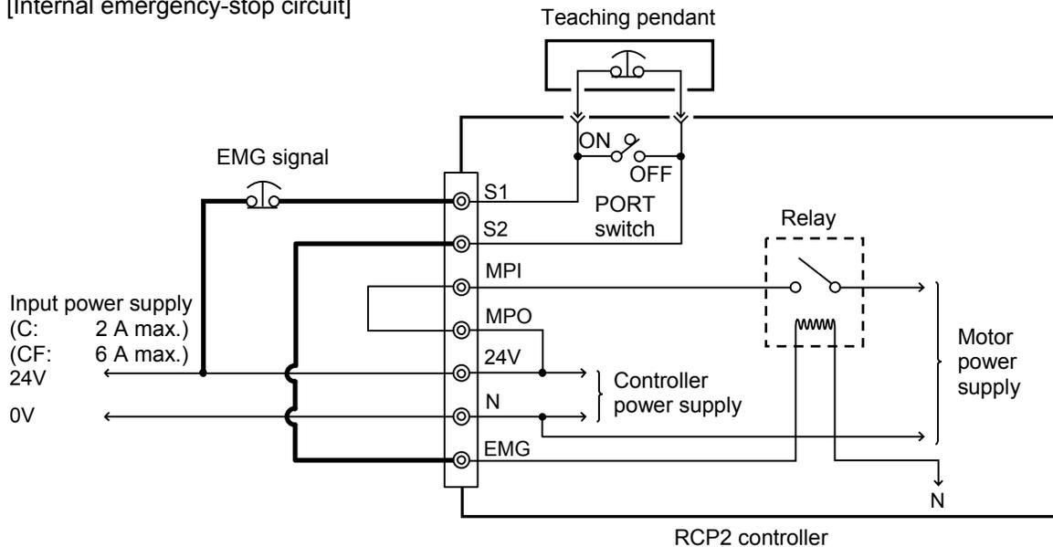
(Note) The current consumption of the internal relay is 10 mA or less.
