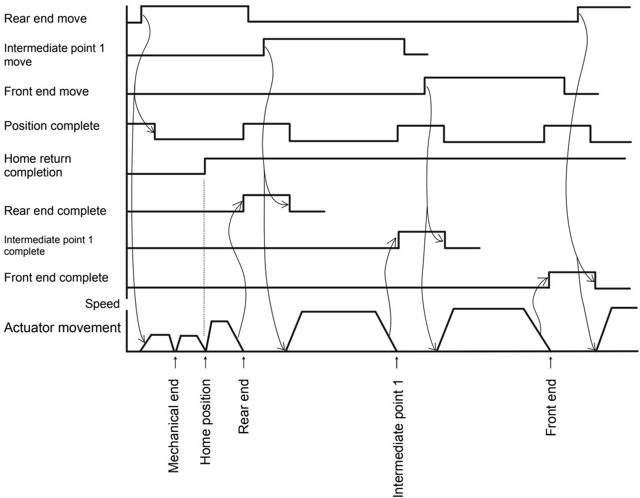
Note: Movement commands are executed based on the rise edge, so input each signal continuously for 6 msec or more.
