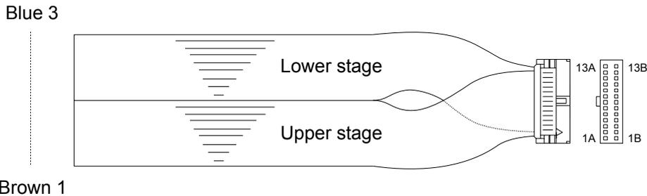
Note: When performing a continuity check of the flat cable, pay due attention not to expand the female pins in the connector. It may cause contact failure and disable normal operation of the controller.
