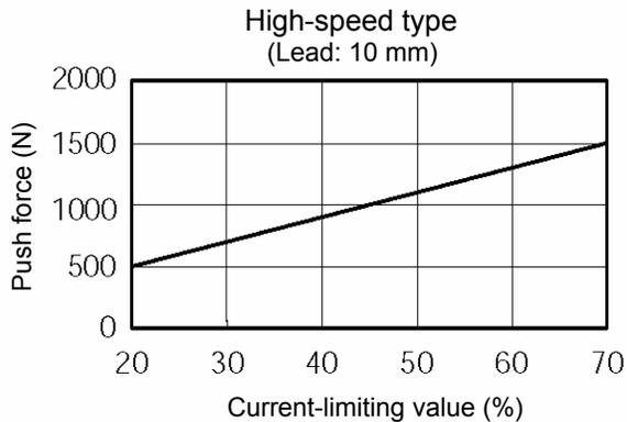
Note: The accuracy of push force at standstill is not guaranteed. The above graphs are provided for reference purposes only. If the push force is too small, malfunction may occur during push & hold operation due to slide resistance, etc., so exercise caution.
