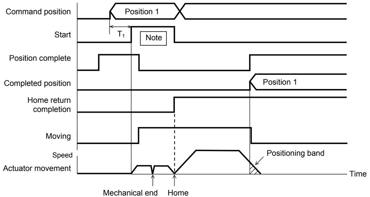
The position complete output will turn ON when the controller becomes ready following the power ON. (The position complete output will not turn ON if the servo ON input is OFF.)
