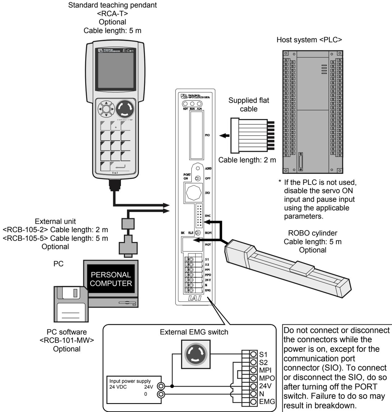
**Note:** Connect one end of the EMG switch to the 24-V output of the input power supply and the other end to the S1 terminal. Also short the S2 and EMG terminals using a jumper wire.
