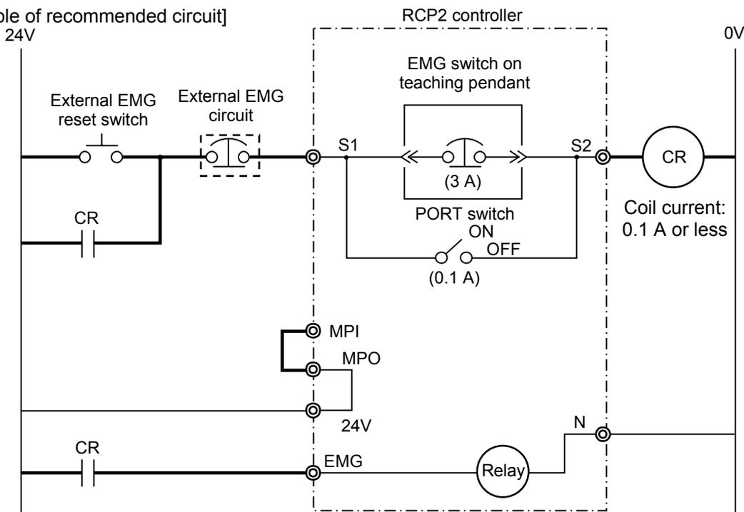
(Note) To cut off the motor drive power supply in conformance with safety category 2, connect 24V to the EMG terminal and a contactor or other contact device to the MPI/MPO terminals. (Refer to 4.2.3; rush current: 8 A.)
