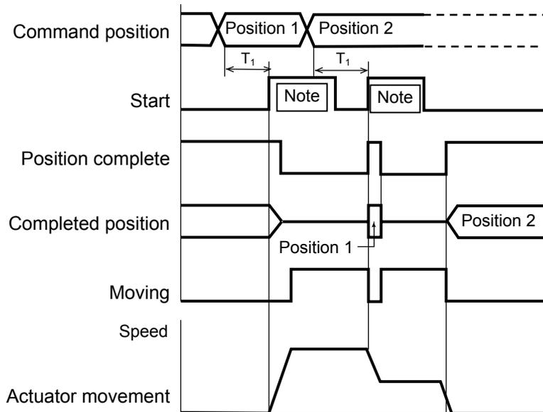
T1: 6 msec or more; time after selecting/entering a command position until the start input turns ON (The scan time of the host controller must be considered.)
