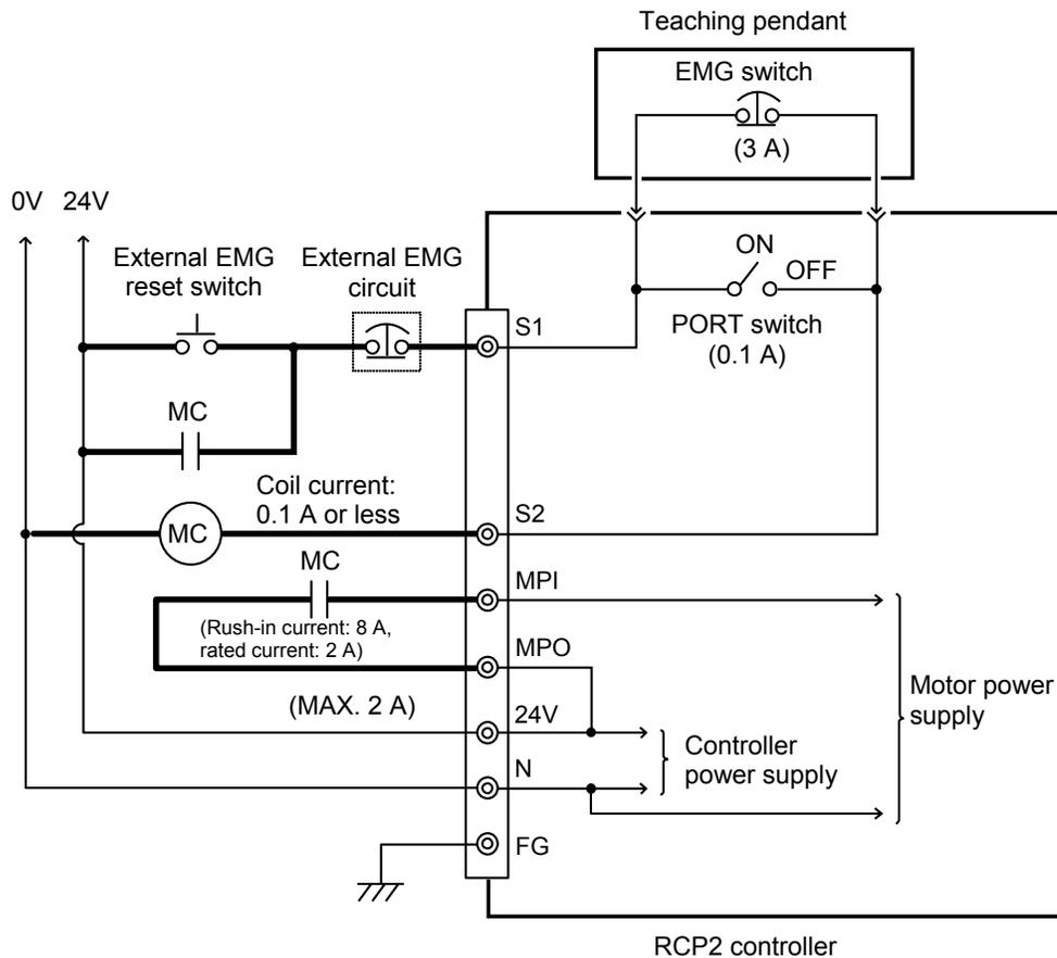
[Connection example of a multiple-axis configuration]
