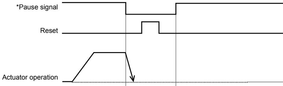
Note) If parameter No. 25 (IO pattern) is set to "0: [Conventional]," the reset input is not available.
