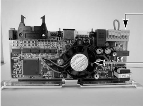
[1] Connect the power cable to the 24V and N terminals on the power terminal block.
