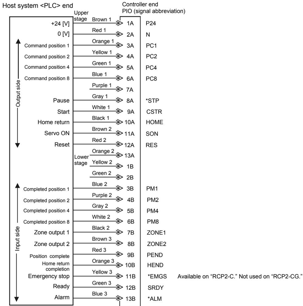
(Note) \*STP, \*ALM and \*EMGS are based on the negative logic.
