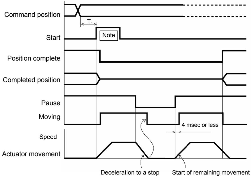
T1: 6 msec or more; time after selecting/entering a command position until the start input turns ON (The scan time of the host controller must be considered.)
