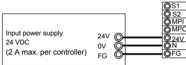
To connect multiple controllers, provide a relay terminal block.
