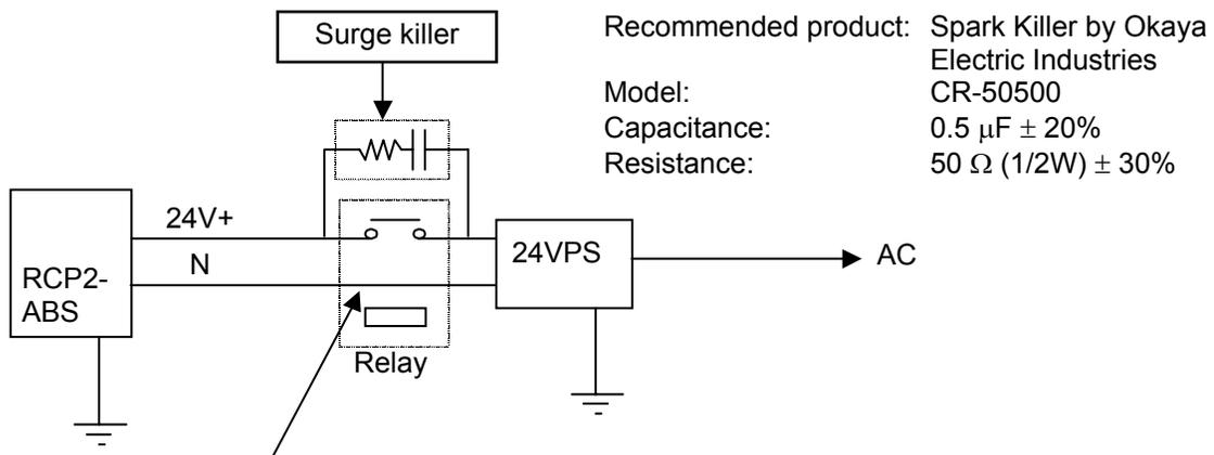
Do not install a relay on the negative side.
