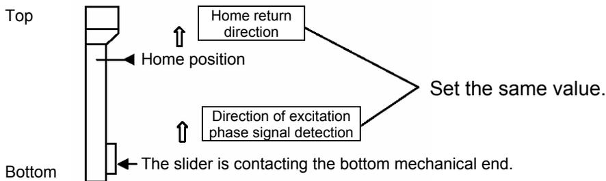
(Example 2) The power is turned on when the vertically positioned slider is contacting the bottom mechanical end, with the motor installed at bottom.
