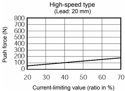
Note: The accuracy of push force at standstill is not guaranteed. The above graphs are provided for reference purposes only. If the push force is too small, malfunction may occur during push & hold operation due to slide resistance, etc., so exercise caution.
