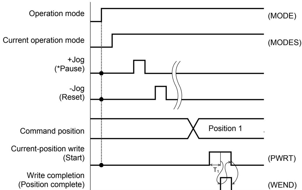
T1: 20 msec or more; time after the current-position write input is turned ON until writing of the current position is started
