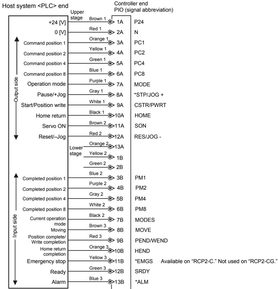
(Note) \*STP, \*ALM and \*EMGS are based on the negative logic.
