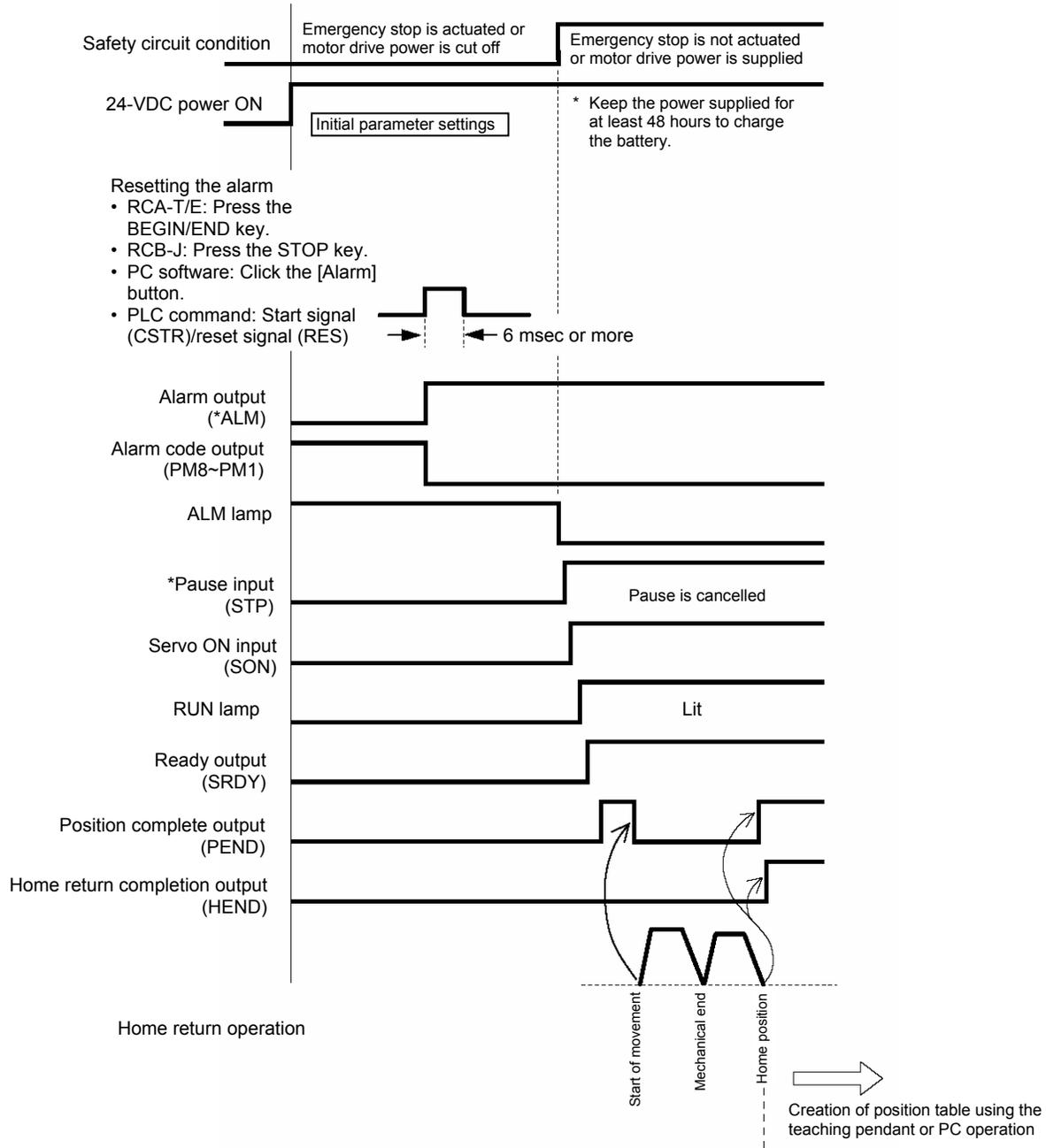
**Note:** If parameter No. 25 (PIO pattern) is set to "0: [Conventional]," "2: [64-point positioning]" or "5: [4 points]," the servo ON input and ready output are not provided.
