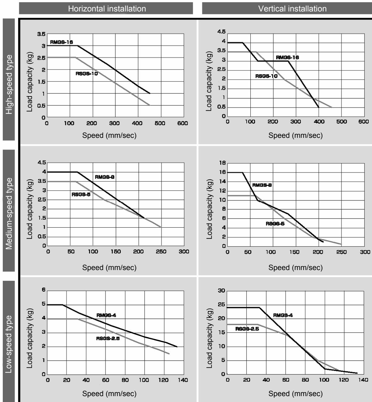
(Note) In the above graphs, the figure after each model type indicates a lead.
