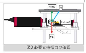
$$F_1 = mg \frac{\sin \theta}{\cos \theta} = mg \tan \theta = 6kg \times 9.8 \text{m/s}^2 \times \tan(30^\circ) = 33.9 \text{N}$$
